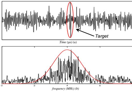
Figure #2: Scan obtained in a dispersive material with a defect at 16 μs using a 4MHz transducer with 2MHz bandwidth. (a) time (b) frequency
