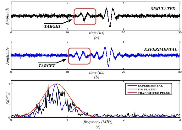
Figure #1: Simulated signal (a), experimental signal (b) and spectrum (c).
