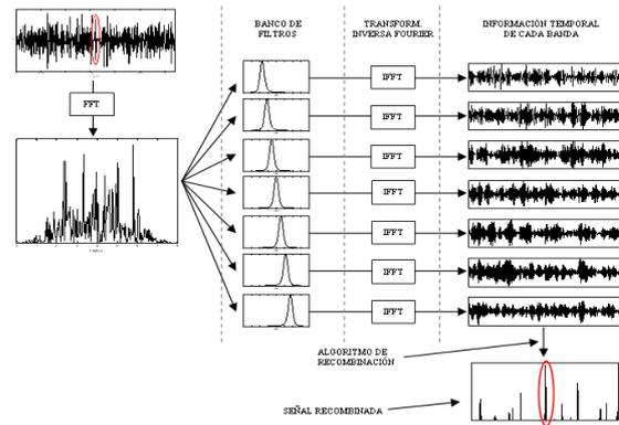
Figure #4 SSP algorithm schema
