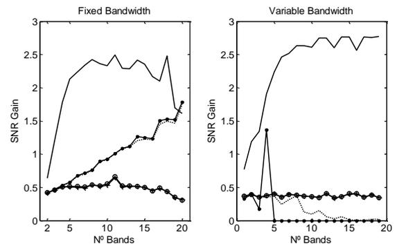
Figure #8: SNR gain Vs. number of bands of the scan using fixed bandwidth filters (left) and variable bandwidth filters (right)
