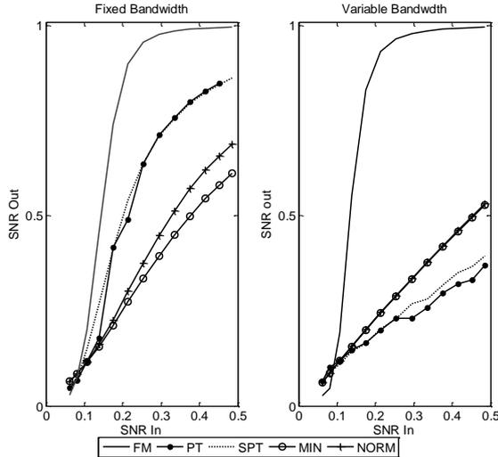
Figure #6: SNRout Vs. SNRin using fixed bandwidth filters (left) and variable bandwidth filters (right)
