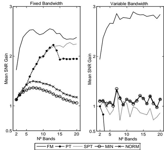
Figure #7: Mean SNR Gain Vs. number of bands using fixed bandwidth filters (left) and variable bandwidth filters (right)
