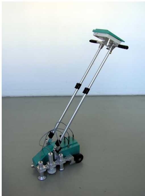
Abb. 3 Mikrowellenscanner MOIST SCAN
