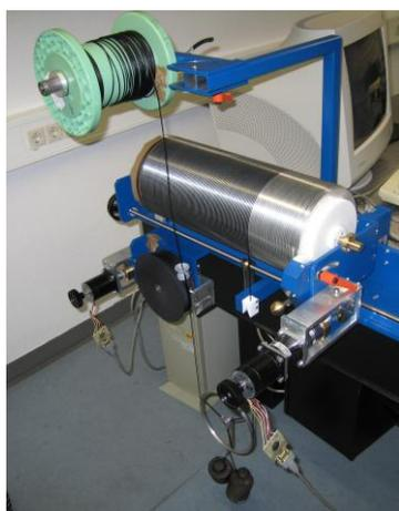
Figure 14: Specially developed test facility to apply distributed strain along an long optical fibre (Photo: BAM)
