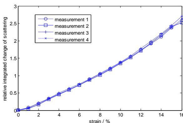
Figure 15: Strain measurements (4 test series) at different locations along the POF [5]
