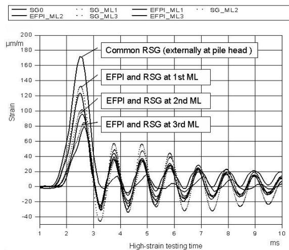
Figure 4: Measured strains during high-strain testing.
