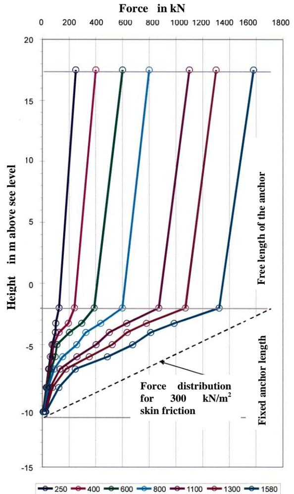
Figure 10: Load transfer of anchor A1 measured with applied strain sensors. Diagram: German Federal Waterways Engineering and Research Institute (BAW) Karlsruhe
