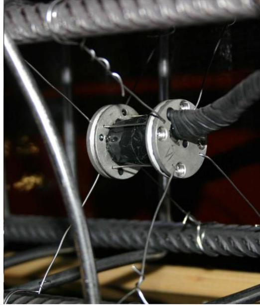
Figure 2: Sensor body fixed at the reinforcement steel
