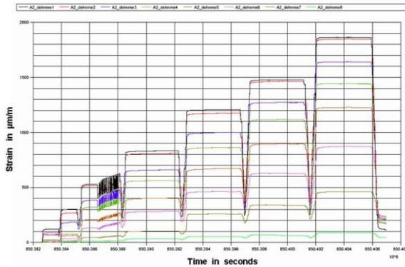
Figure 9: Original strain distribution data from FBG sensors during stepwise loading of anchor A2. Diagram: BAM
