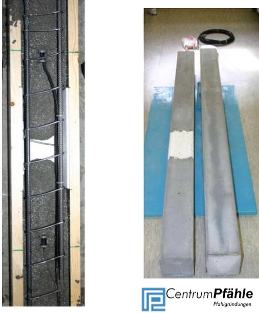
Figure 1: Casting of sensor-equipped model piles. Sensors are fixed at the cage of reinforcement (left); one pile has got an imperfection (left pile in the right picture)
