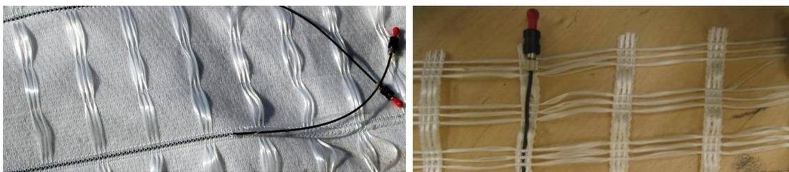
Figure 13: Geotextiles with integrated POF sensors (Photo and textile: STFI e. V. Chemnitz)
