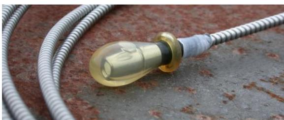
Figure 17: Water filled topcoat for the pH sensitive membrane to prevent dehydration. Photo: STUMP GmbH
