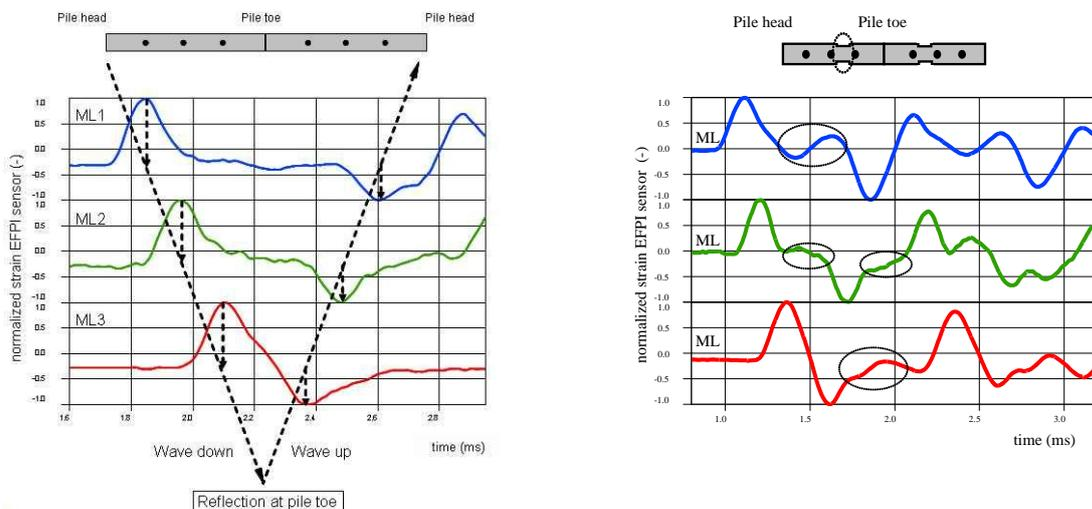
Figure 3: Strain responses of EFPI sensors over time from one pile without imperfection (left) and one with imperfection (right) during low-strain integrity testing; impact was generated by steel ball with a diameter of 40 mm (falling height: 60 cm).
