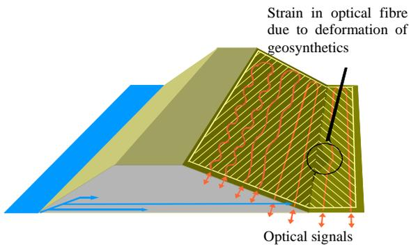
Figure 11: River dyke with sensor-based geosynthetics
