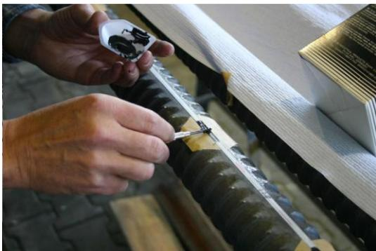
Figure 6: Application of FBG sensor to the steel bar
