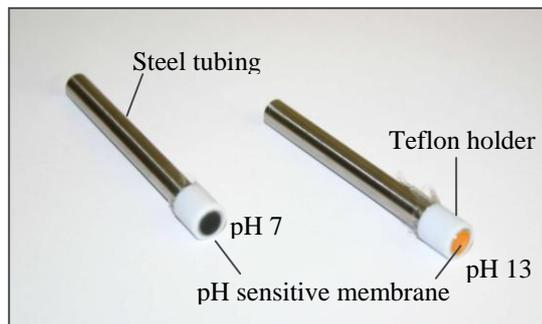
Figure 16: pH sensor head design; the head is pluggable and can be replaced. Photo: BAM
