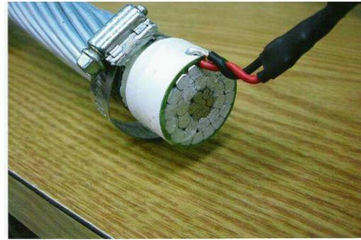
Fig. 13: Piezoelectric ring transducer attached to the transmission line.
