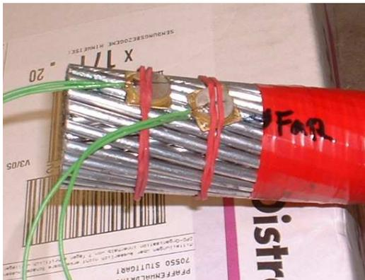
Fig. 17: Disc transducers attached to a surface wire.
