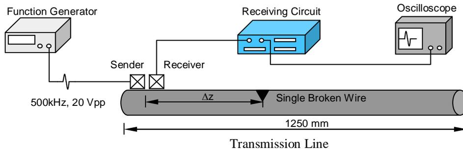
Fig. 16: Alternative experimental setup for defect detection in a transmission line.
