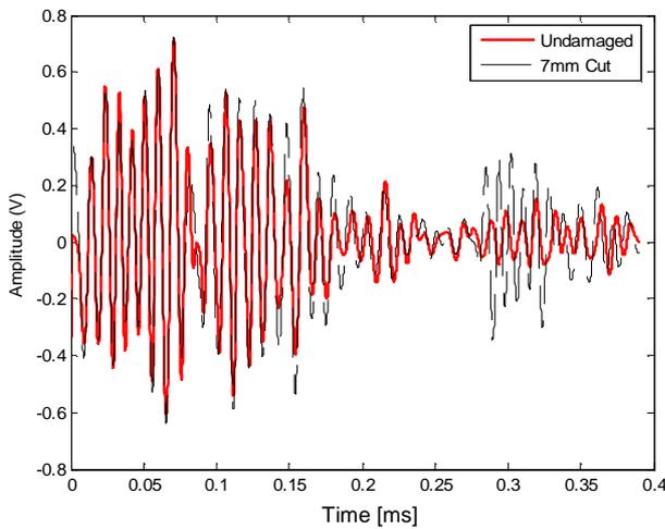
Fig. 14: Transducer output for a damaged and an undamaged transmission line.
