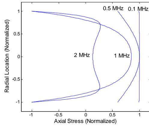
Fig. 4: Radial variation of axial stress for the 1<sup>st</sup> longitudinal rod mode.
