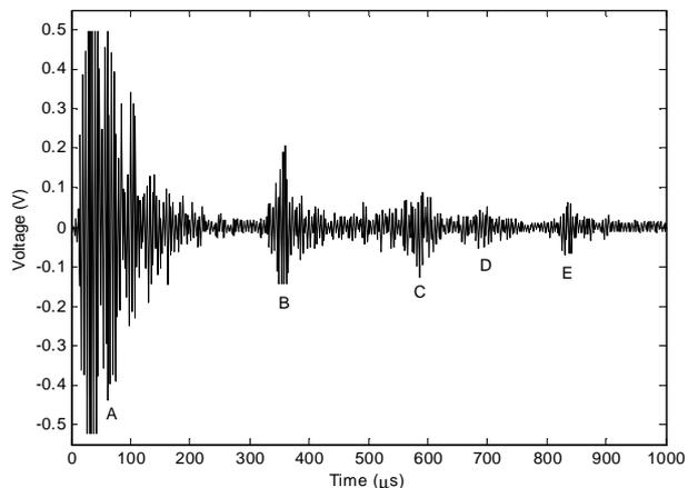
Fig. 18: Electrical output from the receiving transducer.
