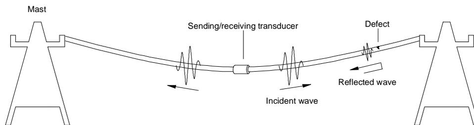
Fig. 1: Interrogation of a transmission line using ultrasonic pulses
