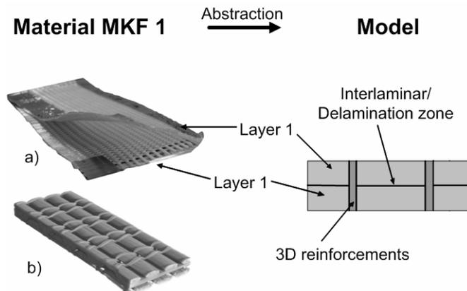
Fig. 8 (a) Material structure photo of unconsolidated knitted MKF 1, (b) CT-scan of the material and mesoscopic model [6]
