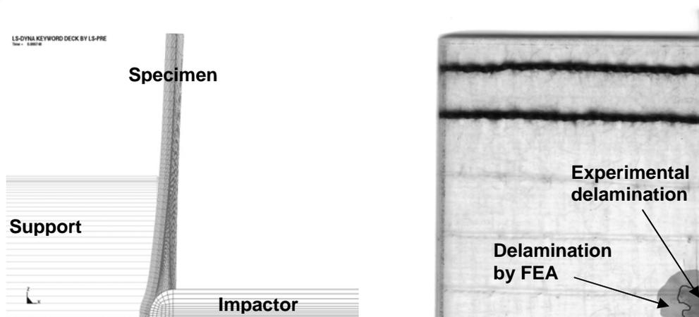
**Fig. 12** Impact simulation (left), delaminated area calculation vs. experimental result (right, quarter of specimen) [6]
