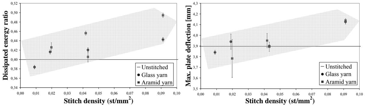
Fig. 7 Exemplary results of impact experiments at  $v_{imp}=8$  m/s based on recorded data [9]
