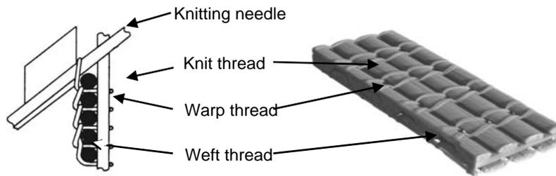
**Fig. 3** MKF type 1, left: basic architecture (schematic) [1], right: CT-scan [9]
