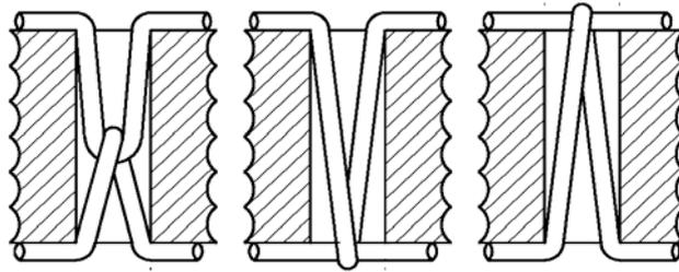
**Fig. 2** Variation of the yarn tension with the double locked stitch technology [8]
