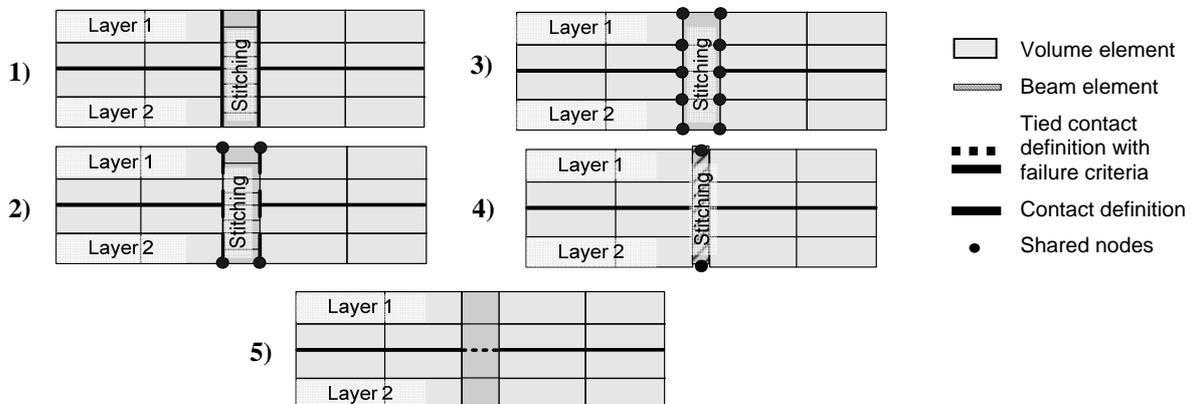
**Fig. 11** Modelling concepts for the 3D-reinforcements: 1) tied contact of volume elements, 2) contact of volume elements, 3) classification by material model, 4) beam element, 5) contact [6]
