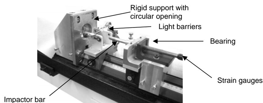
**Fig. 1** Impact-bending-test device (IBT) with rigid support (without specimen) at the Department of Engineering Science, Oxford University [6]
