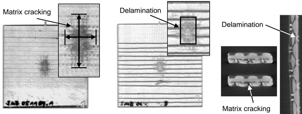
**Fig. 5** Damage events and failure modes after impact (left: glass stitching; middle: aramid stitching, right: CT-scan) [9]
