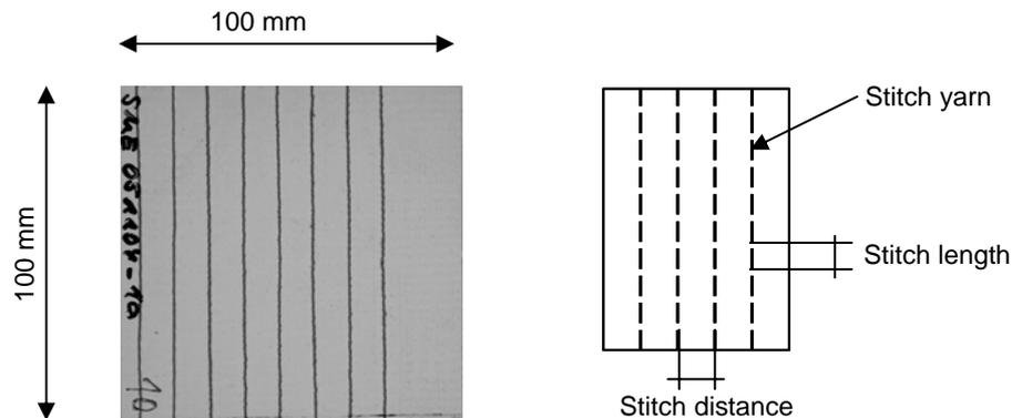
**Fig. 4** Configuration of the stitched specimens
