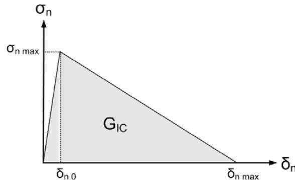
**Fig. 10** Bilinear stress-gap opening behaviour (linear post failure response) for interlaminar mode I fracture with  $\sigma_n$  and  $\delta_n$  the normal stress and the gap opening
