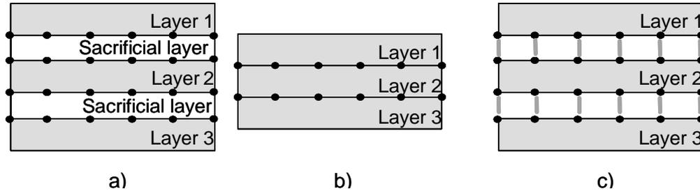
**Fig. 9** Basic approaches for delamination modelling: (a) sacrificial layer, (b) implemented in material model, (c) contact definition
