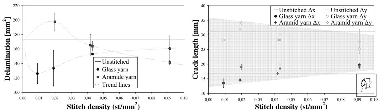
**Fig. 6** Exemplary results of impact experiments at  $v_{imp}=8$  m/s based on non-destructive inspections [9]
