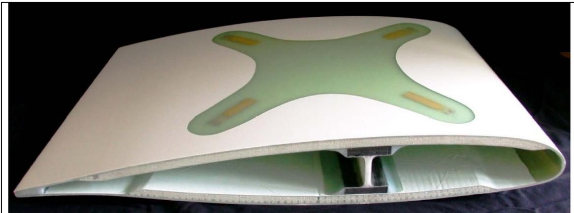
**Fig. 14:** Embedded PZT fibre transducers for Structural Health Monitoring of an aircraft wing.
