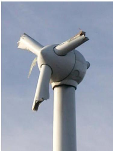
loss in stiffness. When a part of the structure is finally too weak to withstand the loads a sudden rupture of the fibres in the remaining cross section occurs. This can lead to a chain reaction destroying the whole structure, as shown in fig. 1. A rupture of a rotorblade of wind energy plants can endanger residents or other plants as far as 600 meters away.
