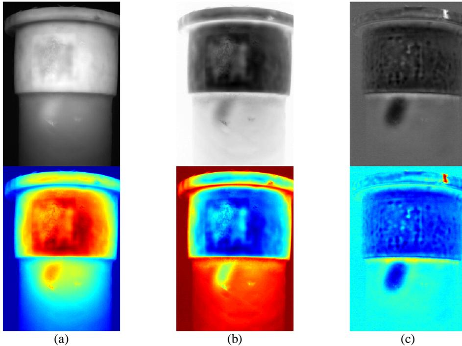
Figure 7: Defect 'A': (a) gray (top) and 'jet' (bottom) raw thermograms at  $t=0.92$  s; (b) first time derivative image (from a 7th degree polynomial fitting) at  $t=2.85$  s; (c) second derivative at  $t=1.49$  s.
