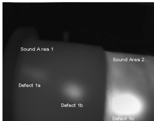
Figure 5: Thermal image of investigated pipe after 0.935 seconds of heating
