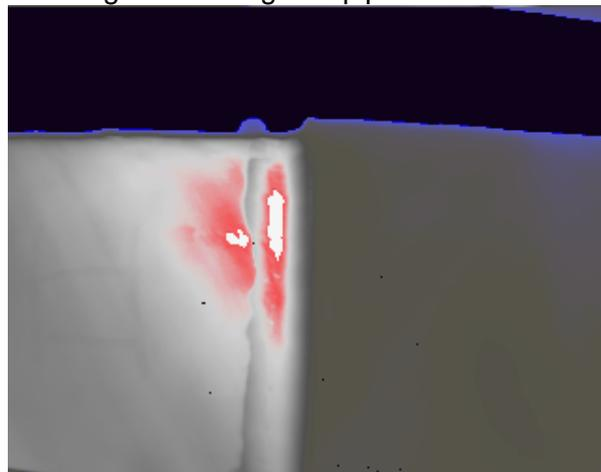
Figure 6: Thermal image of investigated pipe after 13.560 seconds of heating revealing kissing bond defect on the pipe
