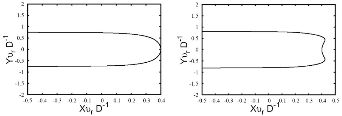
Figure 4: Crack shape obtained for  $\Delta = 1.3$  and  $\Delta = 2.3$ , using the series expansion method. The negative tip curvature can cause tip splitting.
