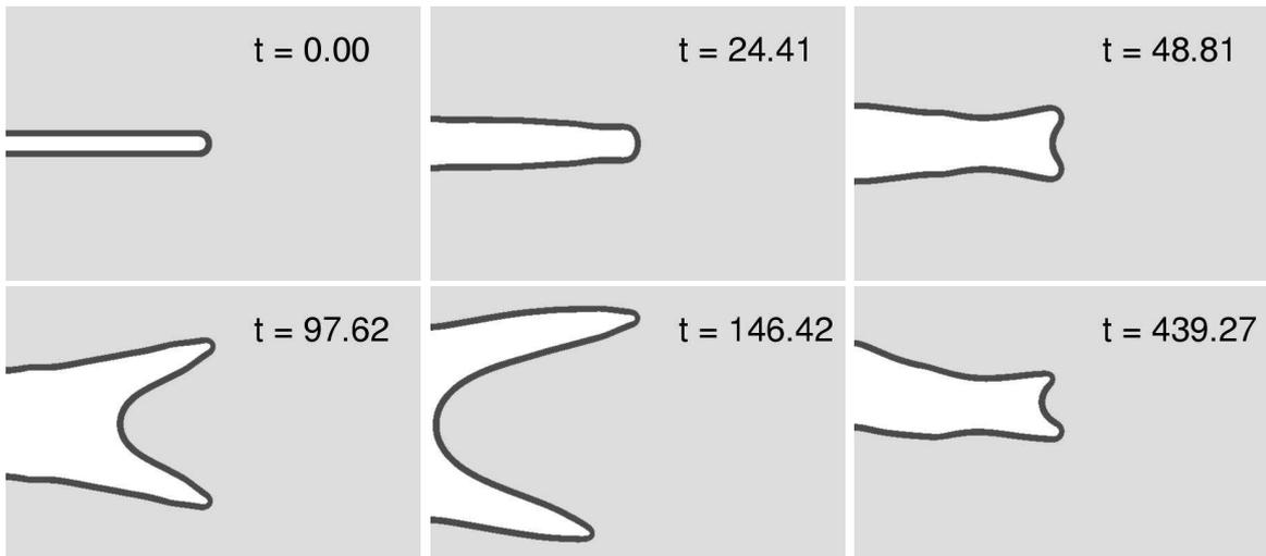
Figure 5: Irregular tip splitting scenario. We used  $D/\xi v_R = 1.85$  and  $\Delta = 3.6$ ; the system size is  $600 \times 400$ . Time is given in units  $D/v_R^2$ .
