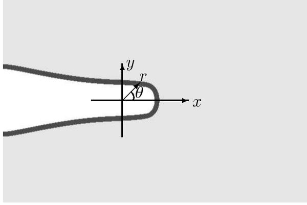
Figure 1: Steady state growth of a crack in a strip with mode I loading, as obtained from phase-field simulations.
