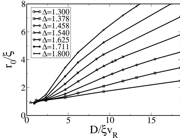
Figure 3: Tip radius  $r_0$  as a function of the kinetic coefficient, for different driving forces  $\Delta$ .
