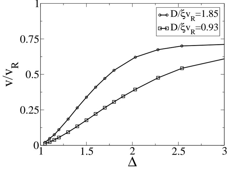
Figure 2: Steady state velocity as a function of the dimensionless driving force  $\Delta$ .
