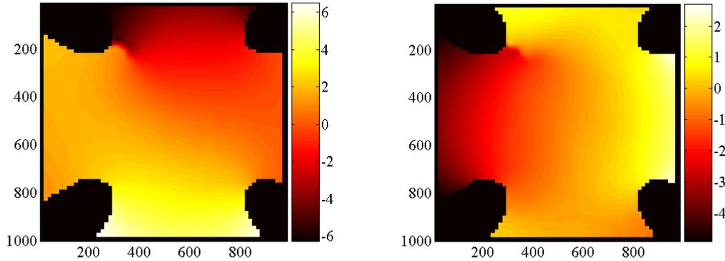
**Figure 2: Vertical (left) and horizontal (right) component of the displacement field obtained from a Q4P1 decomposition with an element size equal to 16 pixels. The physical size of one pixel is 67  $\mu\text{m}$ .**
