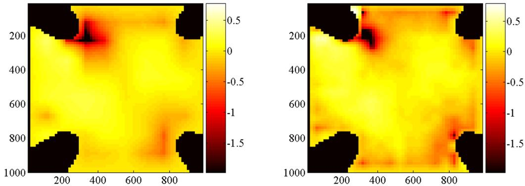
**Figure 3: Map of  $\log_{10}(1-D)$  obtained for a coarse (10 x 10) and fine (20 x 20) mesh.**
