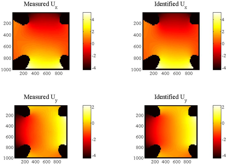
**Figure 7: Comparison between measured (left) and recomputed (right) displacement field based on the identified damage law.**
