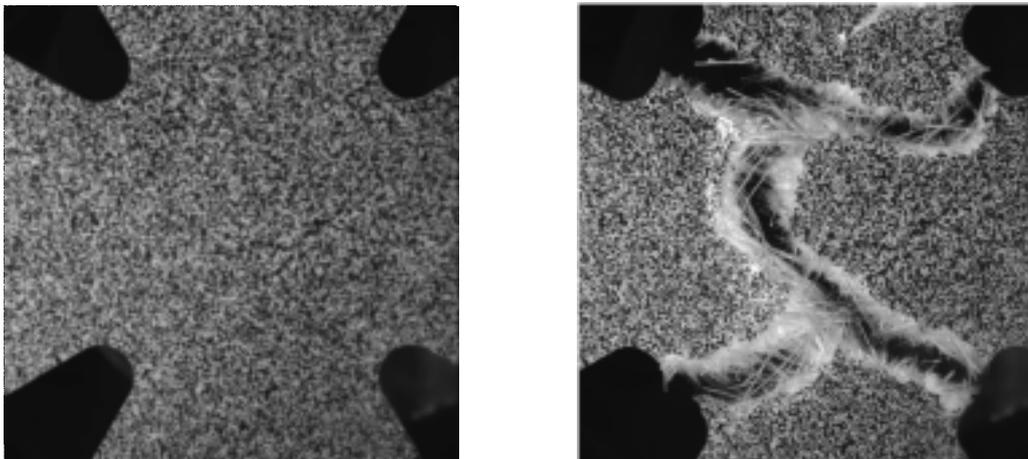
**Figure 1: Image of the sample prior to loading (left) and after failure (right)**
