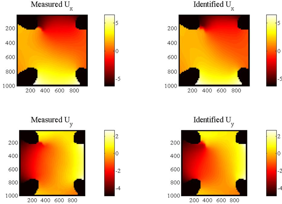
**Figure 4: Comparison between measured (left) and recomputed (right) displacements from the identified damage field (fine grid 20 x 20).**
