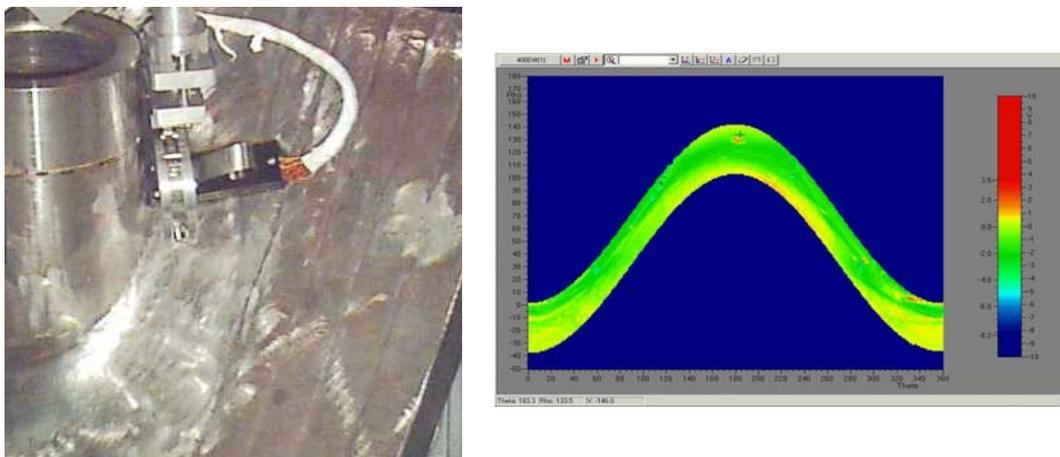
Figure 3 a) Multi-coil element J-Weld Inspection and b) C-Scan Representation data output
