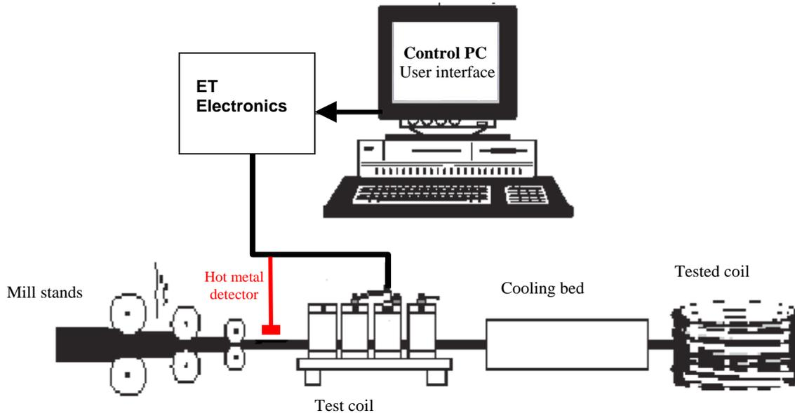
Figure 4 Components of an inspection system for hot-wire inspection
