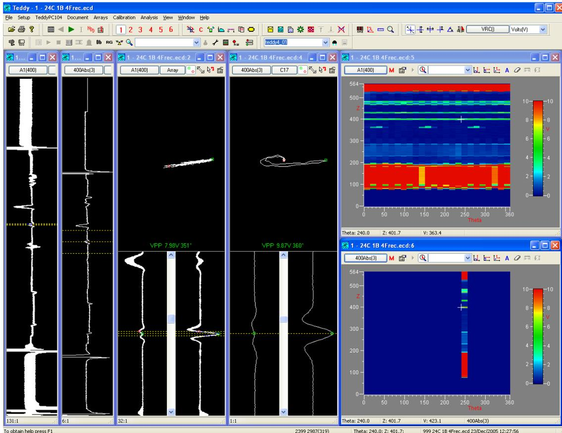
Figure 8 Strip-chart, lissajous and C-Scan representation of an array channel corresponding to the I-Probe
