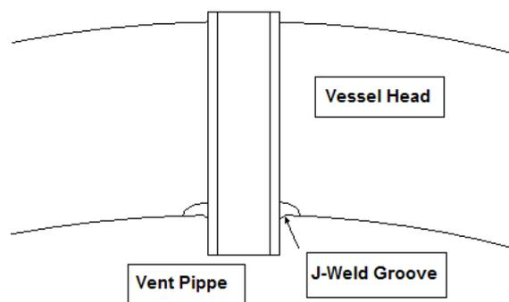
Figure 2 Sketch of the J-Weld groove to be inspected
