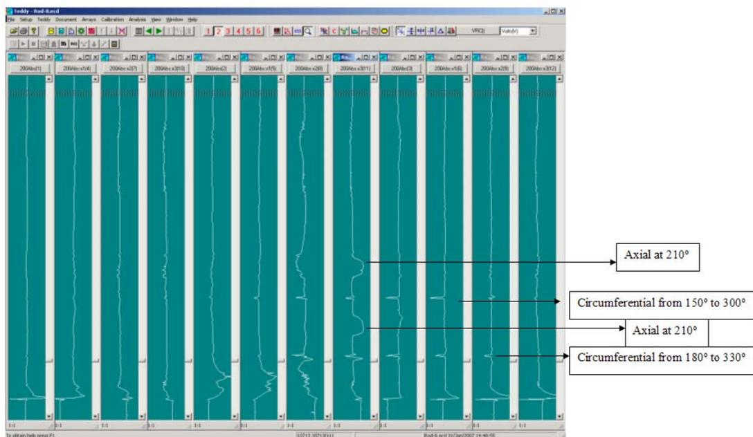
Figure 5 Results with the plus-poin array sensor and rod 8
