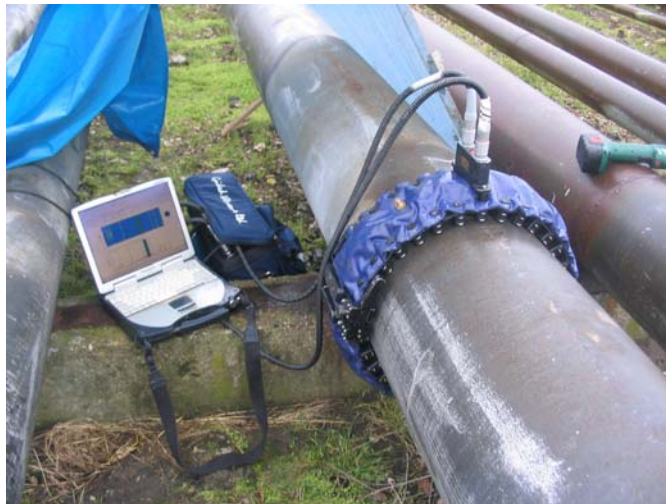
Figure 4 – Anneau souple et instrumentation d'acquisition
