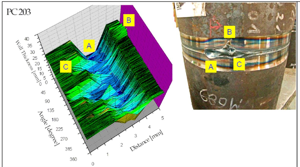
Figure 3. Typical result obtained with a sample with artificial defects.
