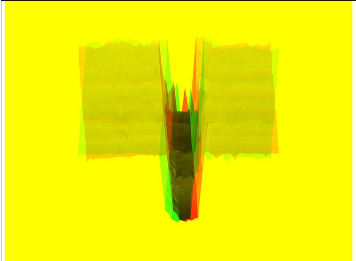
Figure 7. Stereo image of the root path of a weld seam reconstructed from phased array UT data processing. The program used for generating the stereo image is available at <http://neuronik.free.fr/Stereo/>.
