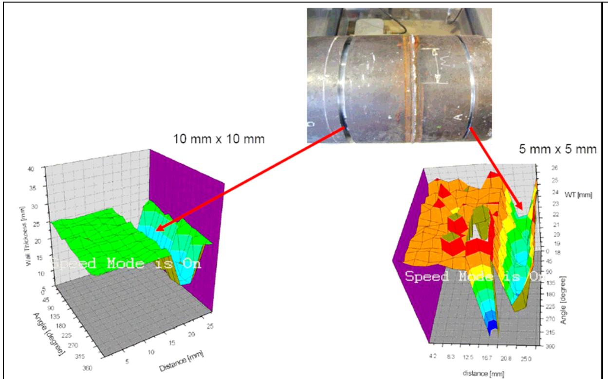
Figure 4. Topographical representation of the sections of 5x5 mm and 10x10 mm constructed for calibrating the measurements on layer thickness of the welds.
