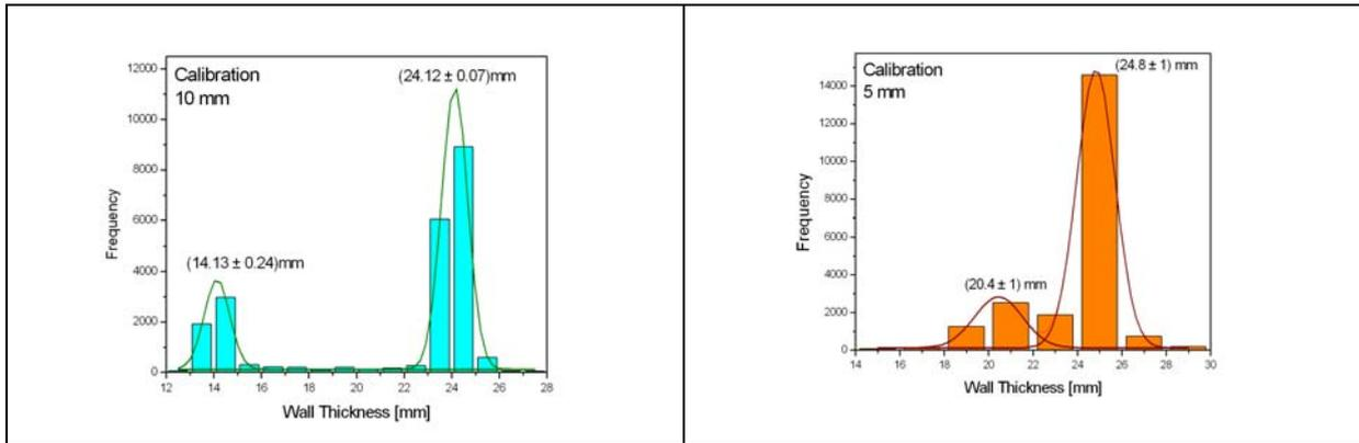
Figure 5. Wall thickness values for the sections of 5x5 mm and 10x10 mm. Mean value is based on a normal fitting. Distances between peaks refer to the WT of the annular section. Uncertainty values (given in Table 1) are given by the some of the LWHM of both gaussians.
