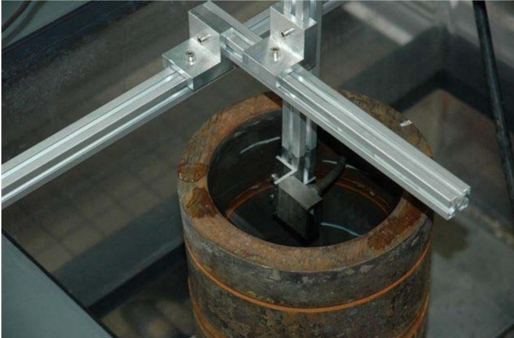
*Figure 1. Experimental setup used to record phased array UT data on weld seam. The phased array sensorhead is fixed and the pipe filled with water turns clockwise. Installing the phased array outside will produce the same effect.*
