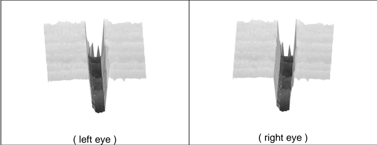
*Figure 6. Representation of left and right eye images of the root path of a weld seem.*
