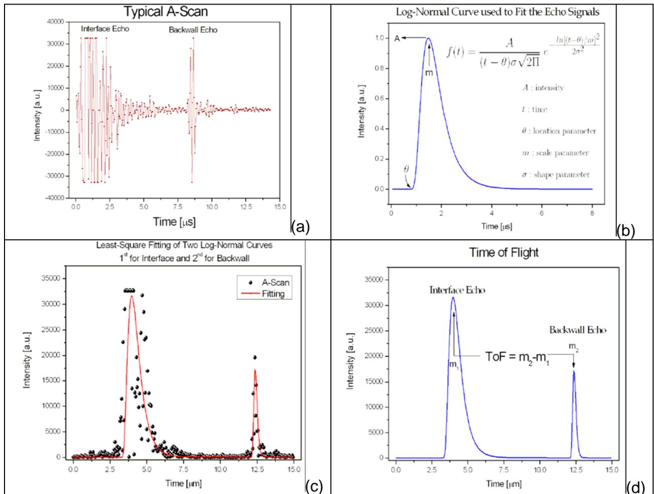
Figure 2. Topographical representation of the sections of 5x5 mm and 10x10 mm constructed for calibrating the measurements on layer thickness of the welds. (a) typical A-scan recorded for one element of the phased array; (b) log-normal curve used to least-square fit the absolute values of the A-scan; (c) typical least-square fitted A-scan and (d) ToF calculation from the peak position.
