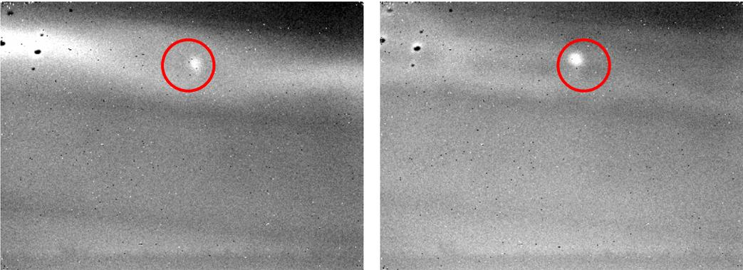
Figure 10: Infrared images of the impact damage with 1.2 s (left) and 2 s (right) excitation times (200 cm distance between excitation point and damage and 1000 W power amplitude).
