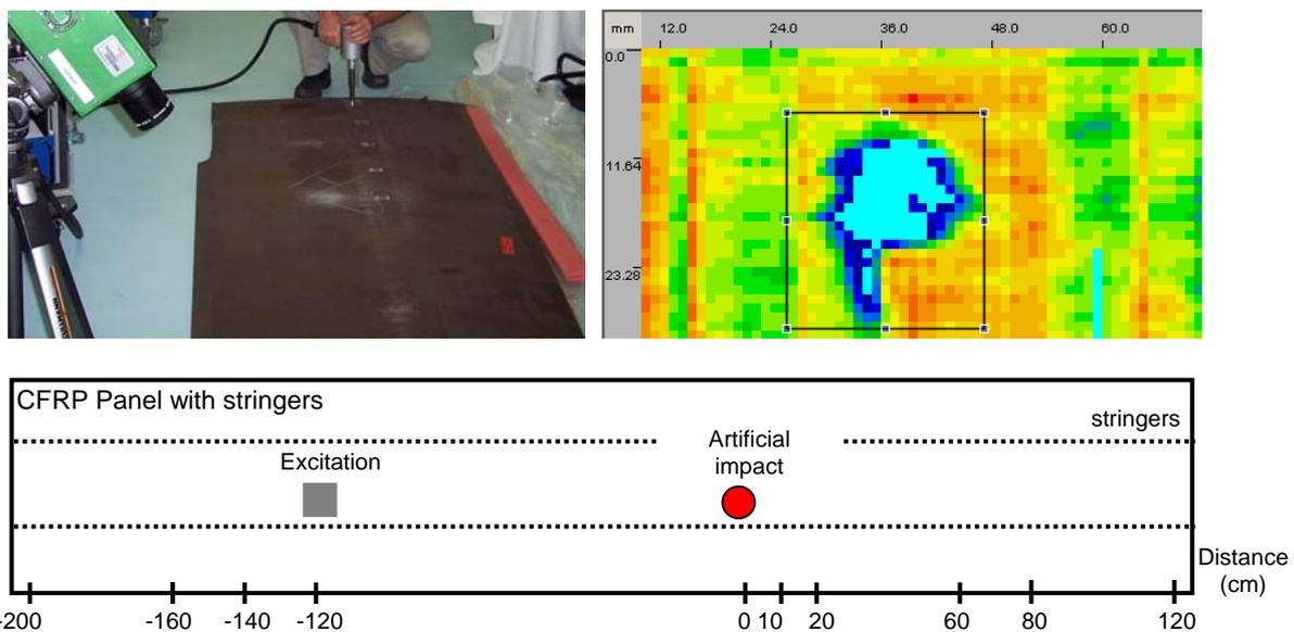
Figure 9: CFRP panel (part 2) with an artificial impact damage (top left), C-scan of the impact damage (top right) and scheme of the CFRP panel showing the different positions of the excitation source.
