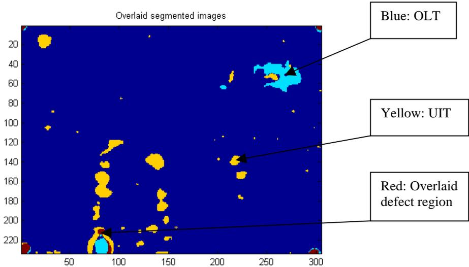
Figure 14: Overlay of segmented UIT and OLT images. The colour areas represent the defect region blue: from the segmented OLT image, yellow: from the segmented UIT data and red the defect area detected in UIT and OLT.
