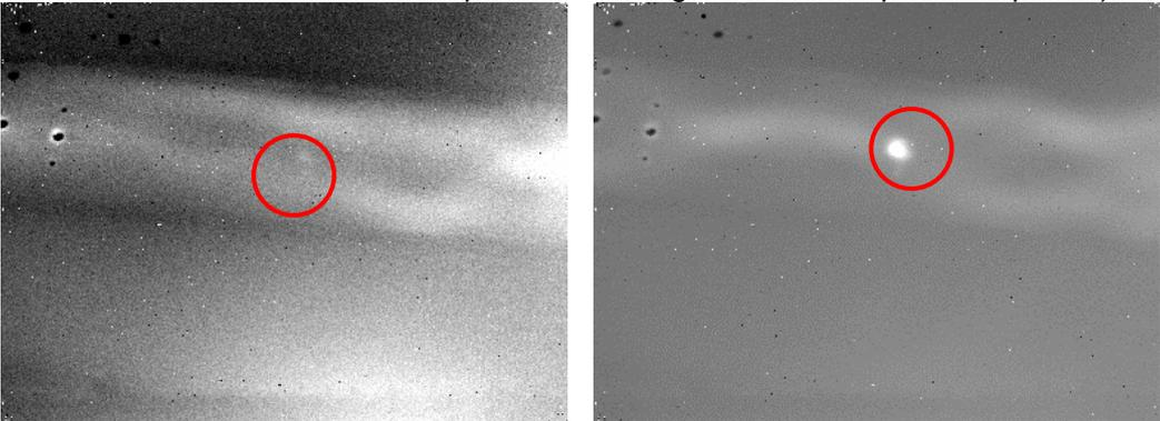
Figure 11: Infrared images with an excitation of power 800 W and 0.8 s duration (left) and of power 1000 W and 1.2 s duration (right) (distance of 80 cm between source and damage).
