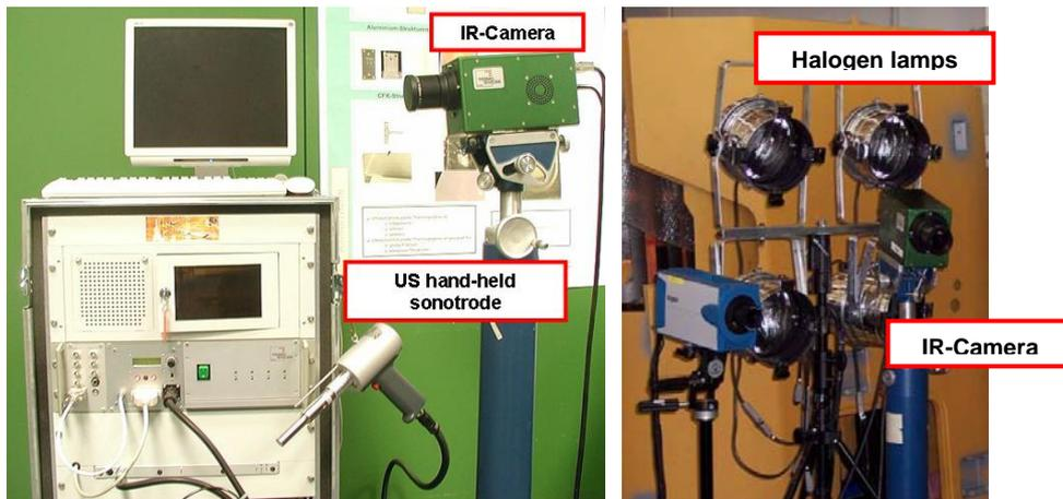
Figure 3: Thermography system with ultrasound gun (left) and with lamps for OLT (right).
