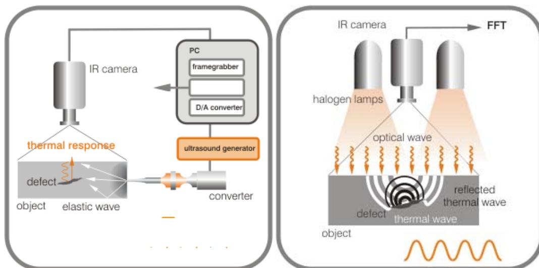
Figure 1: Ultrasound induced thermography (left) and optically excited LockIn thermography (right) [12].
