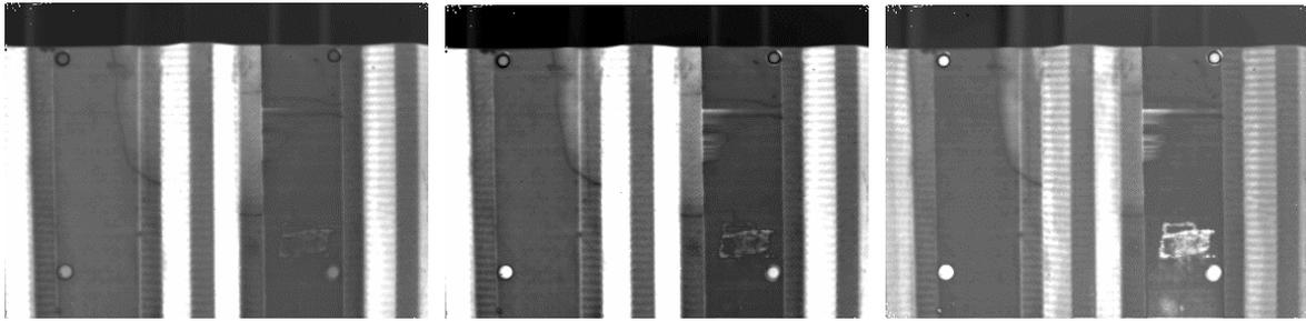
Figure 7: LockIn thermography phase images with different excitation frequencies (from left to right: 0,03 Hz 0,06 Hz and 0,1 Hz).
