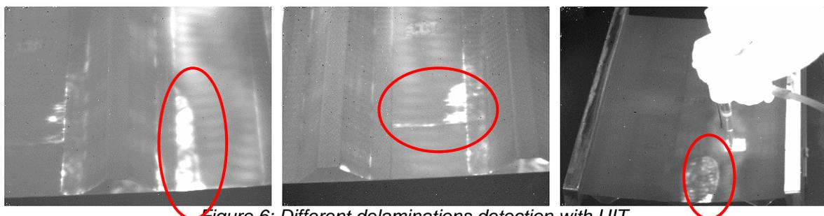
Figure 6: Different delaminations detection with UIT.
