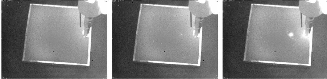
Figure 2: Detection of an impact damage in a composite part (UIT at times 0, 0.22 and 0.93 seconds after the start of ultrasound)
