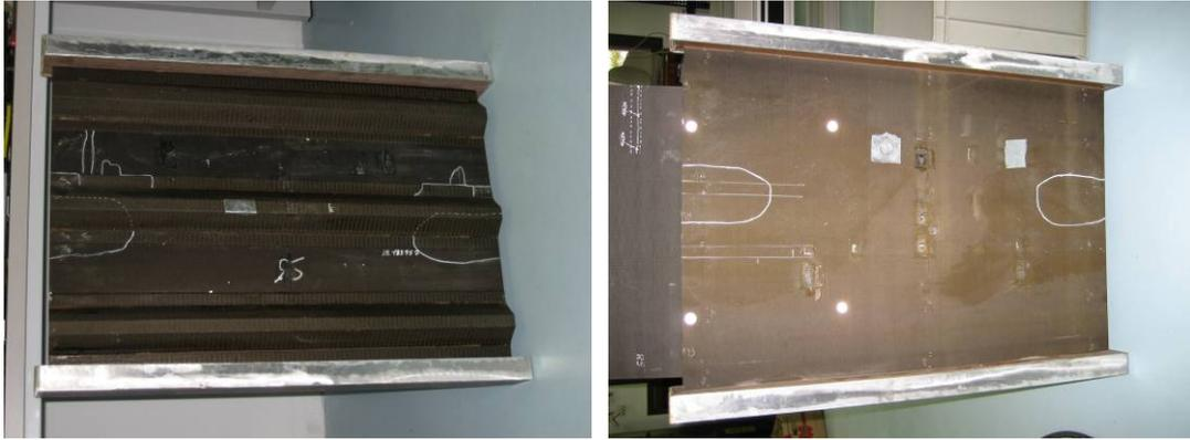
Figure 4: Image of the CFRP stiffened panel: Part 1
