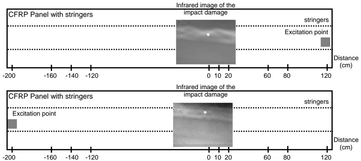
Figure 12: Some results of the detection of the impact damage with distances of 60 cm, 120 cm and 200 cm.
