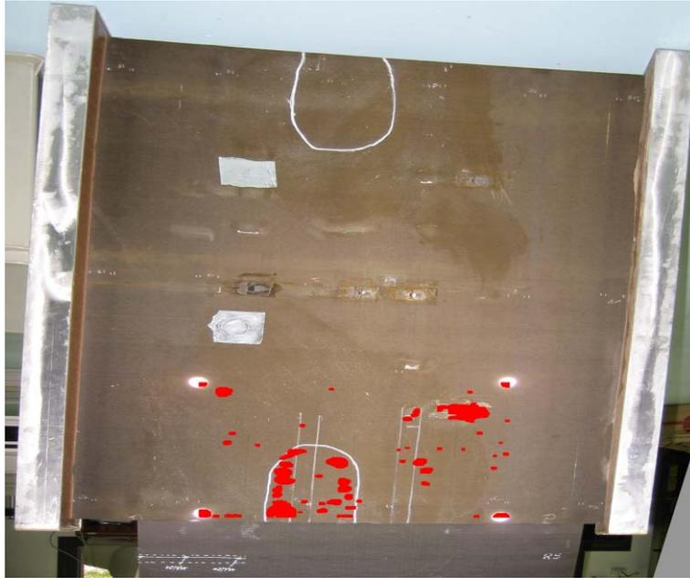
Figure 15: Representation of the defect area on the live image taken with a basic camera (rectified).
