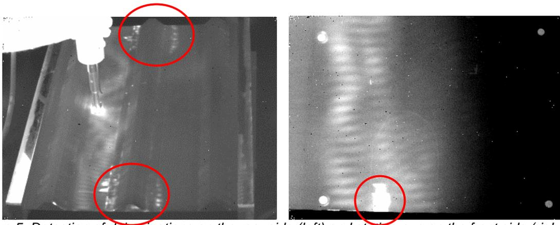
Figure 5: Detection of delaminations on the rear side (left) and static wave on the front side (right) with UIT.
