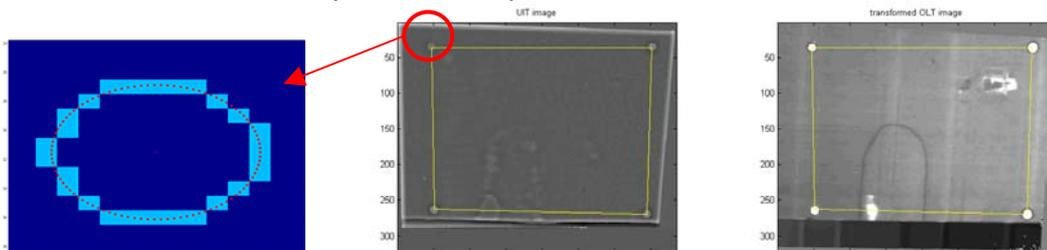
Figure 13: edge detection and ellipse fitting (left), rectified coordinates of the UIT and OLT images (middle and right).
