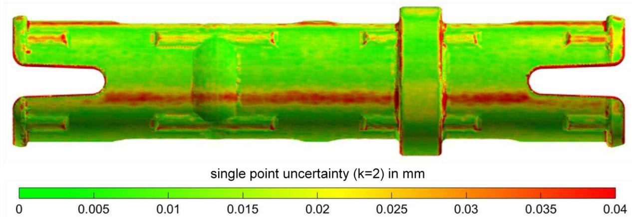
Figure 8: Estimated single point uncertainty of the simulated measurements, calculated from the single point uncertainty and the mean systematic offset (uncertainty map).
