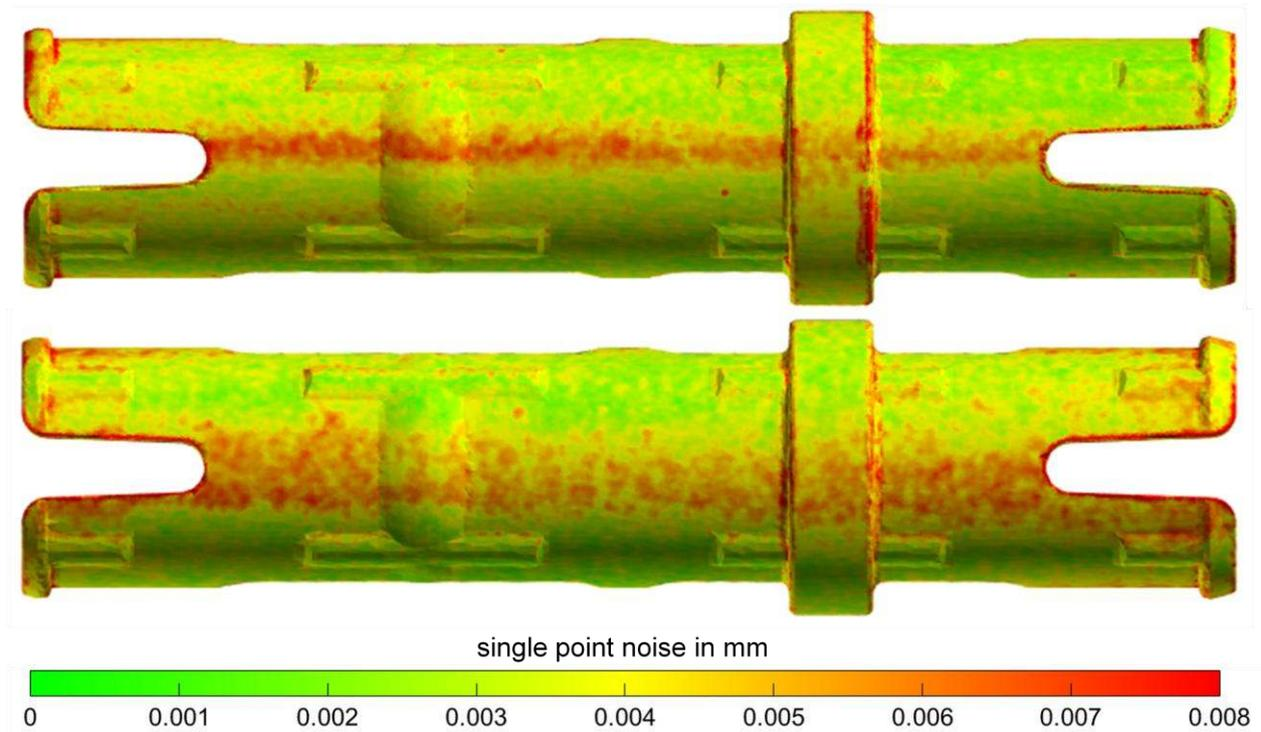
Figure 6: Single point noise of the real (top) and simulated measurements (bottom).
