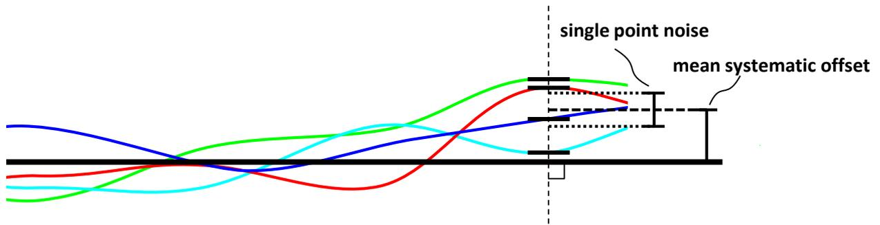
Figure 2: Exemplary calculation of the single point noise and the mean systematic offset for the extracted surface datasets of four different (simulated) measurements of the same object. The single point noise is defined as the standard deviation of a repeated measured surface point in direction of the nominal surface normal at this point. The mean systematic offset is the average of the perpendicular distances.
