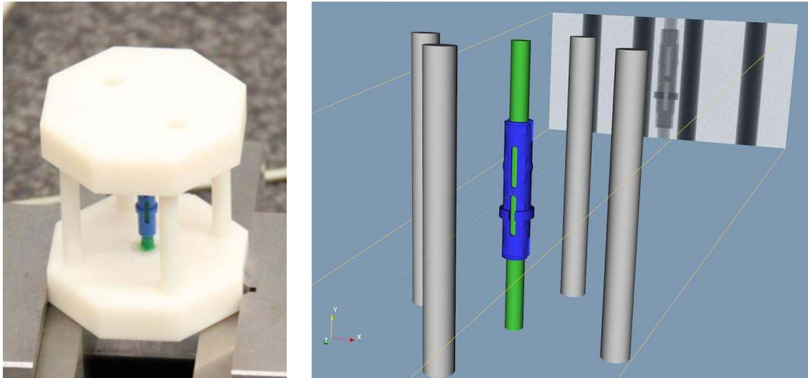
Figure 4: LEGO connector including fixture. The 3D-printed fixture is designed to protect the calibrated connector from damage while still allowing tactile and optical measurements. The right side shows the aRTist scene of the simulation.
