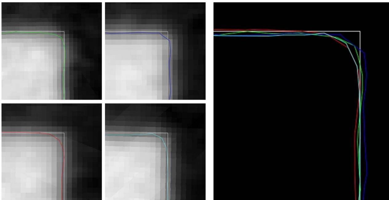
Figure 1: Magnified visualisation of four different scans of the same object including the extracted surfaces (green, blue, red and cyan) and the nominal surface (white). On the right side, the four surfaces are depicted in one image, illustrating the local variations of the extracted surfaces.
