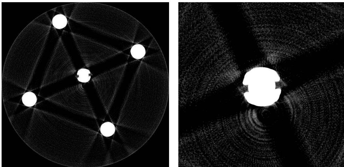
Figure 5: Typical cross-section of a measurement (note that brightness and contrast of images have been heavily adjusted to reveal artefacts). In the magnified visualisation (right), streak artefacts (induced by the fixture) affecting the connector are visible.
