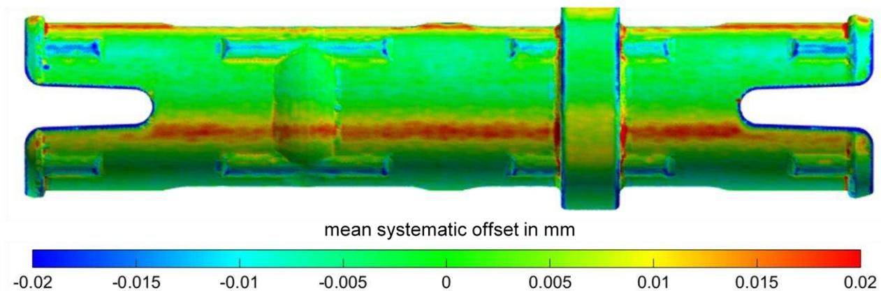
Figure 7: Mean systematic offset of the series of simulated measurements.
