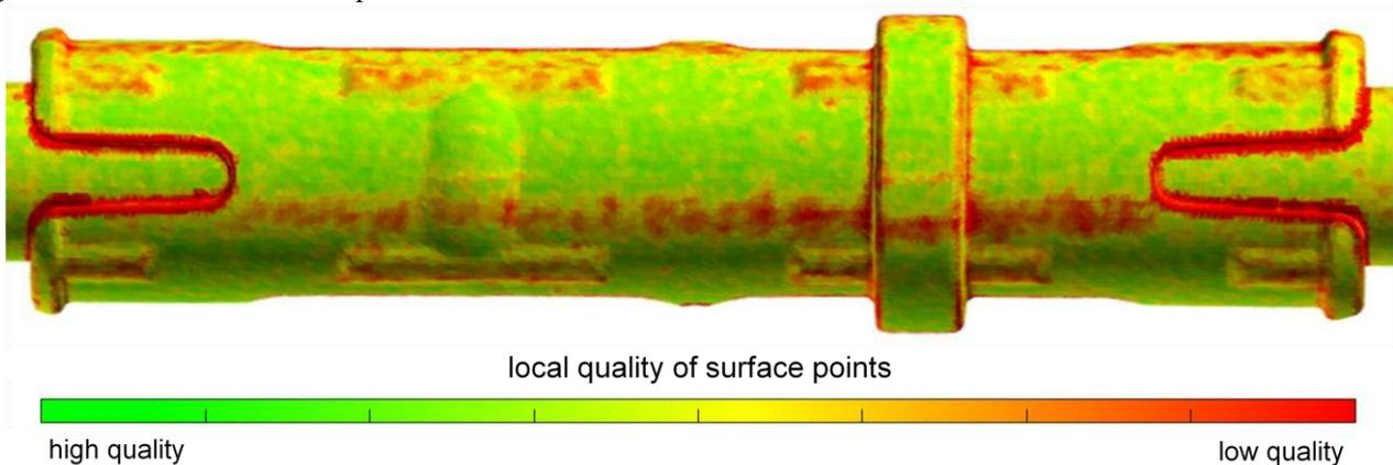
Figure 9: Colour-coded visualisation of the local quality value (LQV) for a single real measurement of the connector to verify the single point uncertainty. The quality values are calculated by analysing the symmetry and homogeneity of the grey values in the proximity of the extracted surface points. A good agreement to the simulated single point uncertainty (Figure 8) is evident.
