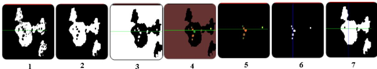
Figure 4: An image processing sequence for filling internal pores and for calculating volume of agglomerate including internal pores ( $V_{agg}$ ): (1) Binary image, (2) Closing-cube (fill small pores), (3) Complement (invert the images), (4) Labeling (identify the objects), (5) Object filter (filter out the air), (6) Binarization, (7) fill all pores (combine steps 6 and 2).
