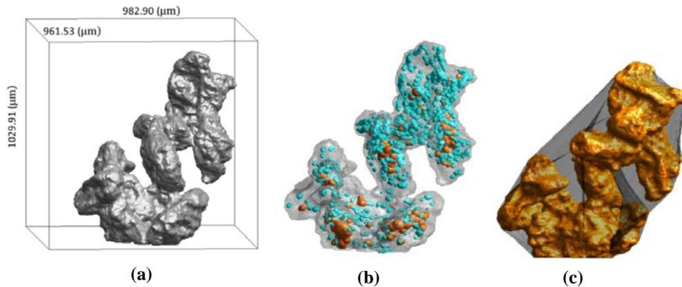
Figure 6: (a) The overall 3D view of maltodextrin agglomerate from X-ray images, (b) the spatial distribution of internal pores, (c) the total volume of agglomerate defined by convex hull method to calculate the porosity of open pores.
