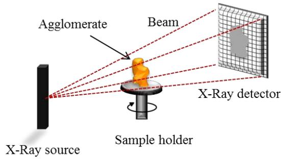
Figure 2: Principle of  $\mu$ -computed tomography.
