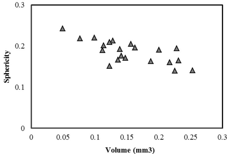
Figure 8: Sphericity of different agglomerates calculated from 3D X-ray images.
