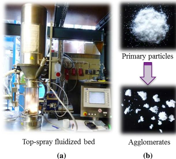
Figure 1: (a) The experimental lab-scale set-up for spray fluidized bed and (b) maltodextrin powders and agglomerates.
