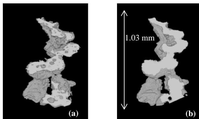
Figure 5: Cross-sectional 3D volume view of an agglomerate: (a) before and (b) after filling its internal pores.
