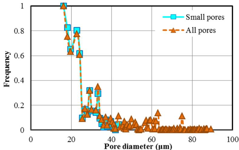
Figure 7: Normalized frequency distribution of internal pores represented by applying closing morphology and labeling method for distinguishing small and large pores.
