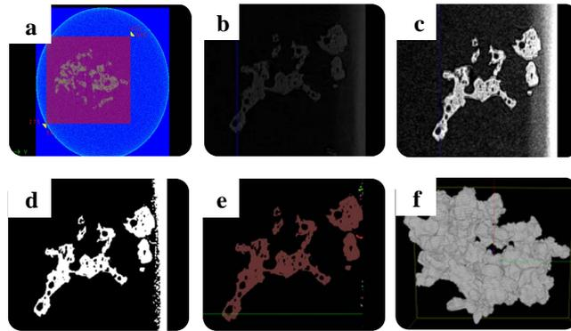
Figure 3: The procedure of image processing: (a) the cross sectional view of original image, (b) extract the region of interest, (c) binarizing the image, (d) removing noise by filtration, (e) removing sample holder effect by labelling and object filter, (f) volume rendering.
