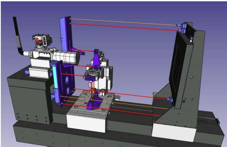
Figure 3: Concept of the cone-beam CT geometry measurement system used to determine the position of the X-ray tube (left), sample (middle) and detector (right): The system consists of eight fibre interferometers (red laser beams), five straightness sensors (orange laser beams), an X-ray tube measurement system, and an index sensor that are all referred to a metrology frame (blue frame on the left).
