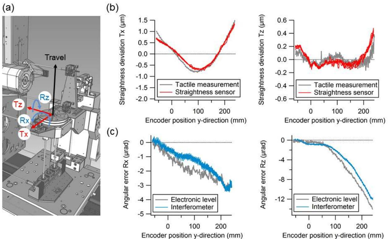
Figure 7: Evaluation of the CT geometry measurement system (coloured curves) against reference measurements (grey curves, data from Reference [3]): (a) Coordinate system for the guideway error measurements of the sample stage. (b) Home-built straightness sensors (red curves) compared to tactile measurements against a straight edge (grey curves). (c) Angular measurements using the differential interferometers (blue curves) and electronic levels (grey curves).
