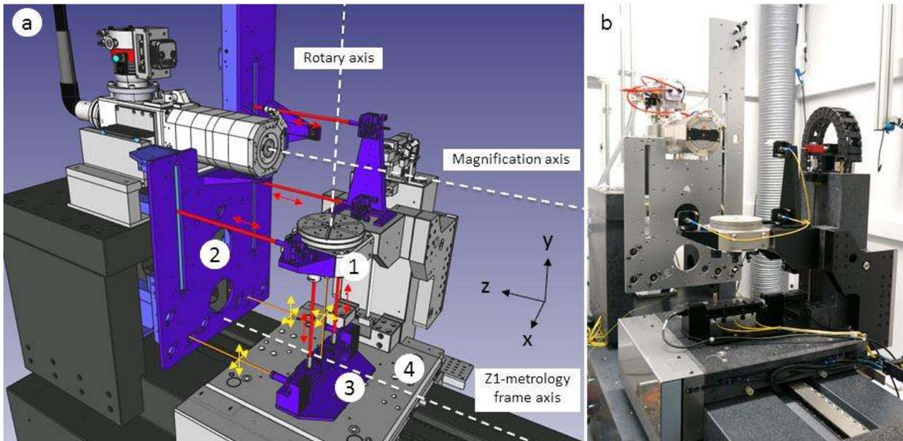
Figure 6: (a) Detail of the sample stage measurement system: To relate the sample stage (1) position to the metrology frame (2), an intermediate metrology frame (3) on the Z1-stage (4) is used. Interferometer laser beams are depicted in red and straightness sensors in orange; the corresponding measurement directions are indicated. The point of interest is the intersection between the rotary and the magnification axis. (b) Photograph of the implementation.
