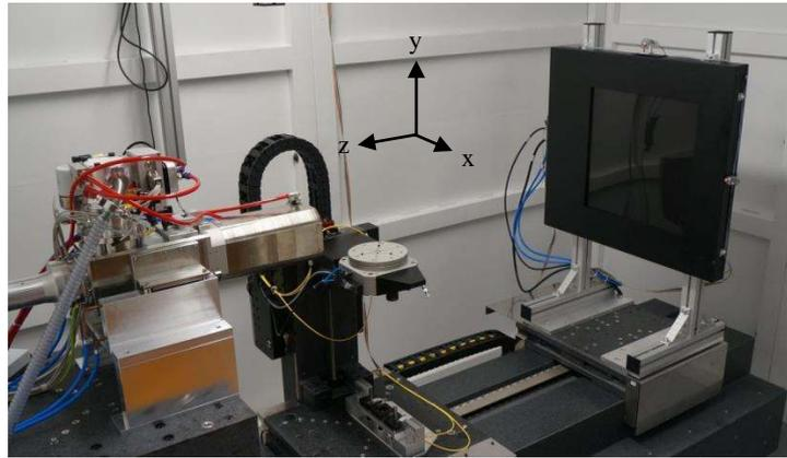
Figure 1: METAS-CT consisting of a microfocus transmission X-ray tube, an air-bearing positioning system and a 4k x 4k detector. The photograph shows the system before the implementation of the metrology system.
