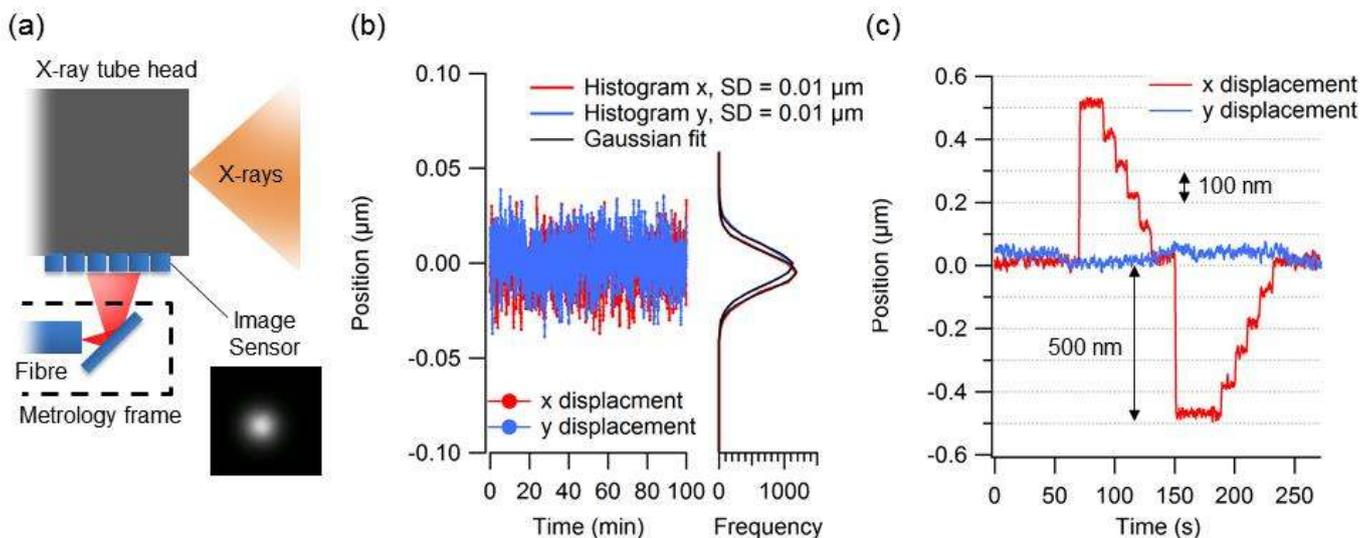
Figure 4: Image sensor based measurement system: (a) Principle: A laser beam from a single-mode fibre is incident on a CMOS camera chip attached to the X-ray tube. The centre of the beam is determined and equals the lateral displacement between the X-ray tube and the incident laser beam. (b) Stability measurement: The intrinsic noise floor of the sensor was 10 nm ( $1 \sigma$ ). (c) Displacements of 100 nm and 500 nm were realised using a linear stage and accurately measured by the sensor.
