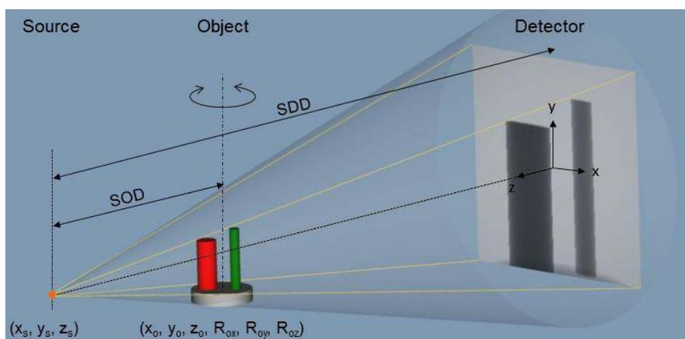
Figure 2: The geometry of a cone-beam CT consists of 9 degrees of freedom (DoF) under the assumption of a point source and an ideal detector. The X-ray source coordinates are  $(x_s, y_s, z_s)$ , the object is positioned at  $(x_o, y_o, z_o)$  with rotation angles  $(R_{ox}, R_{oy}, R_{oz})$  with respect to the detector reference system.
