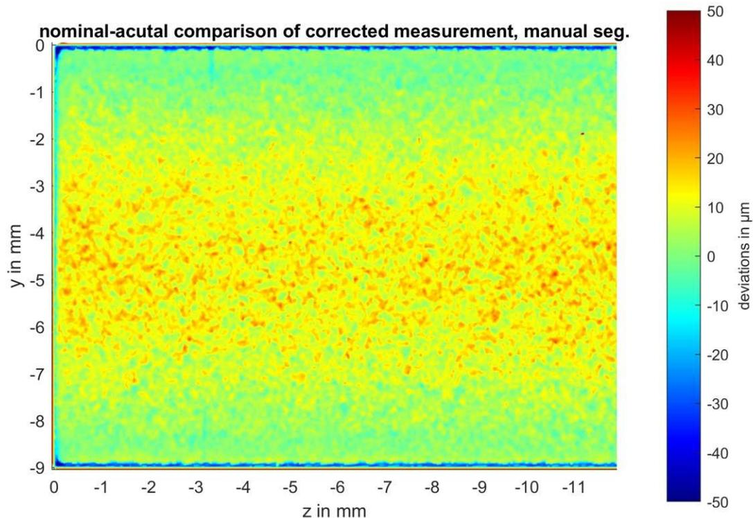
Figure 10: Nominal-actual comparison of corrected measurement and CAD for manual surface determination.
