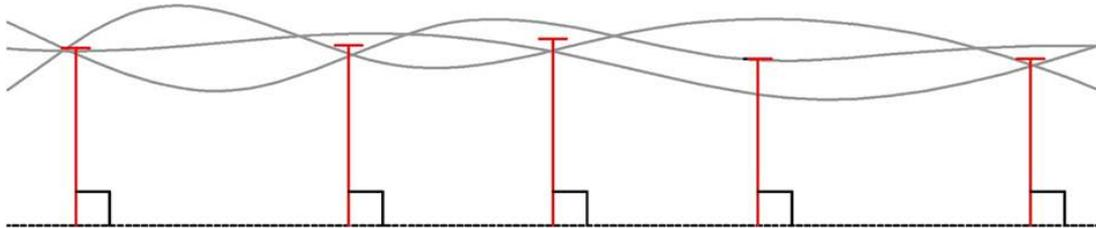
Figure 1: Sampling of the simulated surfaces (grey) with search rays (red) orthogonal to the CAD-surface (black) for the determination of the local mean deviation (systematic error).
