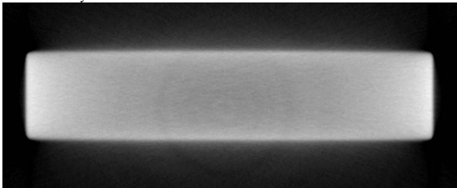
Figure 3: Cross-sectional view of the volume data of the measurement. Different artefacts which hinder segmentation and subsequent dimensional measurement are visible.
