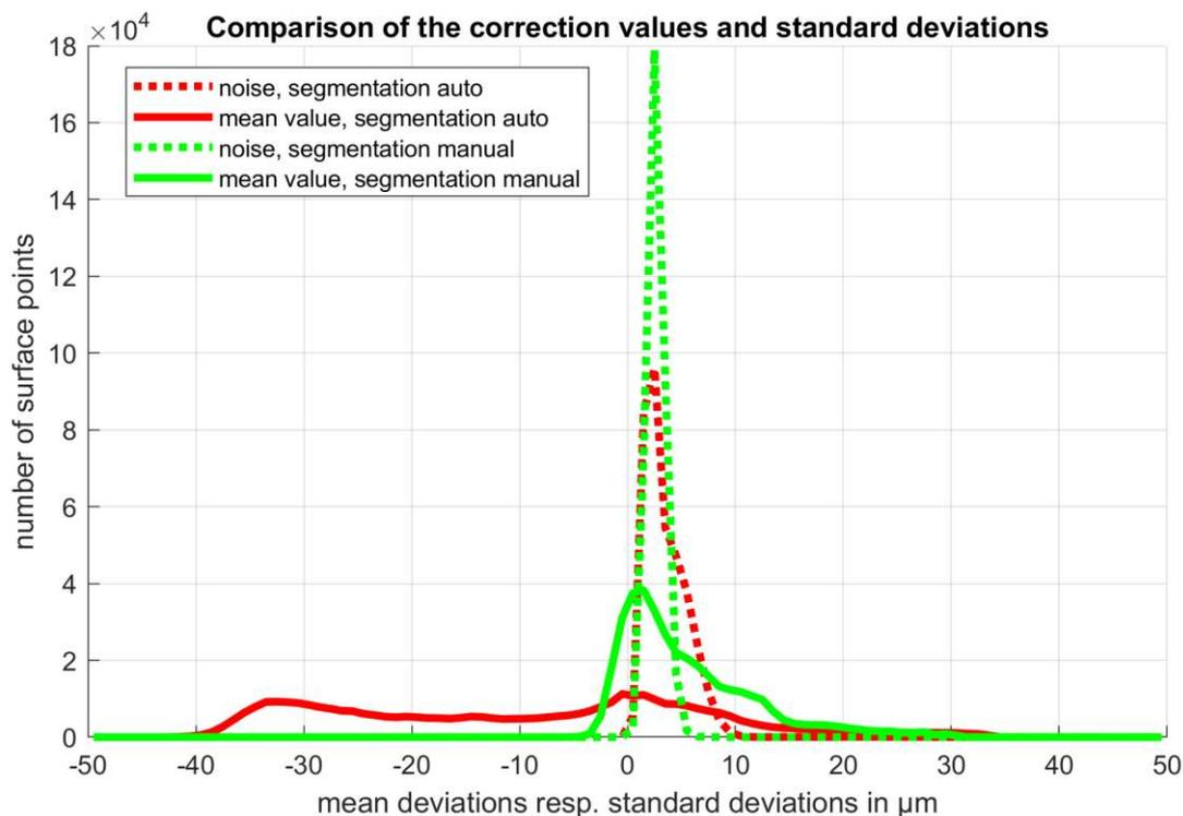
Figure 11: Histograms of the magnitude of the correction vector (with the sign indicating ‘in the direction of’ or ‘in the opposite direction of the normal vector’) (lines) and its standard deviation (dotted lines) for both segmentation modes in comparison.
