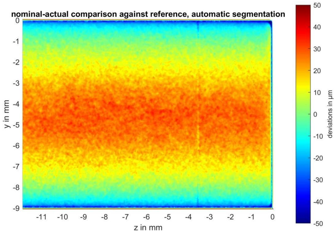
Figure 6: Nominal-actual comparison of measurement and CAD for automatic surface determination.
