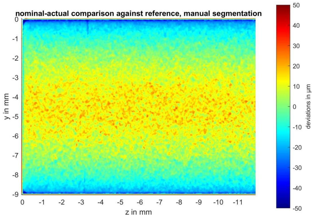
Figure 7: Nominal-actual comparison of measurement and CAD for manual surface determination.
