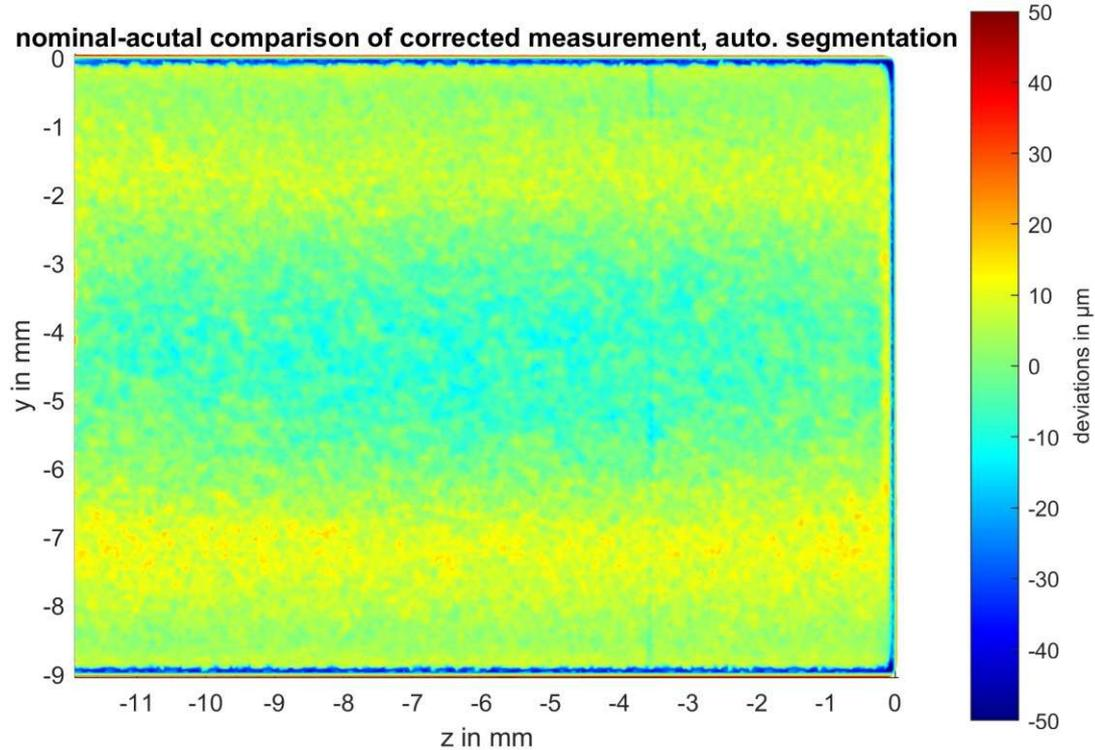
Figure 9: Nominal-actual comparison of corrected measurement and CAD for automatic surface determination.
