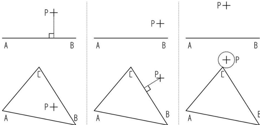
Figure 2: Illustration of the three different cases for the closest point search described in '4. Correction of the real measurement data' in chapter 2. The point P is a point from the measurement surface, the triangle ABC represents the CAD surface.
