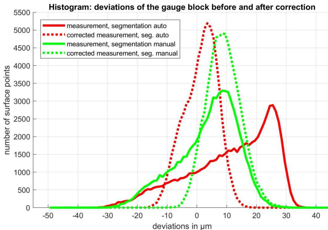
Figure 8: Histogram of the deviations on both side surfaces of the measurement from the CAD before and after correction for both segmentation methods. The point density on the surfaces is homogeneous so that the number of points corresponds to the occupied surface.
