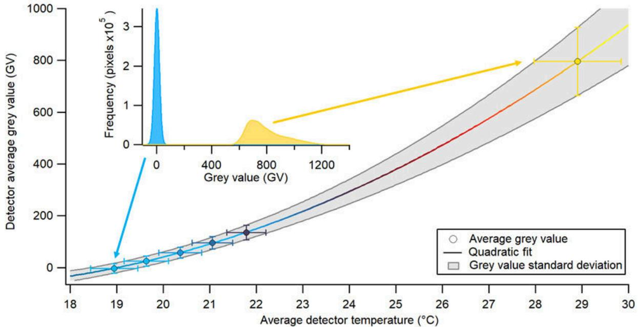
Figure 4: Average dark grey value across all detector pixels relative to the detector average temperature; error bars indicate grey value (vertical) and temperature (horizontal) standard deviations across the detector. The following cooling settings were used: Water-cooling setpoints 16 °C to 20 °C in 1 °C steps, and air-cooling. The inset shows the grey value histogram for water-cooling at 16 °C (blue) and air-cooling (yellow).
