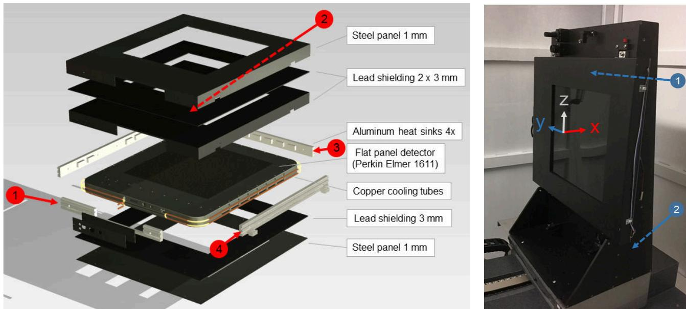
Figure 1: Left: CAD of the flat-panel detector cooling and shielding system in exploded view. The numbers indicate the positions of four detector housing temperature sensors. Right: Photo of the shielded and water-cooled flat-panel detector mounted on an aluminium supporting frame. The numbers indicate the positions of two detector mount temperature sensors.
