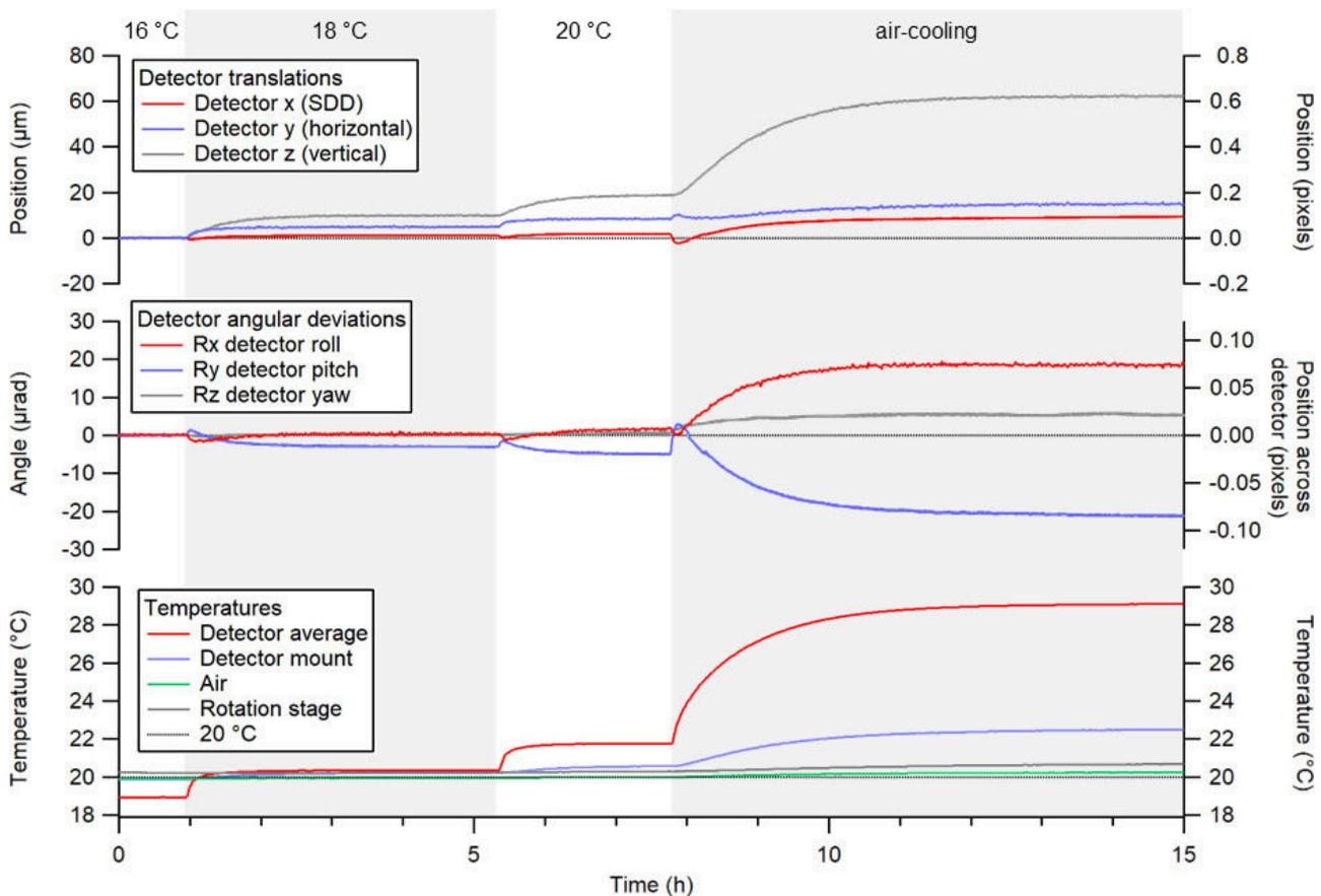
Figure 3: Detector position (top), angular deviations (middle), and CT system temperatures (bottom) under different cooling settings (thermostat setpoints: water-cooling 16 °C (baseline; no heat transfer into the CT system), 18 °C, 20 °C and air-cooling); see Figure 1, right for coordinate system.
