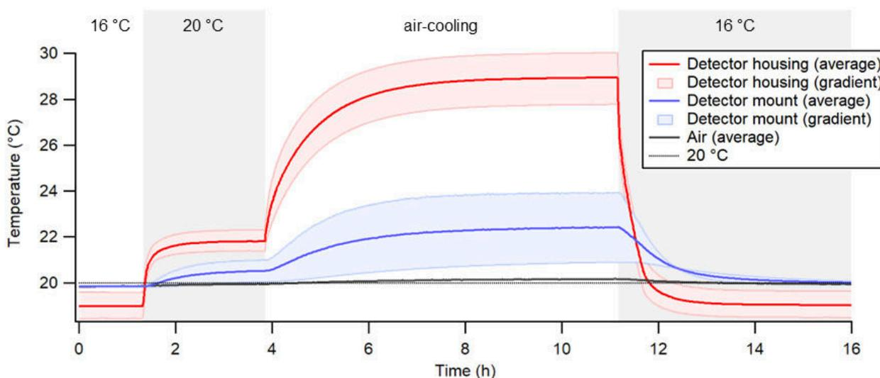
Figure 2: Detector housing (red) and mounting structure (blue) temperatures and air temperature (black) under different cooling strategies: Water-cooling 16 °C (no heat transfer into the CT system) and 20 °C, and air-cooling. Temperature sensor positions are indicated in Figure 1.
