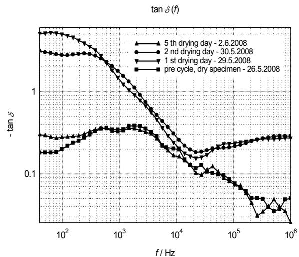
**Fig. 3.** Roofing tile loss factor versus frequency for various water contents (both frequency and loss factor are plotted in log scale)
