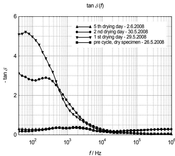
**Fig. 2.** Roofing tile loss factor versus frequency for various water contents
