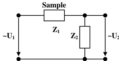
**Fig. 1.** Circuit diagram for the unknown impedance  $Z_1$  to be measured and the known value impedance  $Z_2$ .
