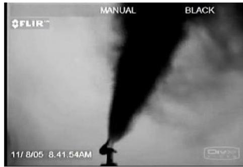
Petrochemical facilities such as refineries offer a target rich environment for VOC leaks. The remote imaging capabilities of IR cameras such as the ThermaCAM® GasFindIR™ dramatically reduce the task of finding leaks. Even when gases have a low contrast with their surroundings, the movement of the gas in a static environment makes finding small leaks, or larger leaks at greater distances feasible. Figures 14 and 15 show some examples of refinery applications.
