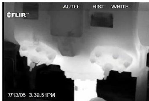
Figure 16. Gasoline fumes cascading from fill spout onto pavement.
