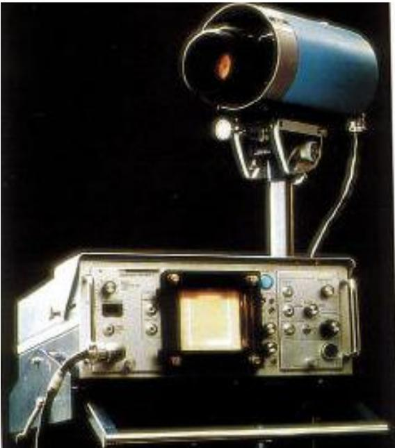
**Fig. 5:** One of the medically broadly used AGA Thermovision cameras (AGA 680 medical, ca. 1975)
