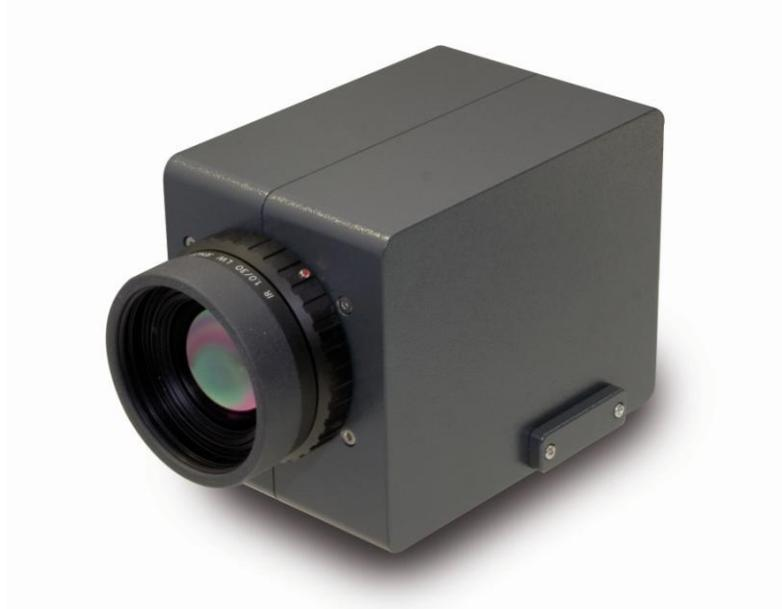
**Fig. 8:** Enhanced resolution 384x288 stationary FPA microbolometer IR camera Jenoptik VarioCam HR used for MammoVision and ReguVision
