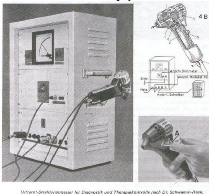
**Fig. 1:** First medical thermographic device, developed by SCHWAMM und REEH 1953
