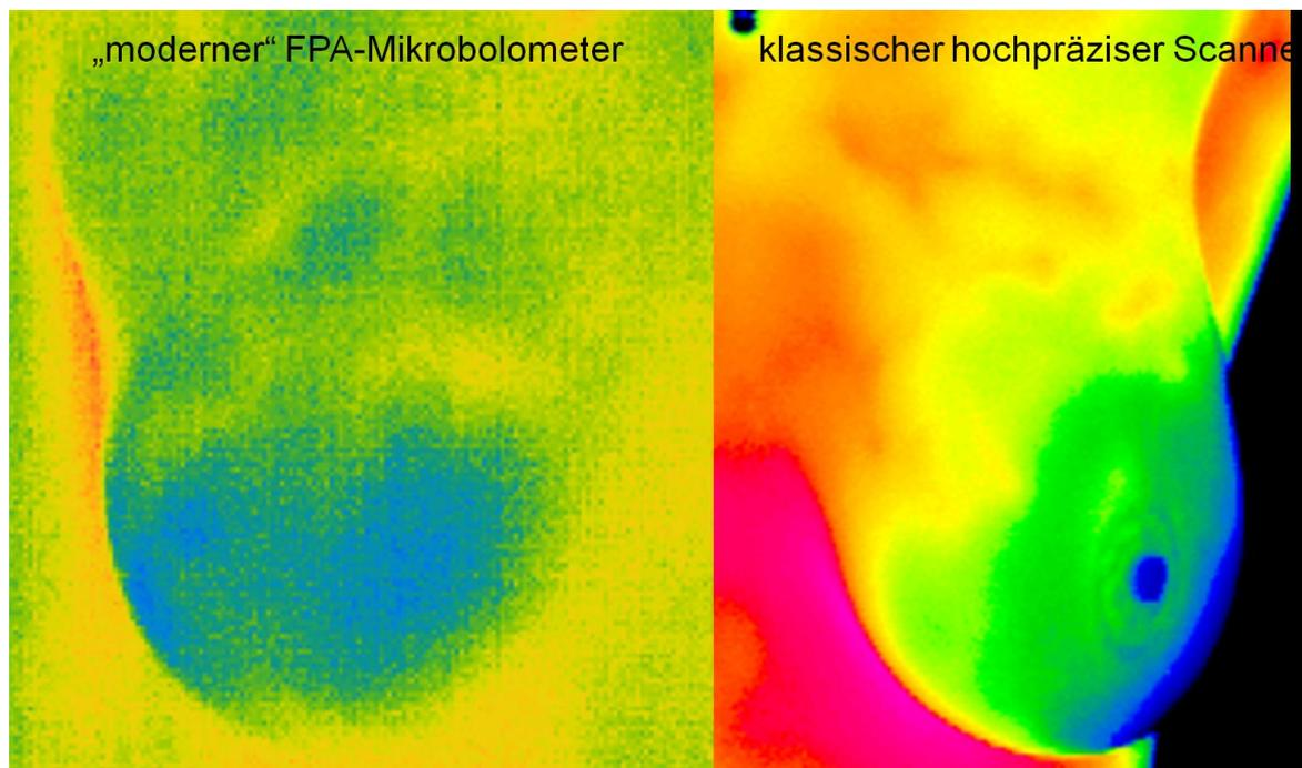
**Fig. 6:** Images of an early uncooled FPA microbolometer camera, compared to cooled MCT scanner (both built in the late 1990s)
