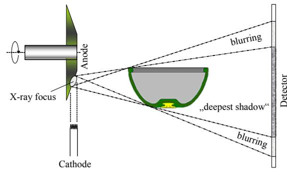
**Figure 5:** The inclination of the anode controls the optical size of the X-Ray focus. A larger X-ray focus increases the blurring of the image.
