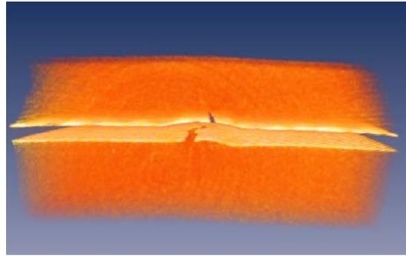
Figure 9: 3-D reconstruction of the membrane rupture.
