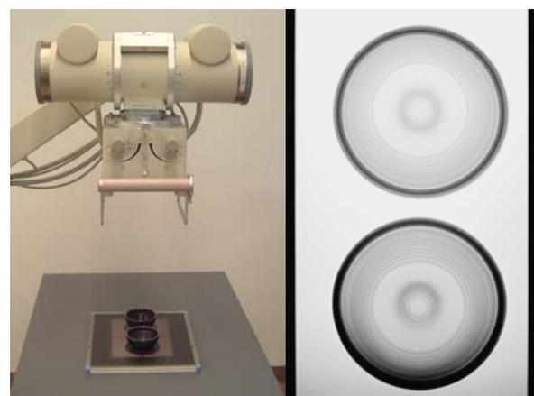
**Figure 2:** Setup of the X-ray fluoroscopy system with a digital cassette (resolution 2364 x 2964 pixel) and data of reference membrane (top) and membrane after test series (bottom).
