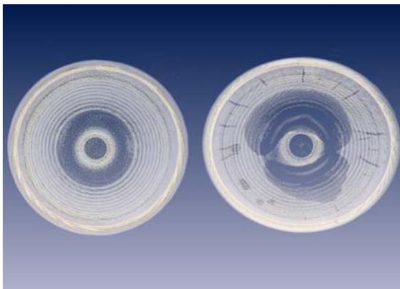
**Figure 3:** 3-D reconstruction of the CT data of reference membrane (left) and membrane after test series (right).
