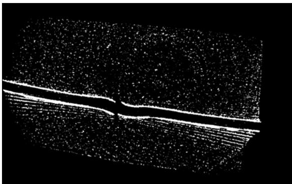
Figure 8: Single tomographic section of the membrane rupture.
