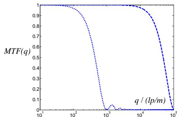
**Figure 6:** Frequency dependent modulation-transfer-function of conventional CT (dotted curve) and micro-CT (dashed curve).
