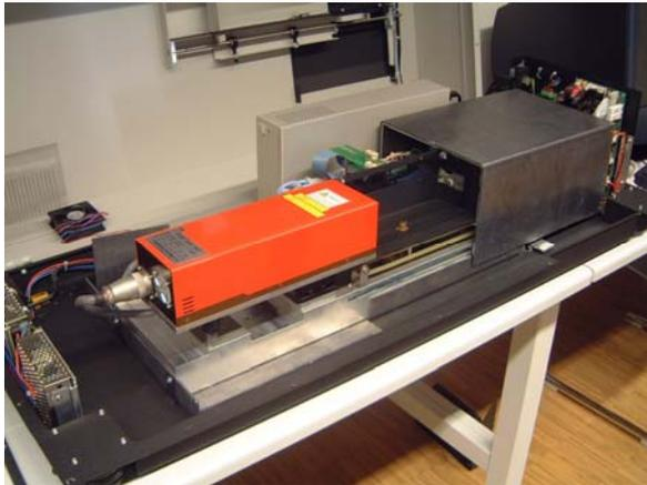
Figure 7: Setup of micro-CT.
