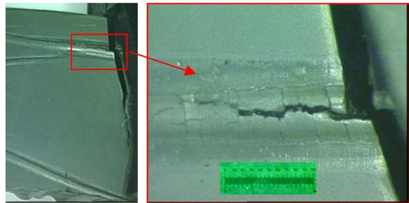
Figure 10: Microscope picture of the fold structure (width approx. 1 mm).
