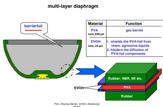
**Figure 1:** Overview of multi-layer diaphragm assembly.
