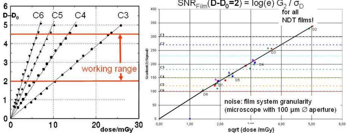
**Fig. 2:** Determination of image quality parameter  $SNR_N$  by NDT film system classification according to EN 584-1 (radiation quality 220 kV, 8mm Cu filter).
