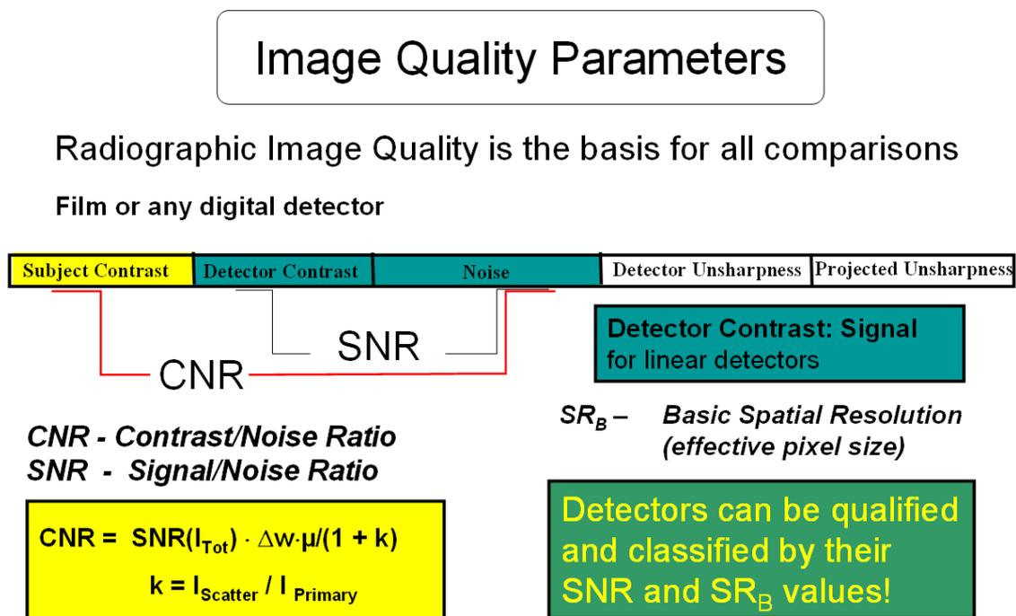
**Fig. 1:** Relationships between image quality parameters of radiographic image detectors (from [7])
