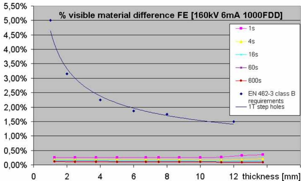
**Fig. 14:** Visibility limits of 1T step hole IQI of EN 462-2 acc. to the requirements of EN 462-3, testing class B for film radiography and visible material difference for 1mm – 13mm steel (V4A) and different integration times for DDA (RID512AF1 by Perkin Elmer).
