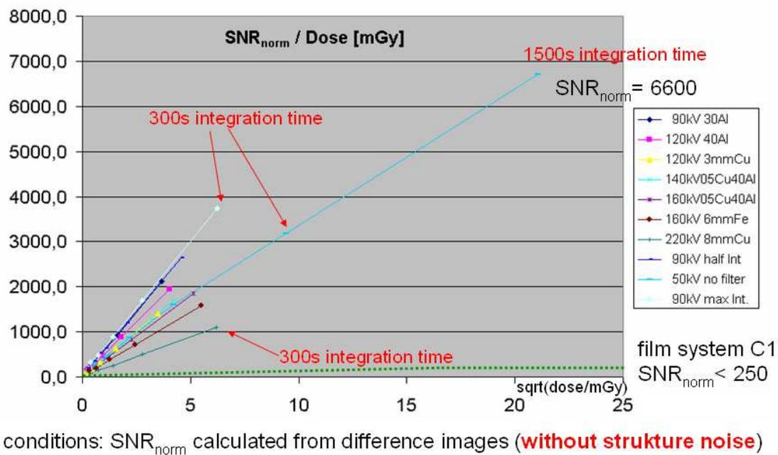
**Fig. 11:** Improvement of normalized  $SNR$  by image integration in the computer. Detector: DIC 100TL of company Ajat. The slopes of the lines characterise the detector efficiency at the selected radiation quality (energy).
