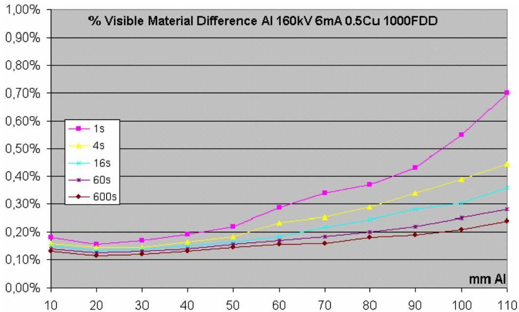
**Fig. 13:** Visible material difference (%) in Al from 10mm to 110mm wall thickness and different integration times. Detector: RID512 AF1 of Perkin Elmer. A similar contrast resolution can be achieved with steel too (see fig. 14).
