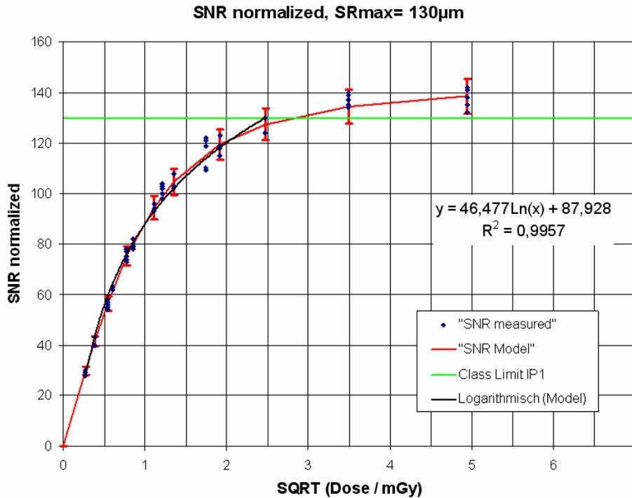
**Fig. 6:** Example of saturation of  $SNR_{Norm}$  by structure noise with the Fujifilm system XG-1 scanner and ST-VI imaging plate. The maximum achievable  $SNR_{Norm}$  value is 142.
