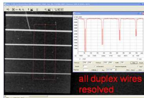
**Fig. 5:** Examples of CR systems and their measured basic spatial resolution:
