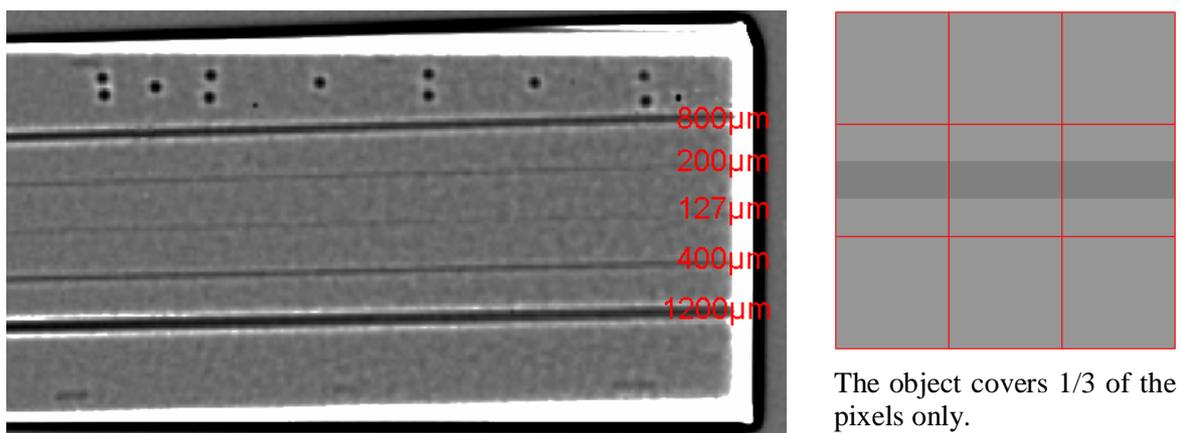
**Fig. 15:** Digital radiograph of a test wedge (5mm to 40mm Aluminium) with longitudinal drilled cross-bore holes of different diameters. With high SNR even details smaller than 1 Pixel are visible (shown image: high pass filtered). This effect is called sub-pixel resolution.
