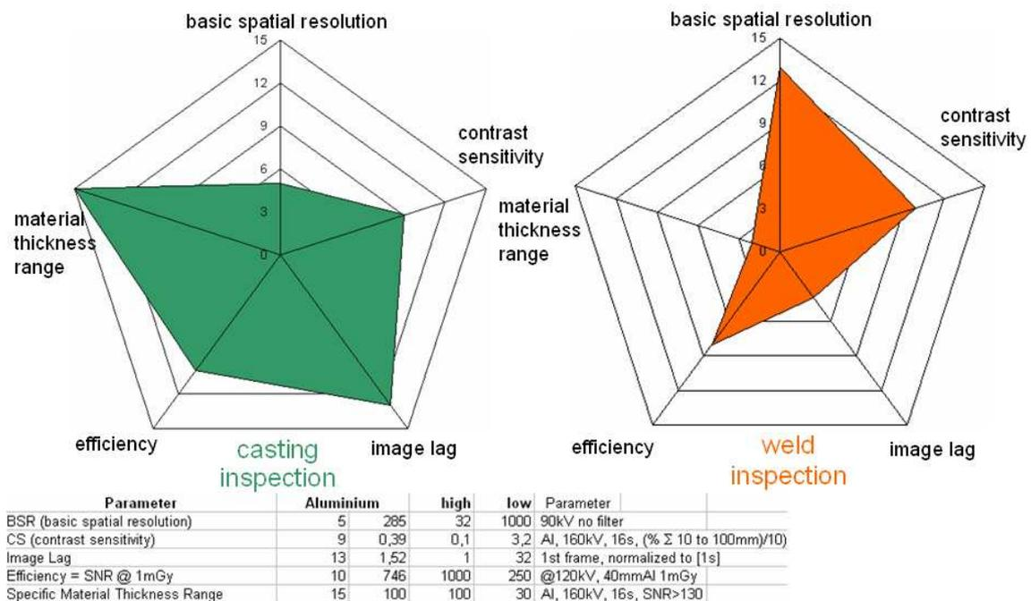
**Fig. 16:** Presentation of results of the ASTM draft on “DDA manufacturing qualification”, left: DDA optimized for inspection of castings, right: DDA for weld inspection
