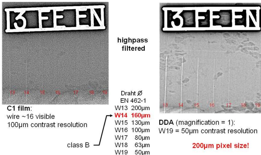
**Fig. 9:** Comparison of visibility of wire type IQIs according to EN 462-1 for film (left) and DDA (right) at 8mm wall thickness (images high pass filtered for better visualization). The improved SNR of the DDA allows to detect the wire W19 (50  $\mu m$  diameter) at a pixel size of  $200\mu m$ !
