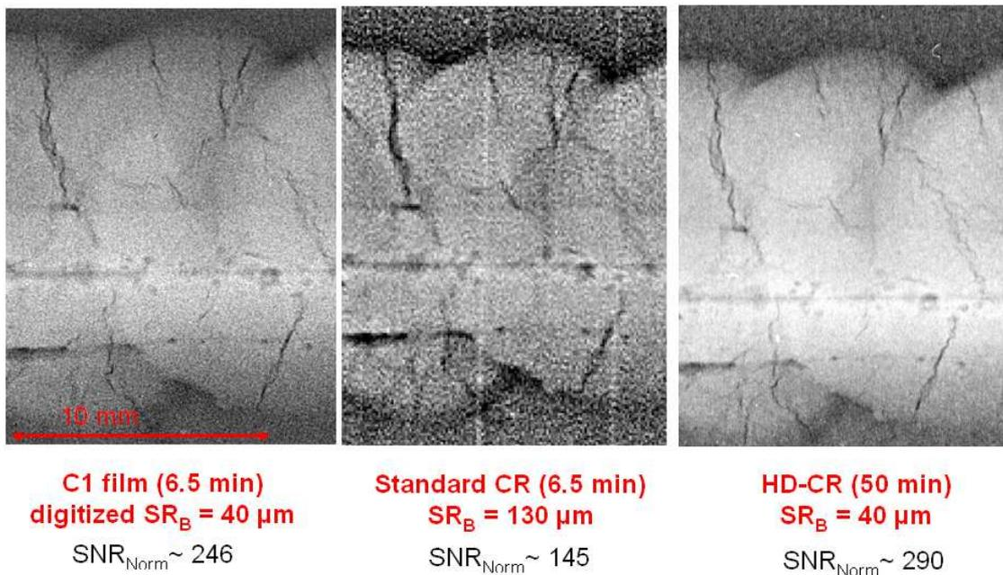
**Fig. 7:** Comparison of a section of the BAM 5 test weld obtained with the best NDT
