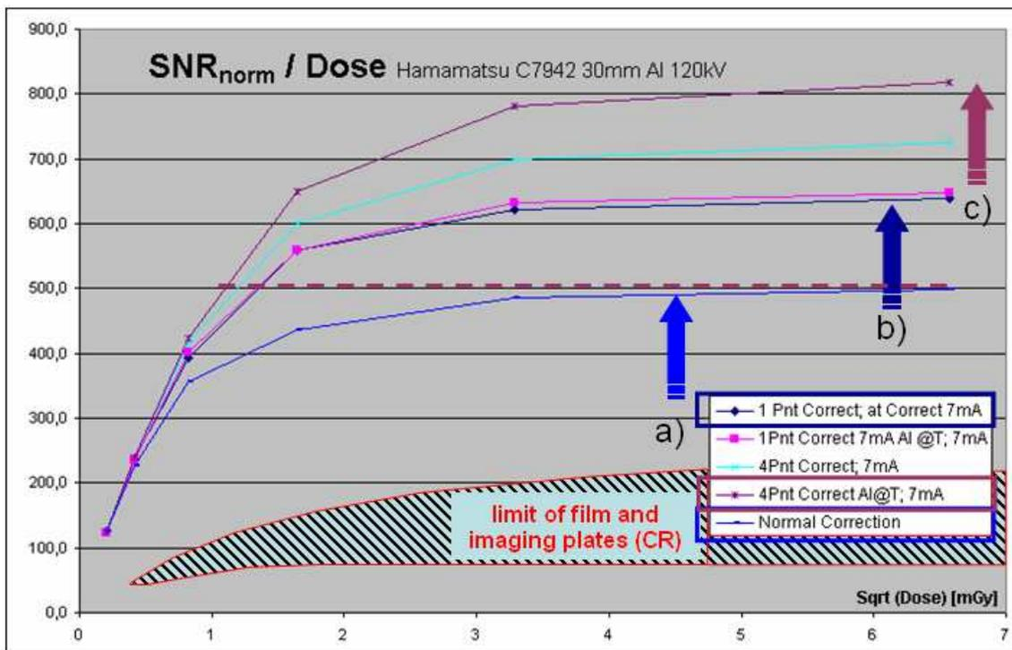
**Fig. 12:** Achievable  $SNR_{Norm}$  with different detector calibrations. Detector: Hamamatsu C7942, exposures with 120 kV, 7mA and 30mm Aluminium.
