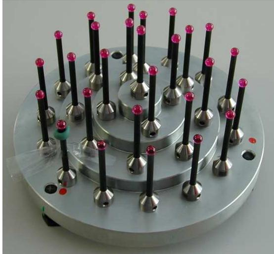
Figure 1. Calibrated test piece for accuracy/ repeatability determination consisting of 27 ruby spheres.
