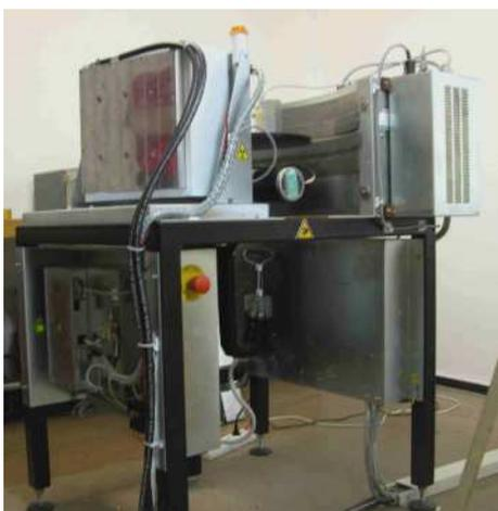
**Fig. 1 – The X-Ray dual-energy Radioscopy and Tomography laboratory equipment**
