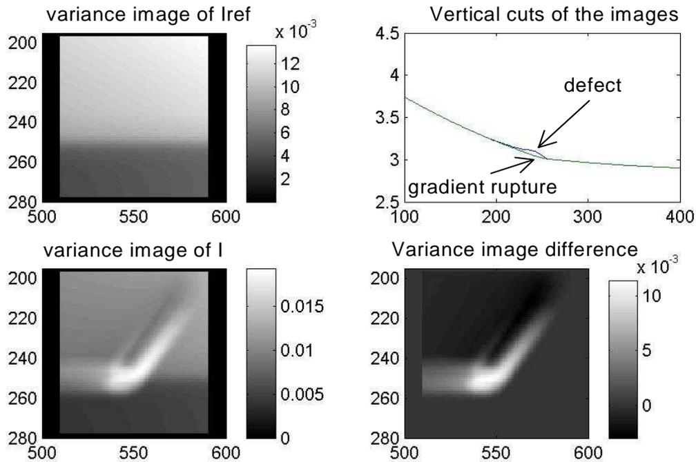
Figure 4 left : Variance image of the reference image and the raw image; right : grey-level profiles in the image  $I$  (crossing the defect) and  $I_{ref}$ , and difference of the two variance images, enhancing the defect.
