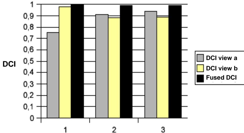
Figure 10 Fusion of the DCI for three different defects matched in two views.
