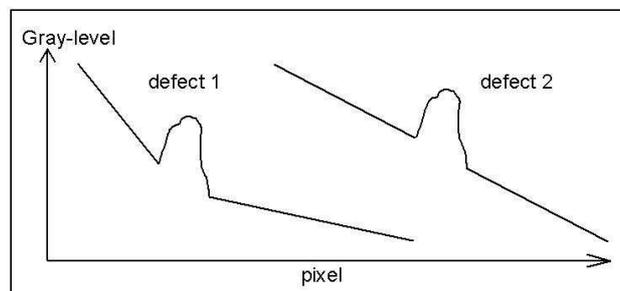
Figure 3 Two defects with the same background gradient but with a variation of gradient (defect 1) or with a constant gradient (defect 2)
