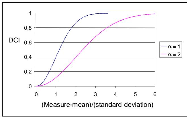
Figure 5 DCI obtained using the relation (1) with a weighting factor of 1 or 2.
