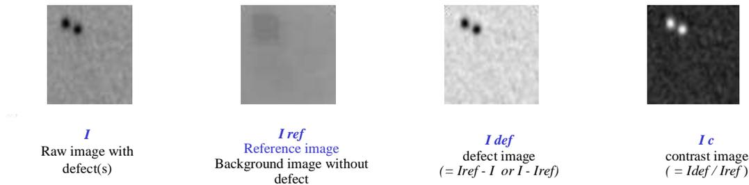
Figure 1 Example of a radioscopic image with darker defects : from left to right : initial image  $I$ , background image without defect,  $I_{ref}$ , defect image  $I_{def}$ , contrast image  $I_c$ . The  $I_{ref}$  image was obtained by a morphological closing of image  $I$ .
