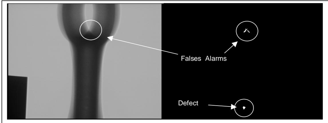
Figure 7 Raw and binary image after automatic segmentation.
