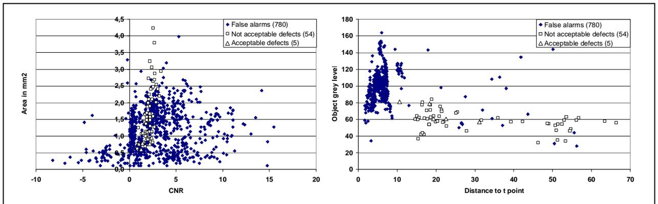
Figure 8 Features representation of the detected objects : (left) area versus CNR and (right) object grey level versus the distance  $D_t$ .
