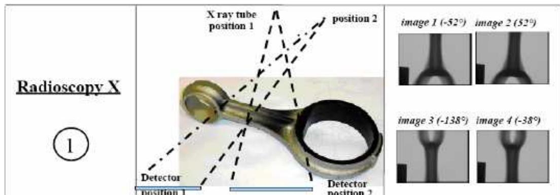
Figure 6 Acquisition of images of the connecting rod in the frame of the QUME project : the four angles were selected for a best inspection of the critical zones.
