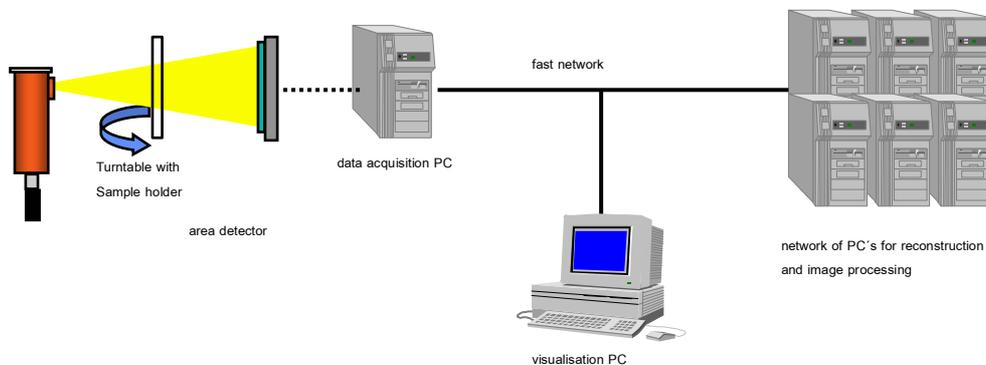
Fig. 2: Set up of inspection system
