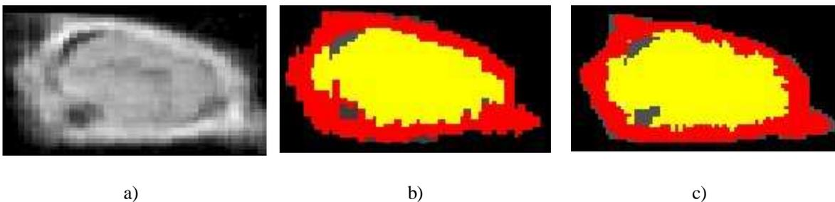
Fig. 8: a) Original slice of a voxel volume. b) Segmentation of a) by hand. c) Automatic segmentation of a) using the proposed method.
