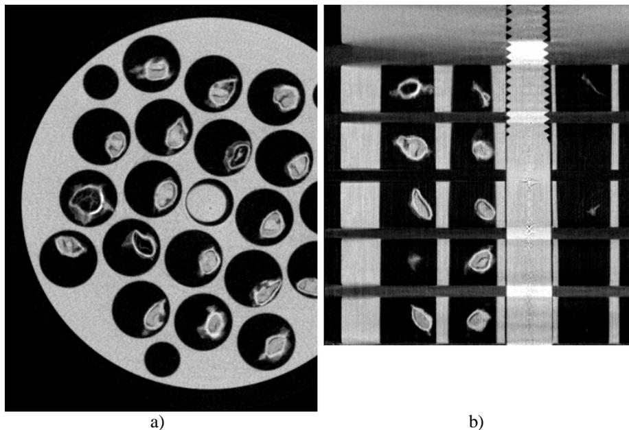
Fig. 5: Reconstruction of the disc filled with sugar beet seeds. a) XY slice. b) XZ slice.
