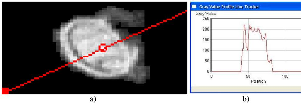
Fig. 7: a) Central slice of a seed volume with a radial line. b) Grey value profile of the radial line in a).
