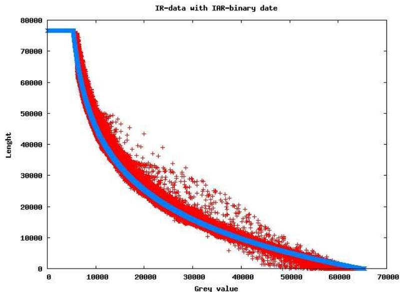
Figure 2. IR-point cloud with path lengths from IAR-binary volume.
