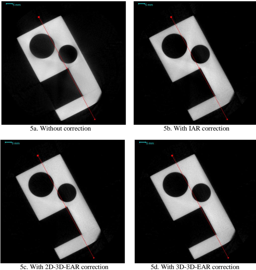
Figure 5. Comparison of three different artefact correction methods with an uncorrected slice of an aluminum test phantom (top left). At top right, the traditional Iterative Artefact Reduction (IAR), at bottom left, the proposed corrections with the 2D-3D-EAR respectively the 3D-3D-EAR (bottom right).
