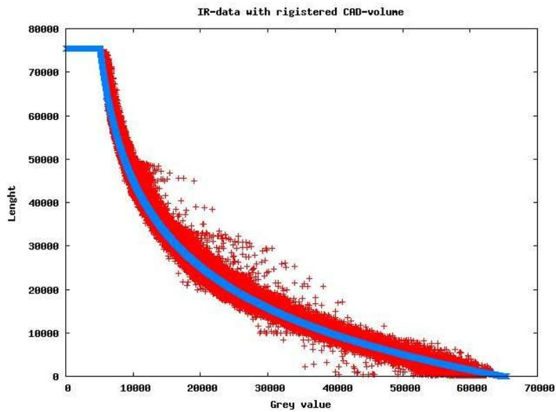
Figure 3. IR-point cloud with path lengths from 2D-3D registered CAD model.
