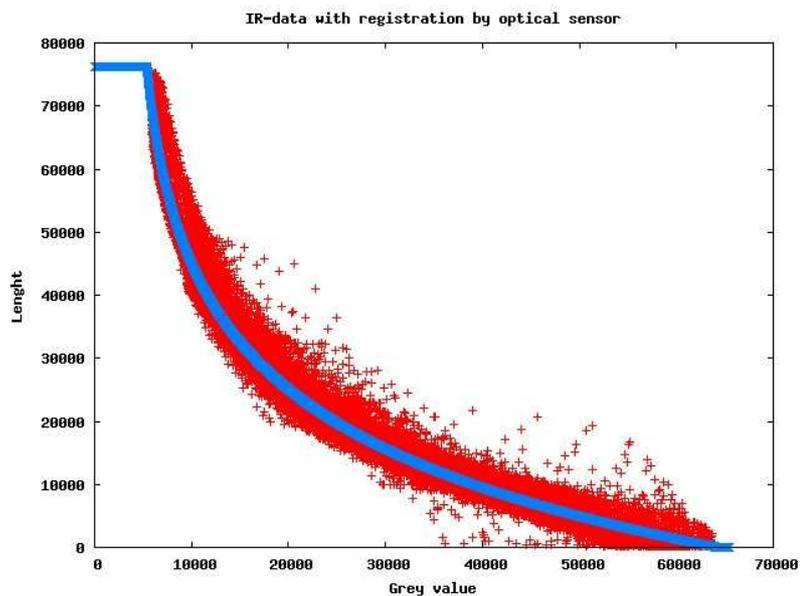
Figure 4. IR-point cloud with path lengths from 3D-3D registered CAD model.
