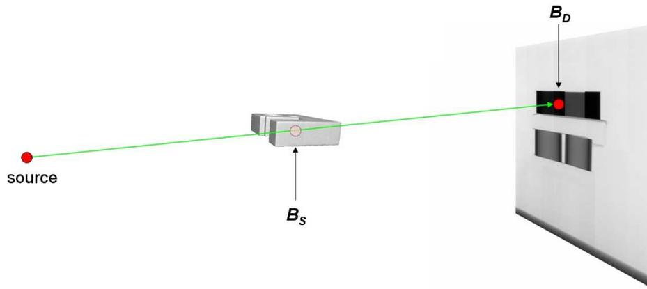
Figure 1. The barycentric line connects the source with the barycentre of the detector  $B_D$ , with respect to the measured intensities. The barycentre  $B_S$  of the object lies approximately on this line.
