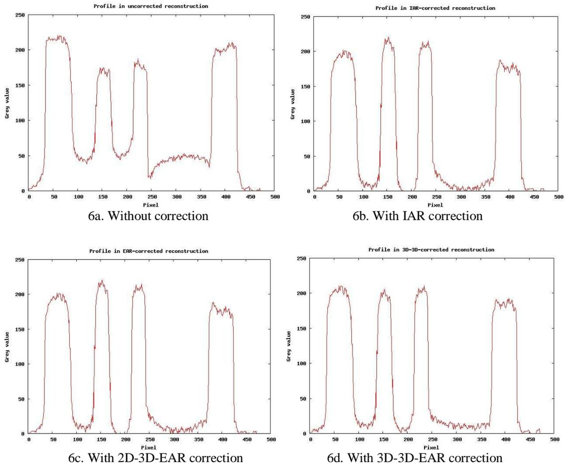
Figure 6. Profiles along the red lines in the cross sections of figure 5. The difference between the corrected profiles is negligible.
