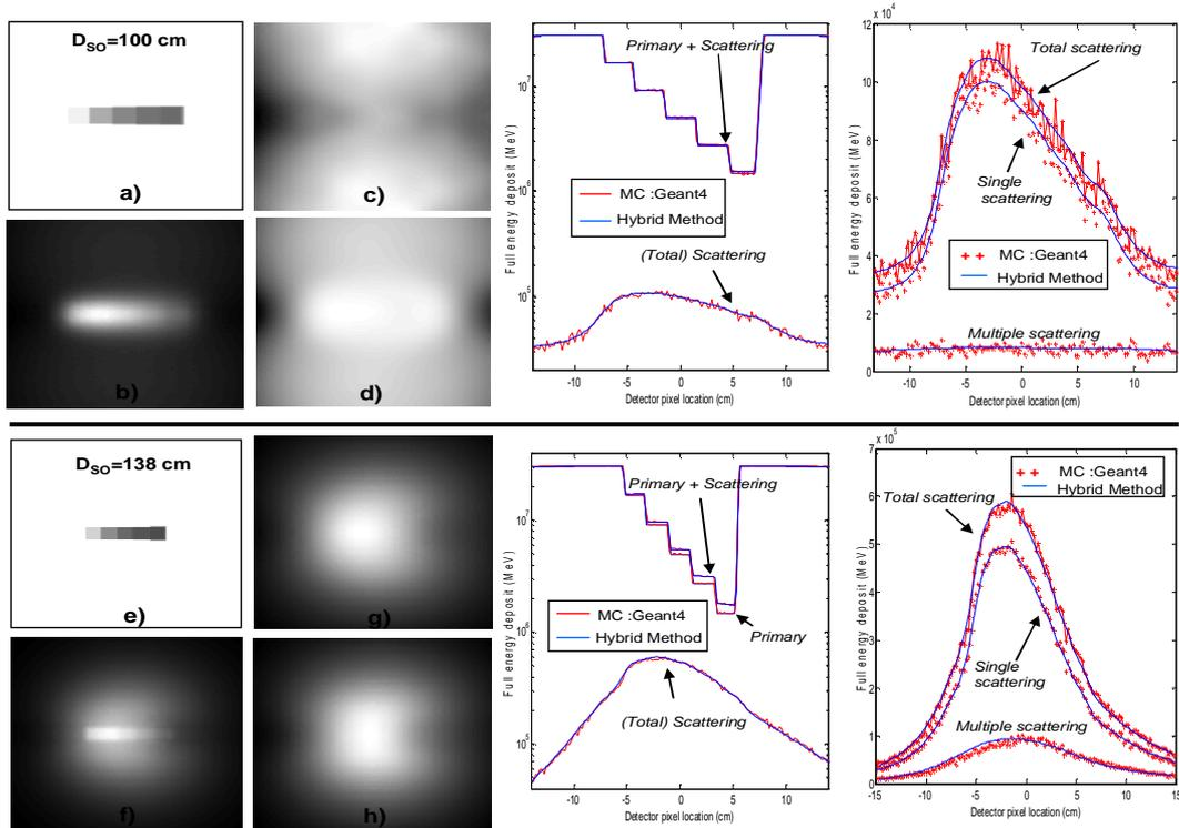
Figure 4 : Projection of object B at  $D_{SO}=100$  cm (above the bold line) and at  $D_{SO}=138$  cm (below the line). Details of primary (a,e), single scattering (b,f), multiple scattering respectively obtained with Geant4 (c,g) and with the hybrid method (d,h). Profile along the central horizontal line is plotted. detail of the decomposition of the scattering into single and multiple scattering is also shown.
