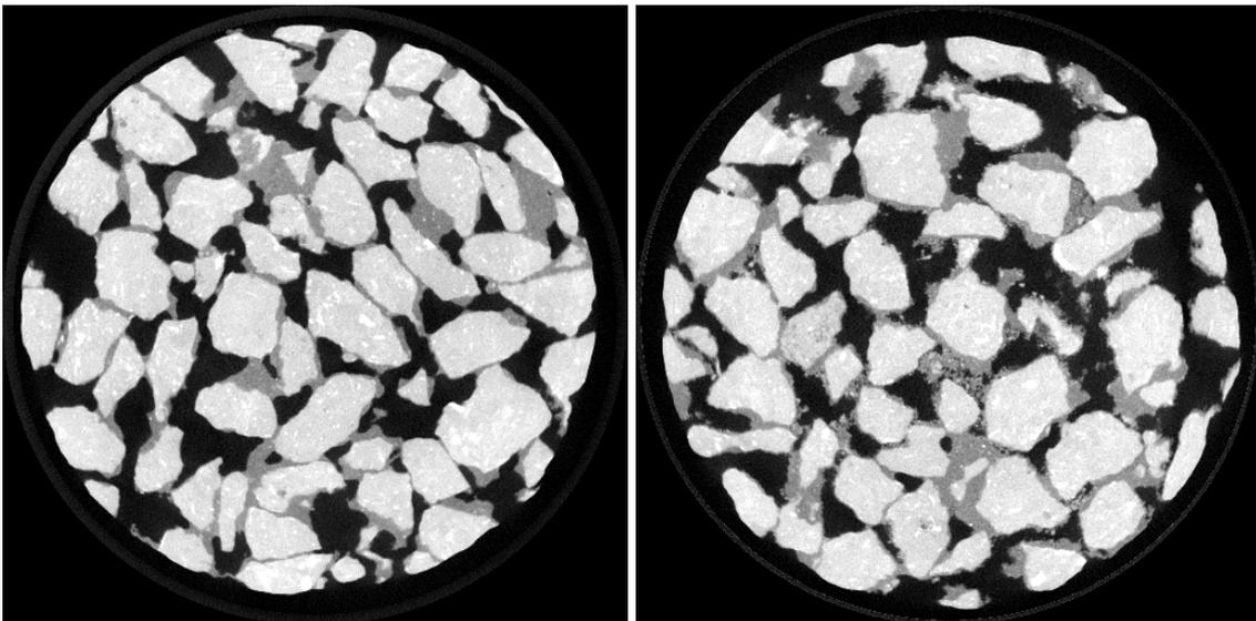
Fig. 3: Two slices of the 3D-data set of two core samples ( $\varnothing$  = 50 mm, height = 40 mm). The sample at right was contaminated with artificial dust.
