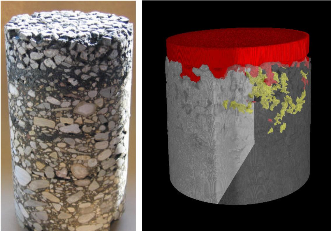
Fig. 9: Core sample (left image) and visualisation of closed porosity (right image).
