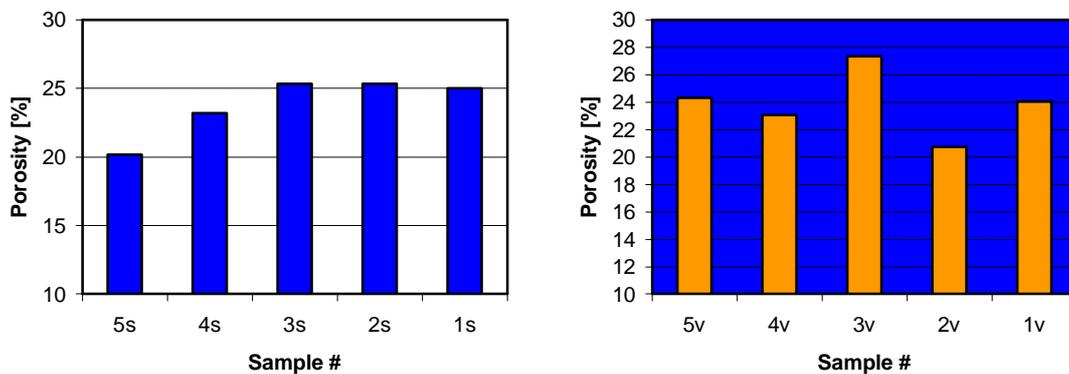
Fig. 7: Porosity of five core samples ( $\varnothing=50\text{mm}$ , height=40 mm), which are cut from two plates with water jet cutting. On of the plate (samples 'v') was artificially contaminated with dust.
