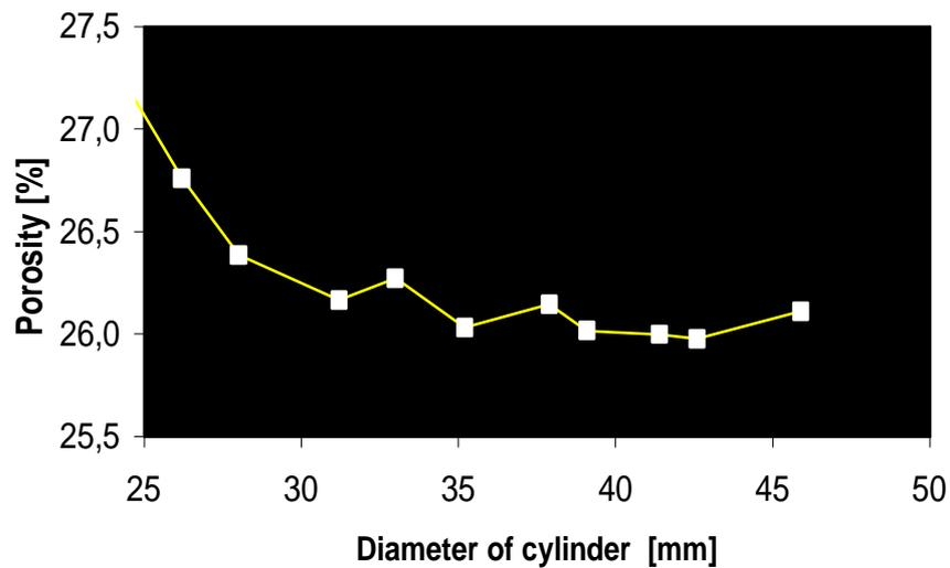
Fig. 6: Dependence of porosity from the elected sample volume.
