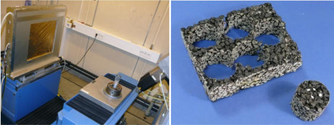
Fig. 1: High resolution tomograph with 225 kV micro focal X-ray tube and a temperature stabilized flat panel detector.
