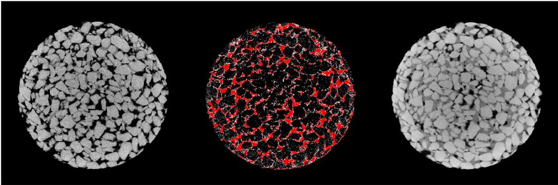
Fig. 10: Difference image (middle image) of an untreated sample (left image) and subsequent artificially infiltrated with dust (right image).
