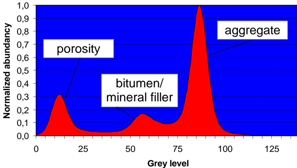
Fig. 4: Histogram of a core sample with the three components porosity, bitumen/mineral filler and aggregates.
