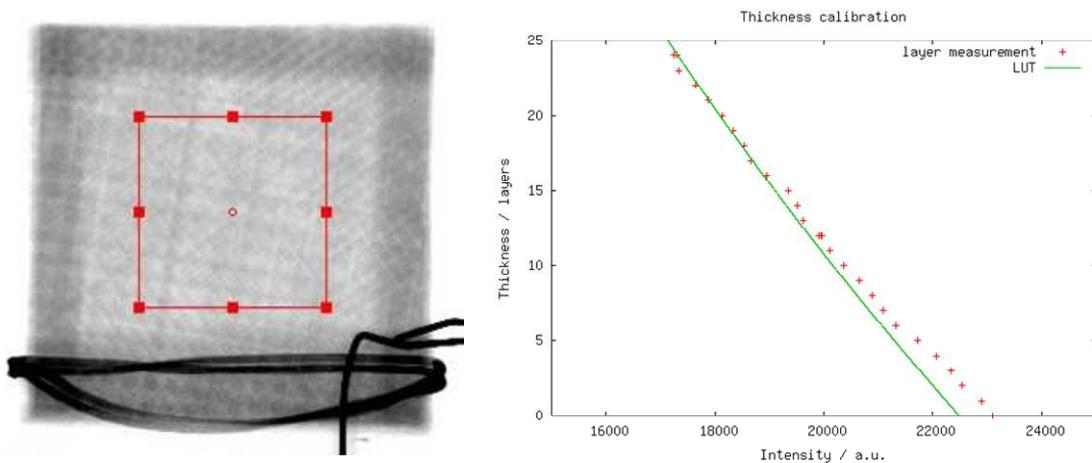
**Figure 7: Projection image of eight layers of perform patches, used for material calibration (left), measured intensities and fitted model curve (right).**
