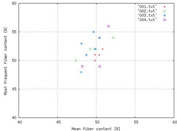
**Figure 5: Distribution of the mean fiber content and the most frequent fiber content values of the 19 preform samples.**
