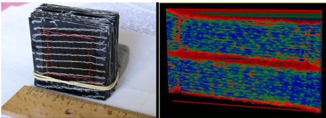
**Figure 6: Several preform patches bound to one block (left) and a cut through the three-dimensional color coded volume (right).**
