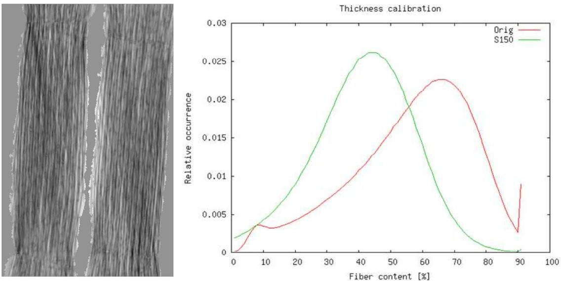
**Figure 9: Influence of limited angle projection data. The left image shows a slice of the difference volume, which is calculated between the original and the limited angle volume. The right diagram shows the computed fiber content of the original and the limited angle volume.**
