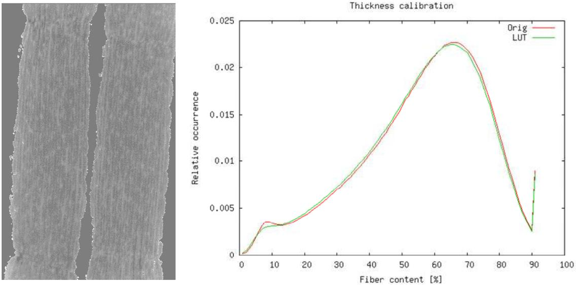
**Figure 8: Effect of the material calibration. The difference is shown in the left image. The right image shows the distribution of the fiber content in the original and the calibrated data.**
