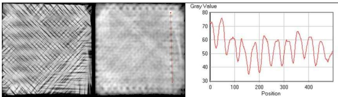
**Figure 4: Slice of a preform (left), the filtered slice (center) and the gray value profile of the line in the filtered slice (right)**
