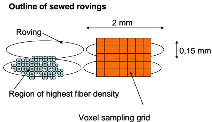
Figure 2: Outline of the voxel sampling of the fiber rovings.
