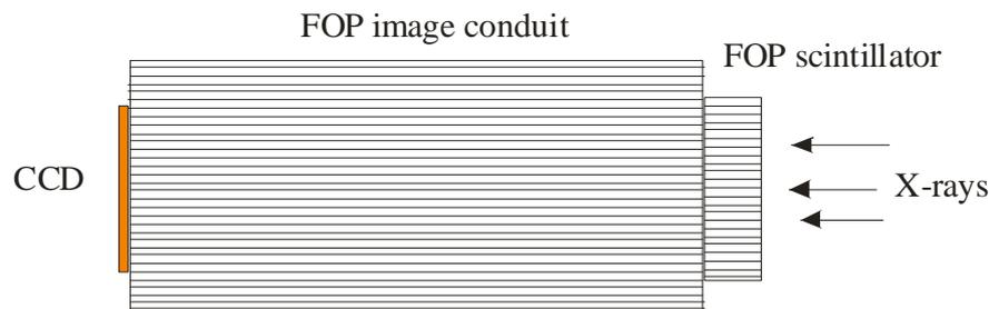
Figure 1. First generation fiber optic x-ray camera.
