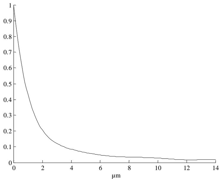
Figure 4. Energy deposition vs. radial distance.
