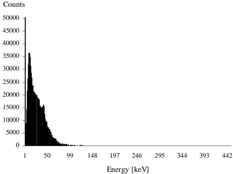
Figure 5. Pulse height spectrum for an 11 micron fiber.
