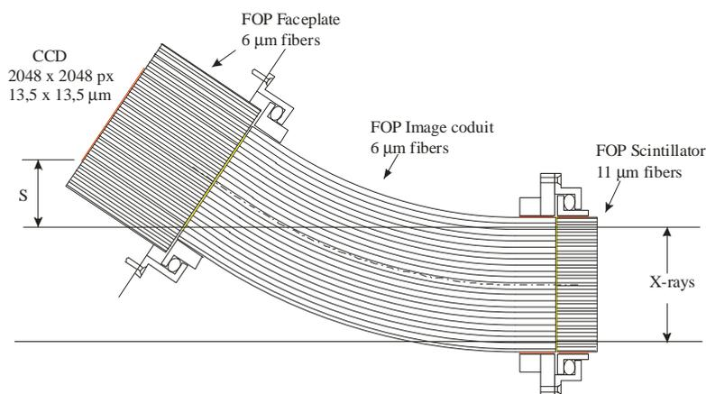
Figure 9. New concept with a bent fiber optic image conduit.
