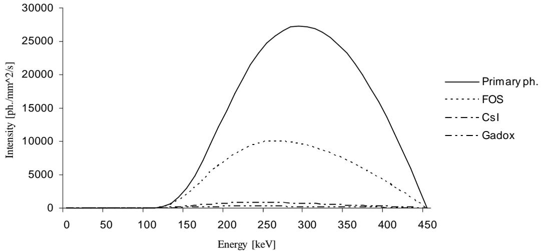
Figure 7. Filtered spectrum and attenuated radiation.
