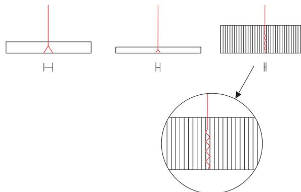
Figure 6. Conventional phosphors compared to fiber optic scintillators.
