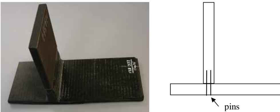
Figure 2: T-shaped CFRP composite assembled with pins.
