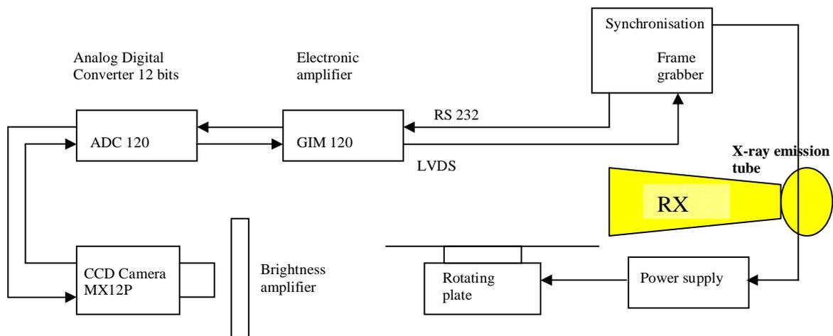
Figure 3: Scheme of the X-ray tomograph.
