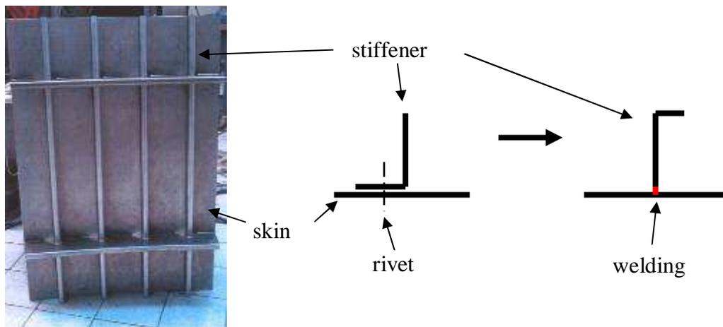
Figure 1: Metallic structure with riveted or welded stiffener.
