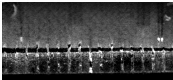
Figure 11: 2D view along the sewing sequence in the stiffener and base plate. White areas correspond to presence of darkening agent.
