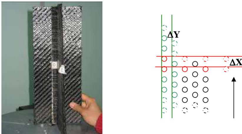
Figure 4: View of a T-shape CFRP preform and nailing sequence.
