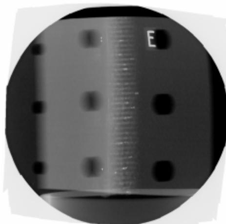
Figure 9: Digital radioscopy of a T-sewed CFRP composite showing defects after mechanical constraints.
