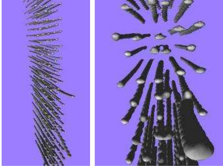
Figure 6: 3D reconstruction of titanium nails. CFRP composite is virtually removed.
