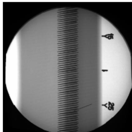
Figure 5: Digital X-ray radiography showing the alignment of titanium nails in the CFRP part.
