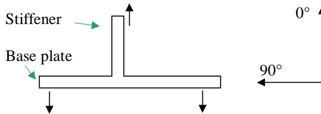
Figure 8: Mechanical constraint to pull-out the stiffener from the base plate.
