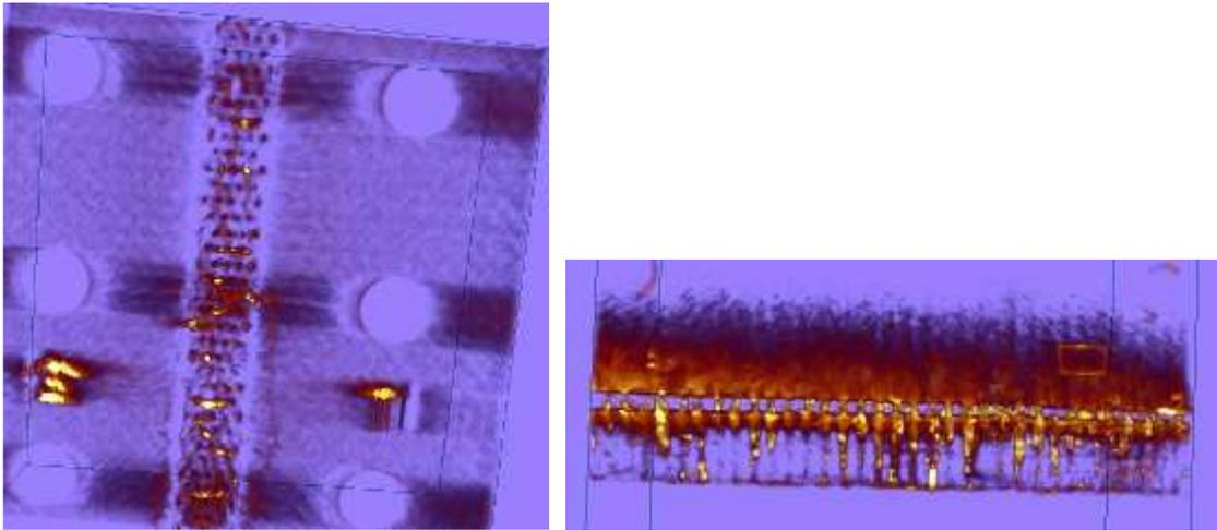
Figure 10: 3D view of stiffener and base plate showing cracks and wire defects. Yellow corresponds to strong attenuation.
