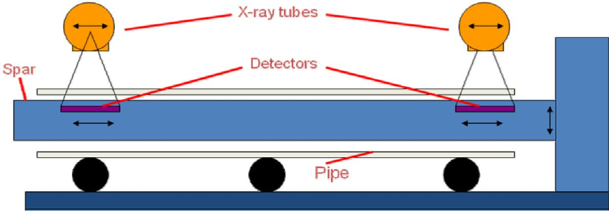
Figure 1: Layout of X-ray arrangement
