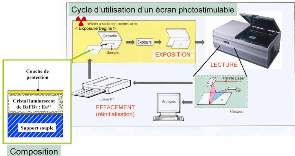
Figure 3 : Principles of reading of a phosphor plate by a scanner
