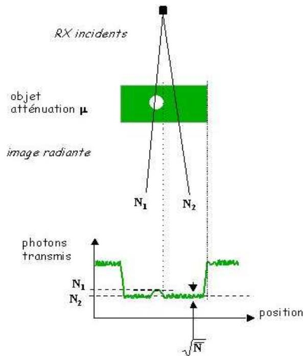
Figure 8 : Defect detection in an image.
