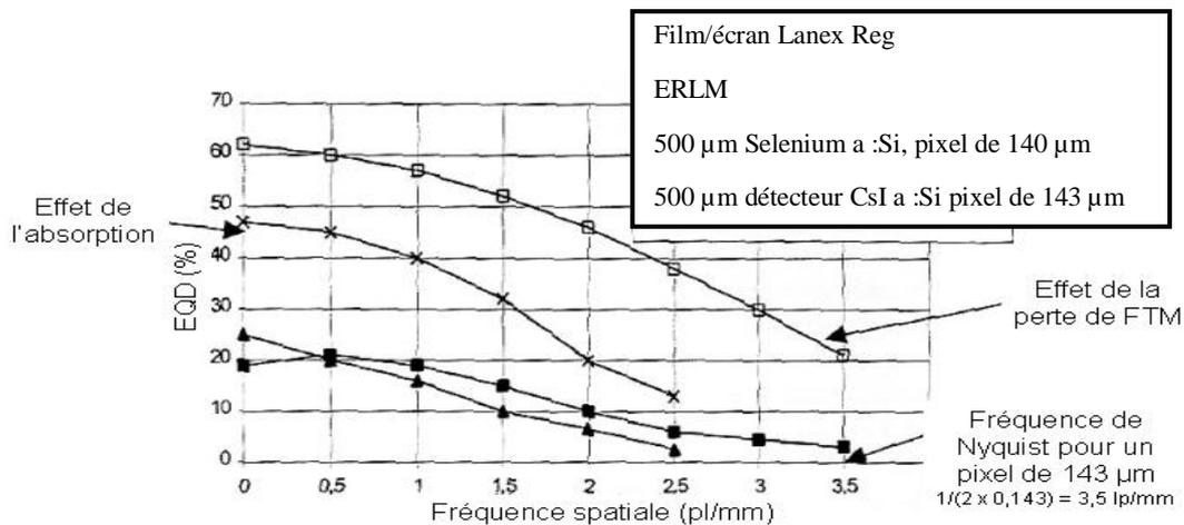
Figure 9 : Quantum Detection Efficiency of different sensors in the same spectrum (70 kV, 21mm Al filter) and dose (2,5 μGy) conditions.
