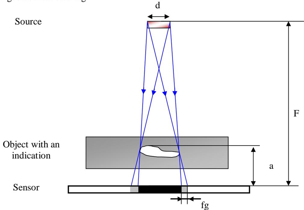
Figure 4 : Radiography acquisition geometry
