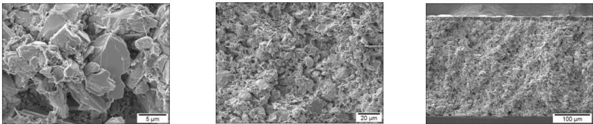
The improved sharpness of the HR imaging plate comes from smaller phosphor particles and a thinner layer.
