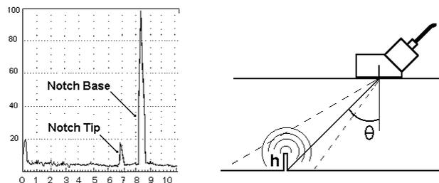
Figure 13: Back diffraction – left, A-scan presentation, right ultrasonic set-up.
