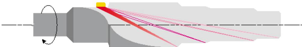
Figure 3: Schematic showing sectorial scanning used on turbine rotor.
