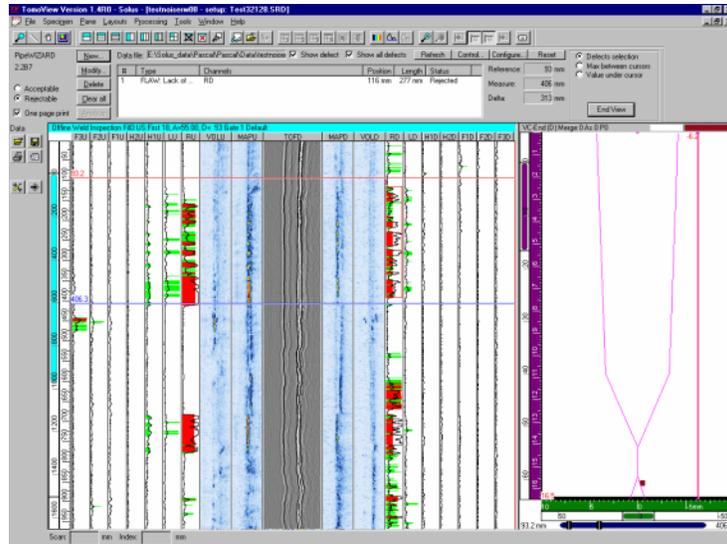
Figure 10: Standard ASTM strip chart display with additional B-scan for interpretation.
