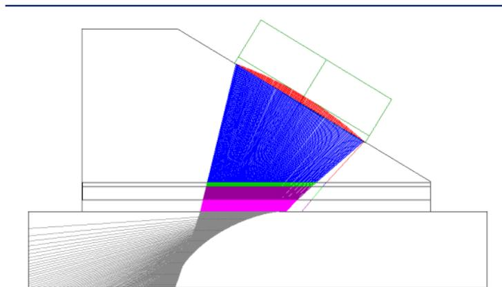
Figure 6: Imagine3D modeling of phased array and wedge on pipe, with temperature gradient in layers from base.
