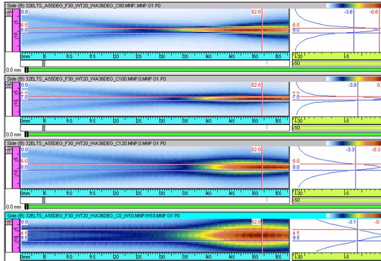
Fig. 15: Modeled Fill 1 channel beam profiles. The red cursors represent the theoretical focal position. The probe is at the left. Curvatures (top to bottom) = 80mm, 100mm, 120mm and infinite (the bottom image is the standard unfocused AUT probe).
