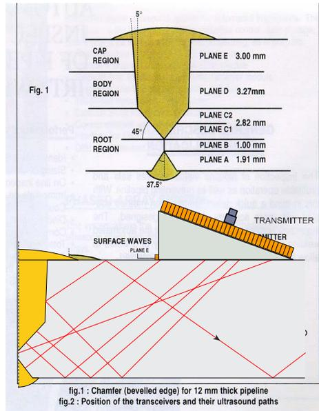
Figure 4: Schematic showing zones on a CRC-Evans weld profile, and ultrasonic beams from a phased array probe.
