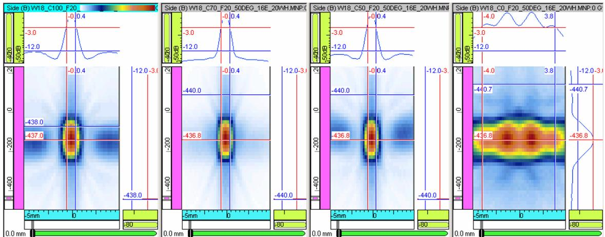
Figure 14: Modeled beam profiles for focused and unfocused arrays. Flat (unfocused) array is at right; 1.5D arrays are left three images.
