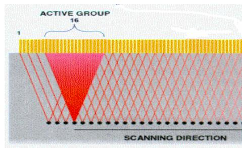
Figure 2: Schematic illustration of electronic (linear) scanning.
