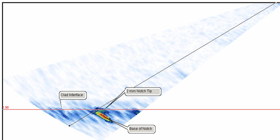
Figure 11: Clad plate inspection clockwise using S-scan, showing notch base, notch tip and clad interface.
