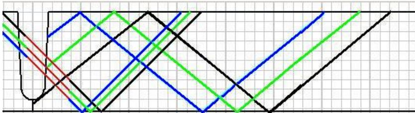
Figure 5: Ray tracing showing beams for nominal, minimum and maximum wall thicknesses, and errors.
