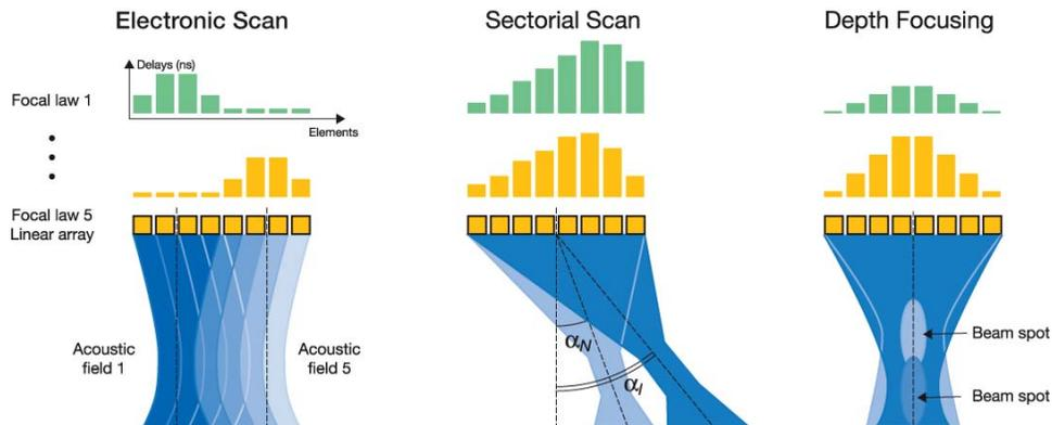
Figure 1: Schematic showing generation of linear and sectorial scans using phased arrays.
