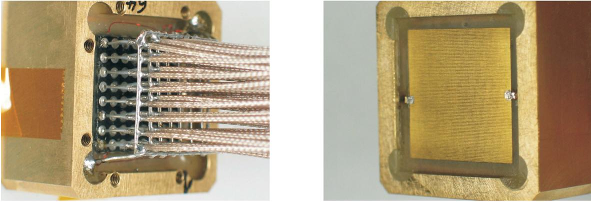
**Figure 7.** 8 by 8 matrix array for lower frequency applications during fabrication. The cabling to supply the 64 elements is clearly visible.
