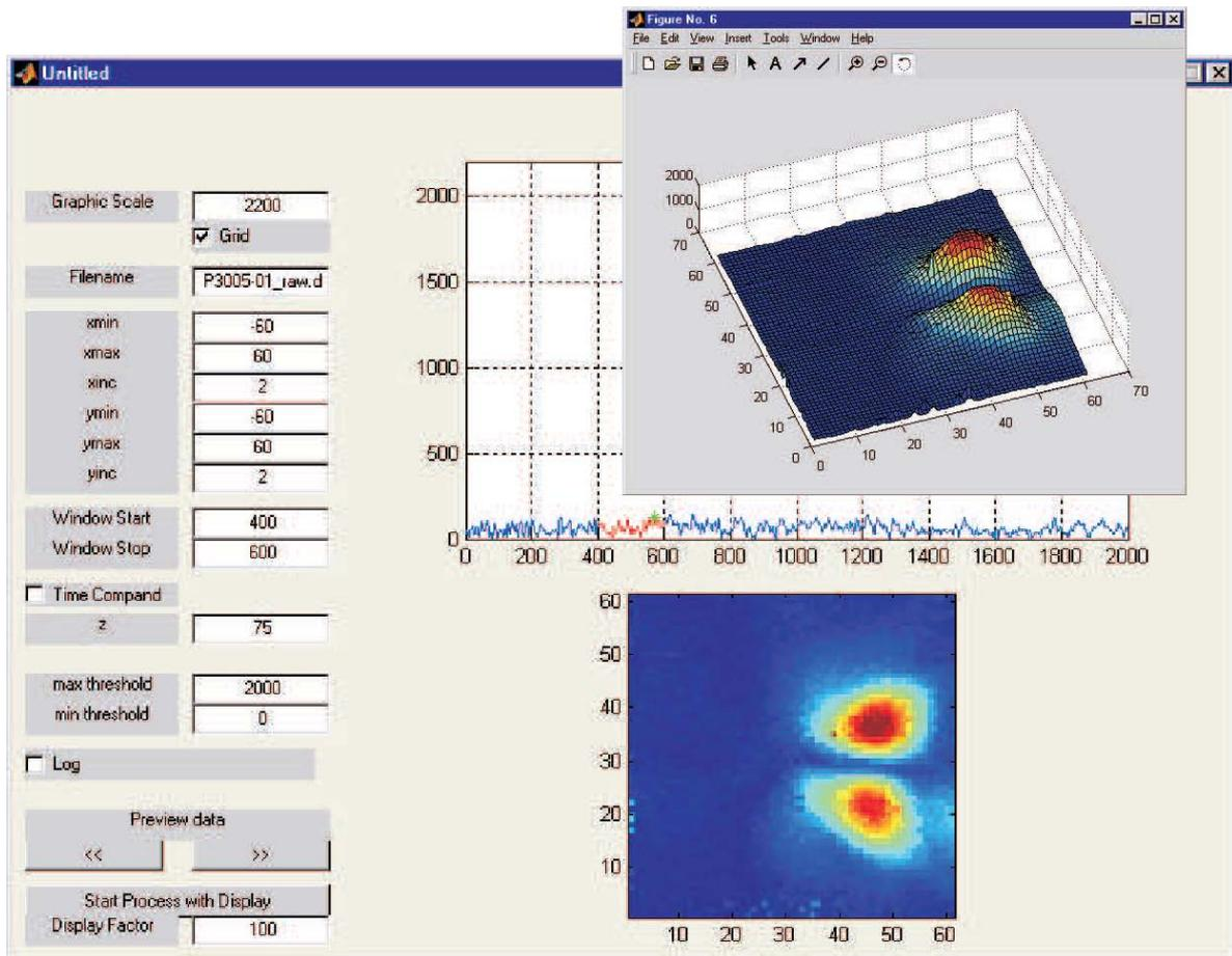
**Figure 8.** C-scan obtained by scanning two side-drilled holes with cone-like tips (note: the indicated scaling does not correspond to mm). An excerpt of MatLab-environment which allows for a user-friendly handling is also shown.
