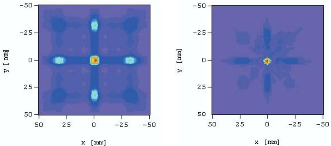
**Figure 4.** Simulated (left) and experimental (right) C-scan for the case of on-axis focusing to a depth of 108 mm, receiver depth 108 mm (one sixth of the near-field length).
