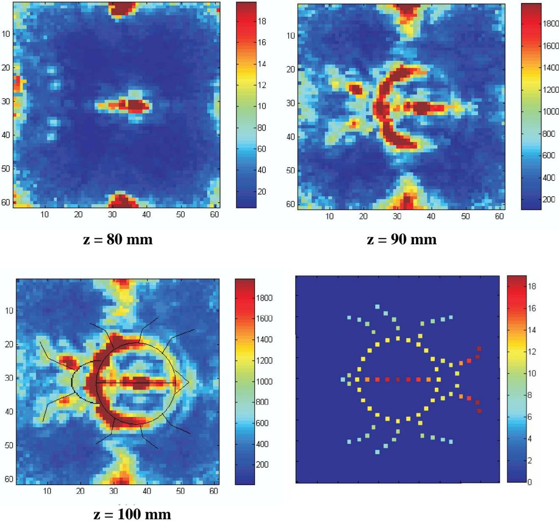
**Figure 6.** Lower right: spider pattern and depth of the flat-bottomed holes, other: C-scans obtained for different focusing depths  $z$  as indicated.
