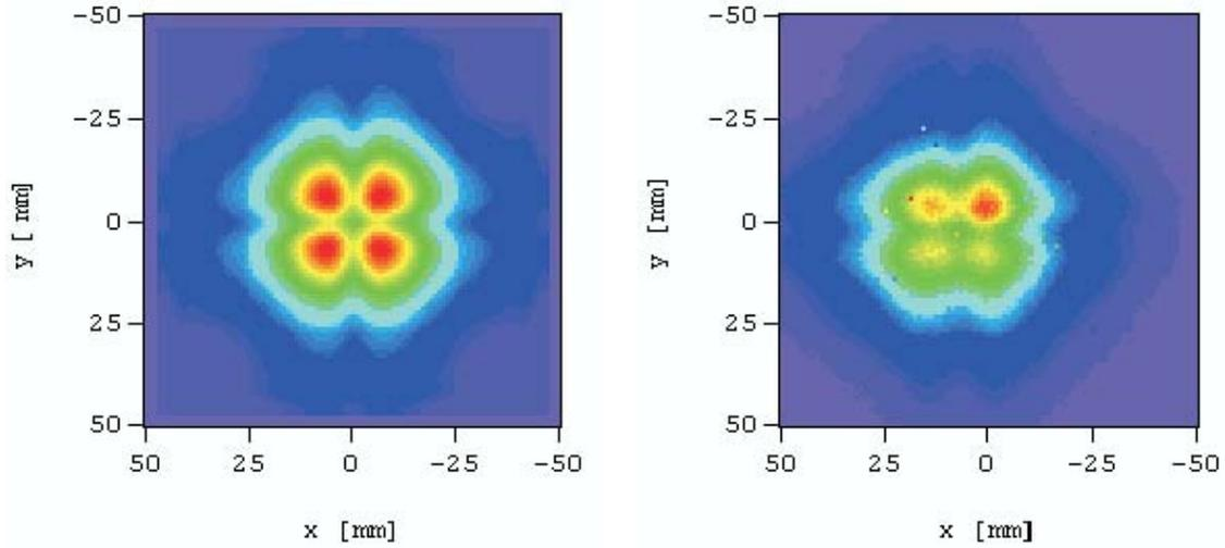
**Figure 3.** Simulated (left) and experimental (right) C-scan for the case of unfocused, perpendicular transmission, receiver depth 325 mm (half of the near-field length).
