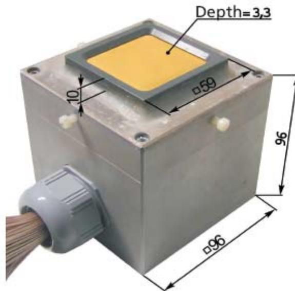
Figure 1. Matrix array sensor with its dimensions.
