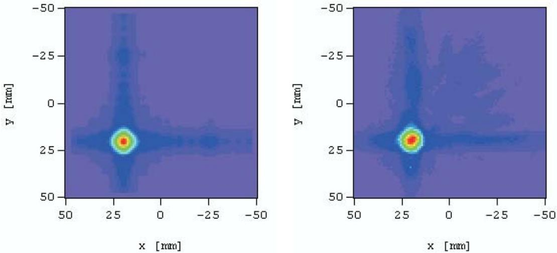
**Figure 5.** Simulated (left) and experimental (right) C-scan for the case of off-axis focusing to a depth of 323 mm, receiver depth 323 mm (one sixth of the near-field length).
