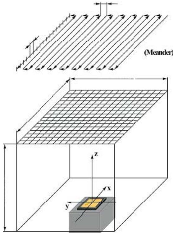
**Figure 2.** Experimental set-up and scanning scheme used to perform the beam field measurements.
