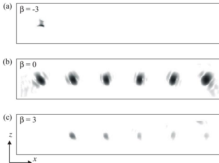
Fig. 5. TFM images tuned using specularity parameter: (a) tuned to highlight non-specular reflectors; (b) untuned; (c) tuned to highlight specular reflectors.
