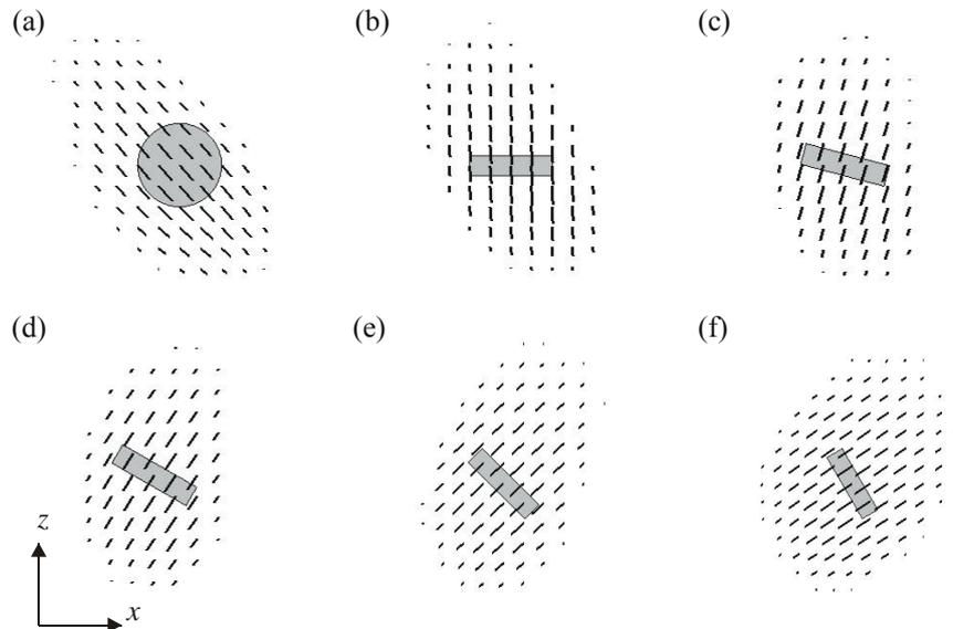
Fig. 4. Detail of VTFM vector field images of reflector orientation from the six reflectors in the aluminium sample: (a)  $\text{\O}1$  mm hole; (b) slot at  $0^\circ$ ; (c) slot at  $15^\circ$ ; (d) slot at  $30^\circ$ ; (e) slot at  $45^\circ$ ; (f) slot at  $60^\circ$ .
