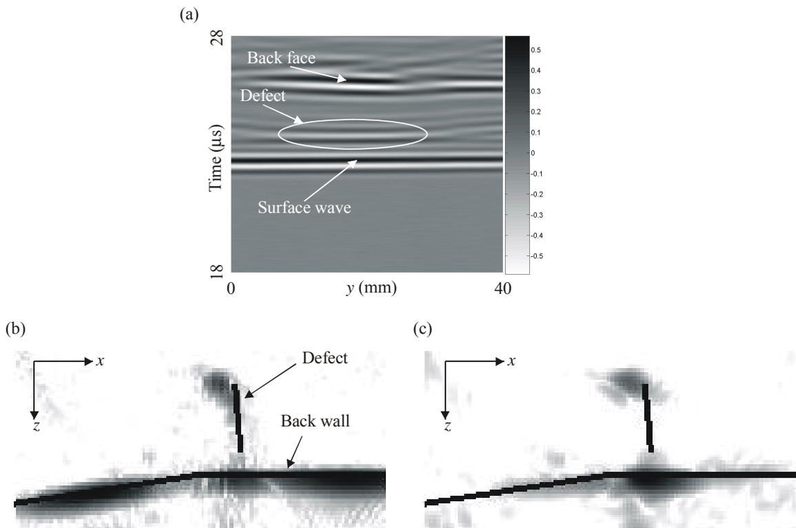
Fig. 6. (a) TOFD image from defect in stainless steel sample and DTFM images from the same defect: (b) using all elements in both arrays; (c) using the elements in one array to transmit and elements in the second array to receive.
