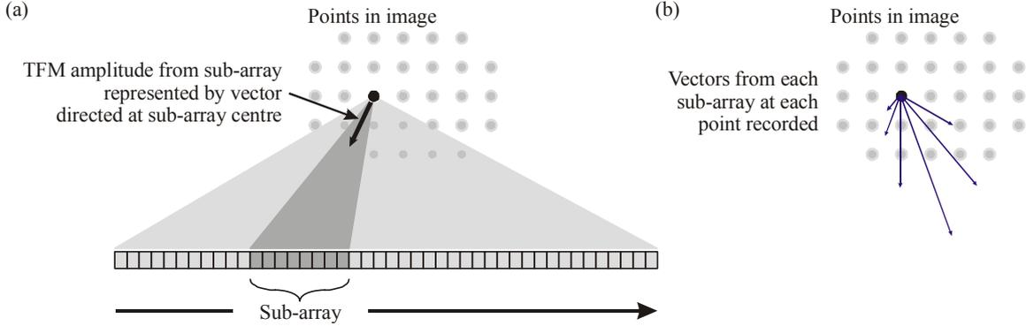
Fig. 1. Schematic diagrams indicating the operation of the basic VTfM algorithm showing (a) the vector generated from one sub-array aperture at a point in the image and (b) the vectors from a number of sub-array apertures at one point.
