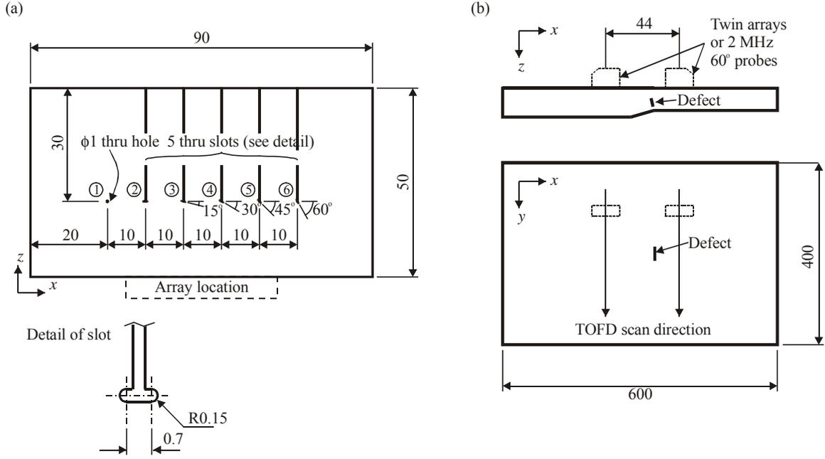
Fig. 2. Samples used: (a) aluminium block containing wire EDM slots at various angles; (b) stainless steel specimen containing simulated weld defects.
