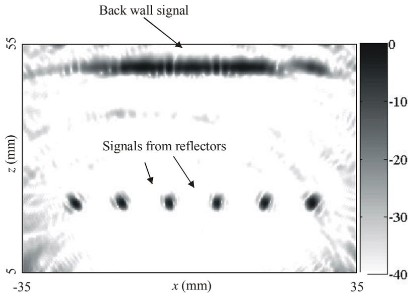
Fig. 3. TFM image obtained from aluminium sample. The greyscale is in dB relative to the largest reflector which is the back wall of the sample.
