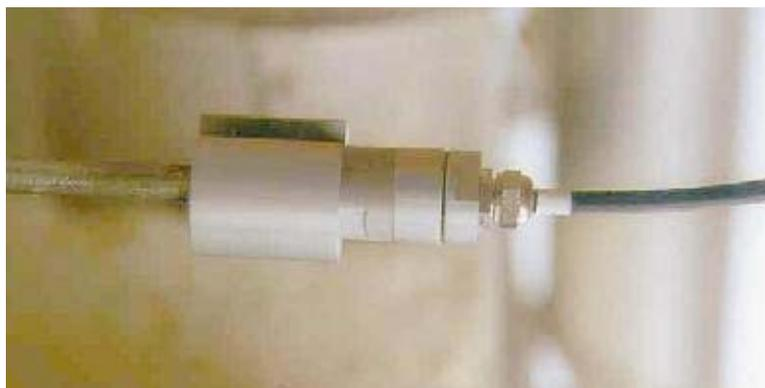
During in-service inspections, the sensors are placed at the end of the wave guide; they then receive the acoustic waves propagated from the surface of the equipment rather than being condemned with the tank in the slope and thus to be exposed to possible damage risks. [Figure 5]
