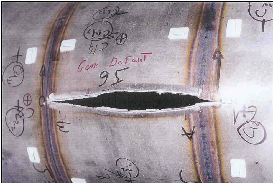
**Figure 2:** Opening of a weak area during the burst test of a mini structure
