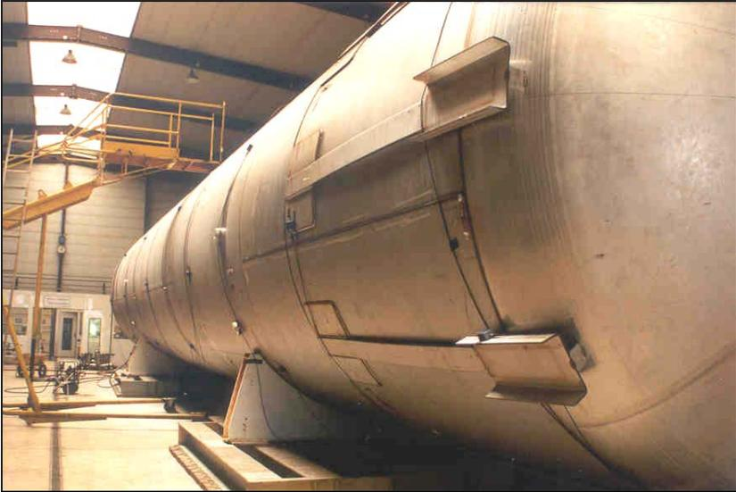
**Figure 3:** Acoustic emission monitoring of the workshop final testing of pressure vessel
