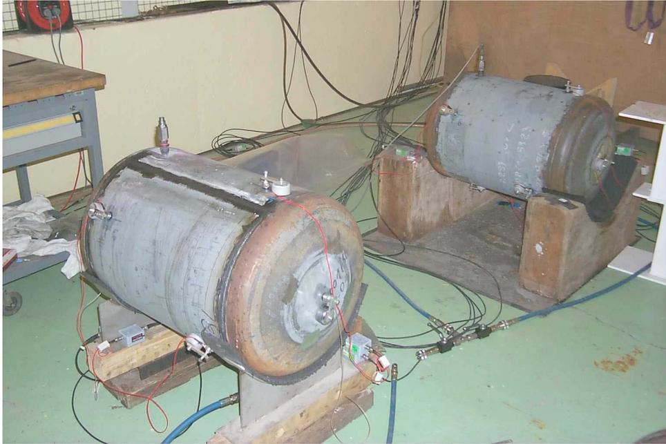
**Figure 1:** mini structures including artificial defects that were tested
