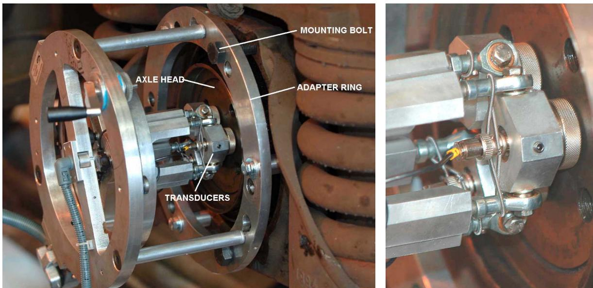
**Figure 4:** General view of transducer-holder tool mounted on an axle during inspection (left) and detail of articulated transducer holders (right).
