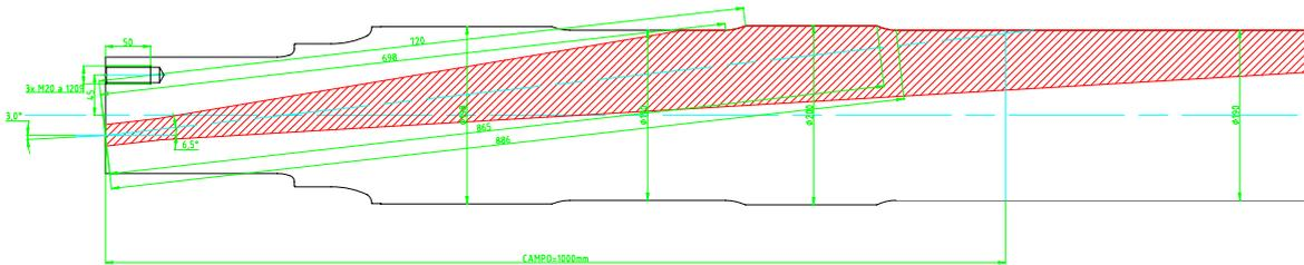
**Figure 1.b:** Specific inspection of reduction gear seat and fillet to body of axle,  $6.6^\circ$  incidence angle.
