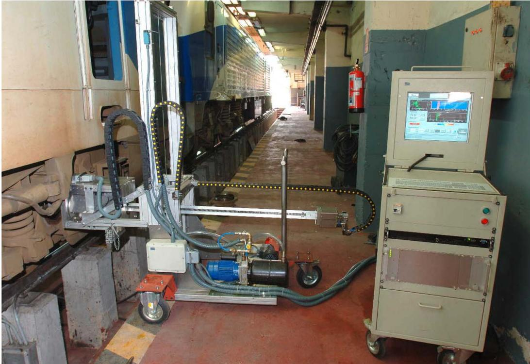
**Figure 6:** General view of the hollow axle inspection system, with the mechanical subassembly (left) mounted to an axle under inspection. The control unit can be seen to the right.
