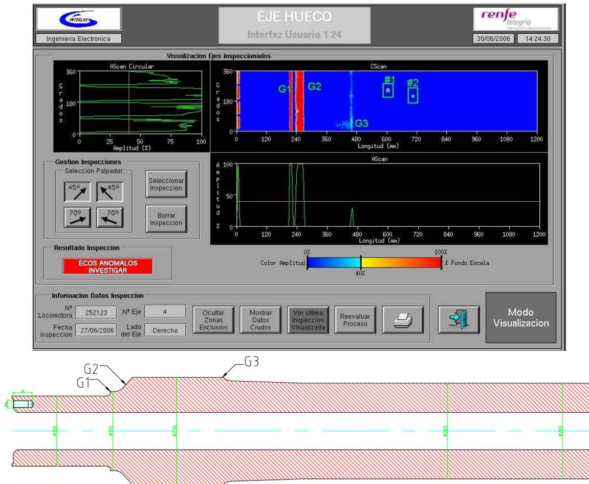
**Figure 9:** Inspection results for type 252 reference axle (above), and diagram of the same axle, showing the geometric features producing echoes (below).
