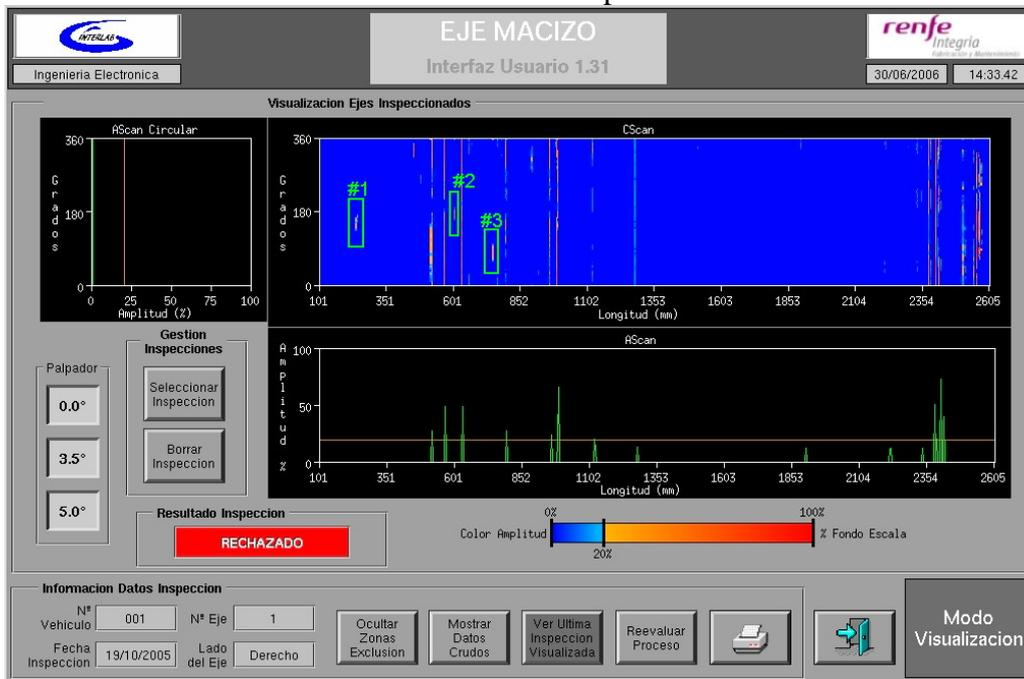
**Figure 7:** Inspection results for the solid axle inspection system with three artificial cracks
