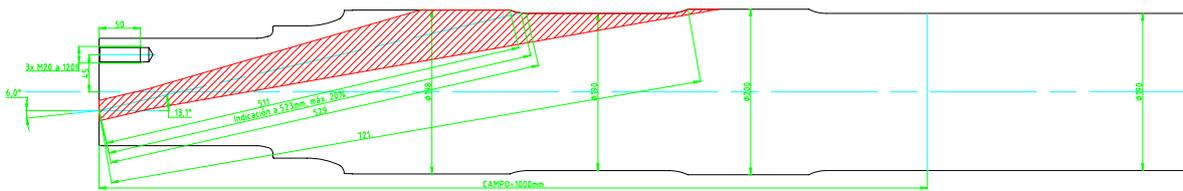
**Figure 1.c:** Specific inspection of wheel seat to body of axle fillet,  $13.3^\circ$  incidence angle.
