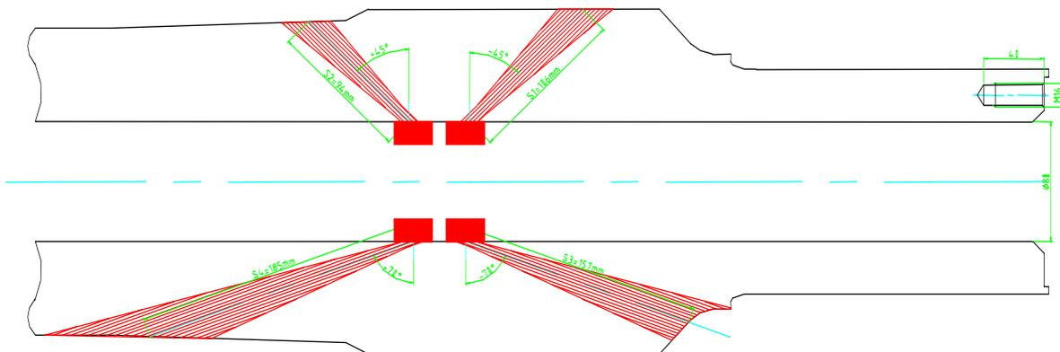
**Figure 2:** Inspection of hollow axles from the bore inner surface, using  $\pm 45^\circ$  and  $\pm 70^\circ$  angles of incidence.
