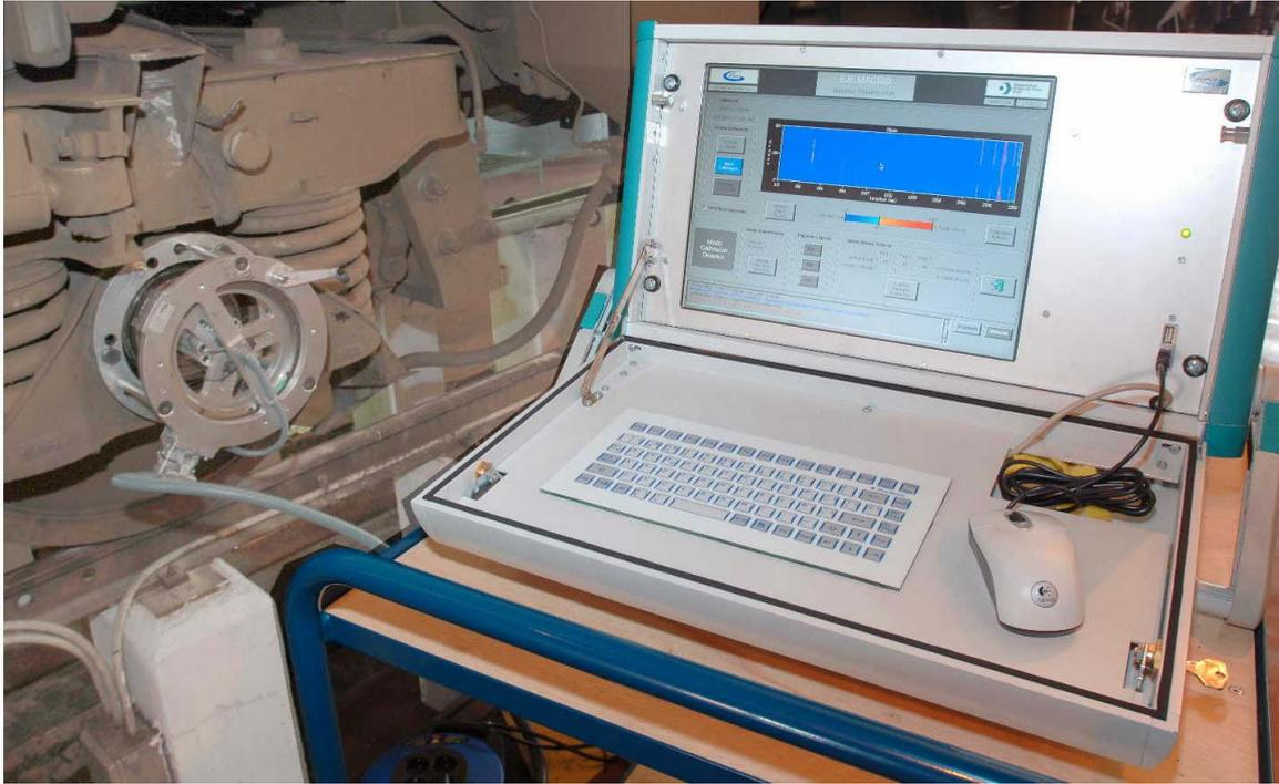
**Figure 3:** Overview of solid axle inspection system, including control unit (foreground, right) and transducer-holder tool mounted on an axle during inspection (background, left).
