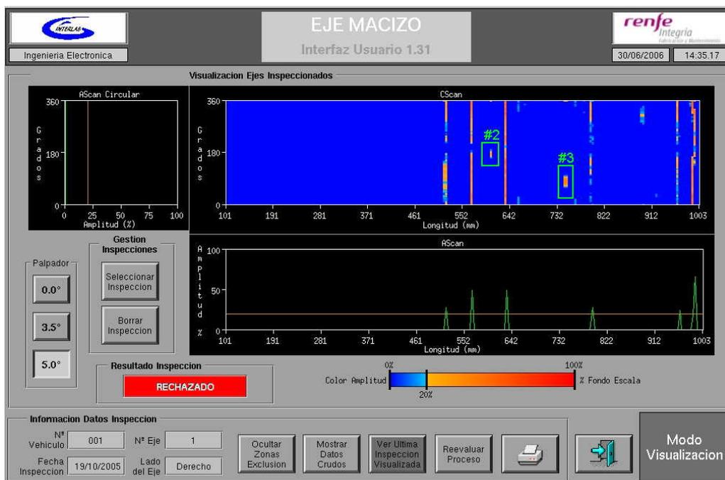
**Figure 8:** Detail of inspection results for the reduction gear seat in a 269.200 solid axle with a 5° wedge.
