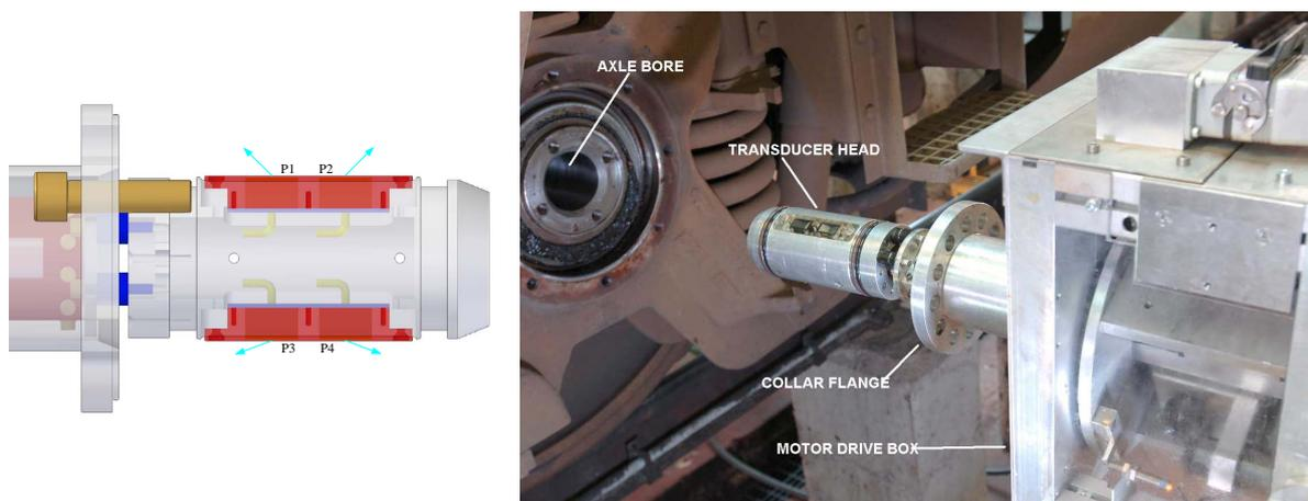
**Figure 5:** Design of four transducer head tool (left) and actual view of transducer head and collar flange for attachment to axle head (right).
