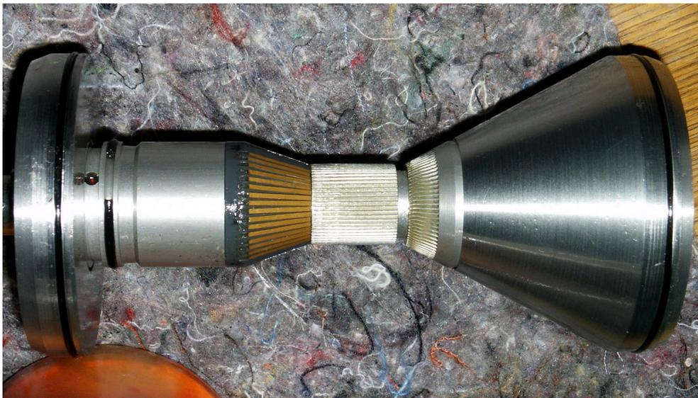
**Fig 6** conical rotation scanner phased array probe adapted for bore hole  $\varnothing$  70mm
