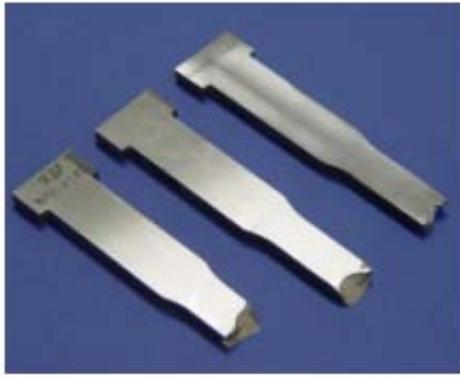
**Figure 2:** Ti-17 Fatigue samples
