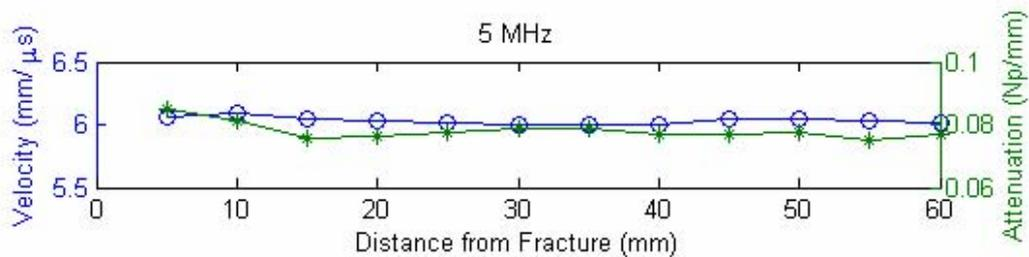
**Figure 4:** Sensitivity in relative  $\beta$  correlated with distance from fracture. Conventional ultrasound properties (Velocity, Attenuation) showing negligible change
