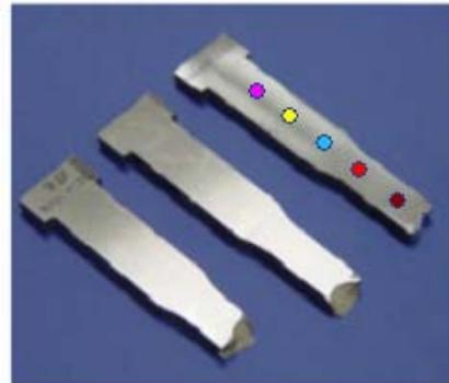
**Figure 3:** Variation in nonlinearity parameter  $\beta$  (slope) from grip section to the gage section.  $\beta$  sensitivity is indicated by the increase in slope from grip to gage section of the failed fatigue bar
