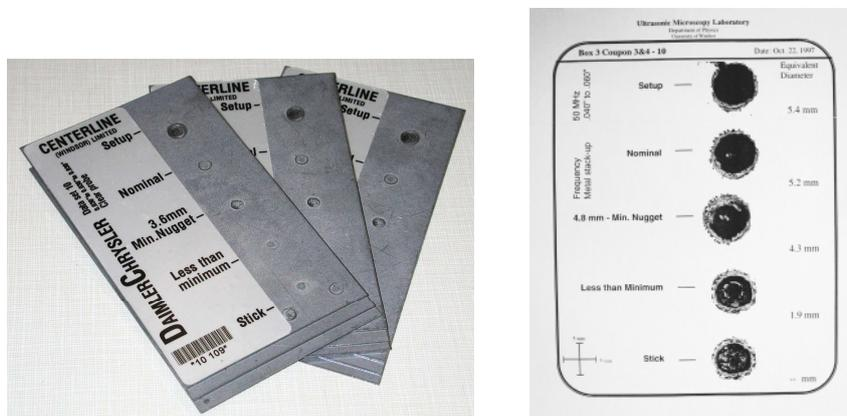
**Fig 6.** Certification of weld coupons
