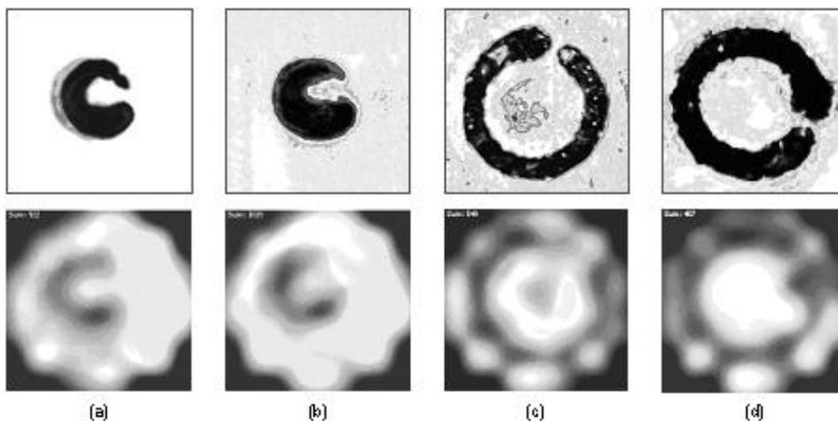
**Fig 3 -** Acoustic imaging inspection of laser spot welds with a desktop scanning acoustic microscope and corresponding images obtained with the 52-element array: (a), (b) 0.75 mm thick steel plate approximately 3.0 mm weld; (c), (d) 1.0 mm thick steel plate around 7.0 mm weld. Detectable imperfections: Insufficient length, Seam interruption, Lack of fusion, Pin hole existence.
