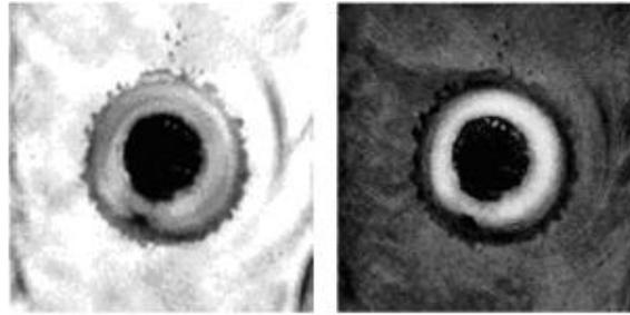
**Fig 2.** C-scans of spot weld, obtained on fundamental frequency (left) and on second harmonic (right). Size of scanned region is 12×12 mm.
