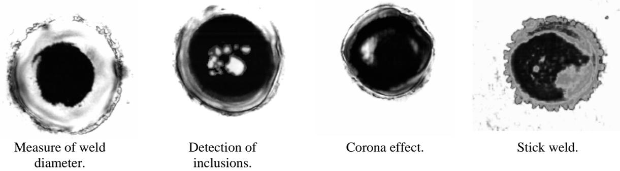
**Fig 5.** C-scan Images of the interface area (depth penetration 1 mm) from the spot welding.
