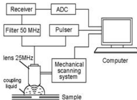
**Fig 1.** Schematic diagram of the scanning acoustical microscope as used for second harmonic imaging.
