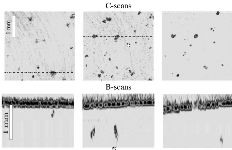
**Fig 4.** Acoustic images of various porosities in an aluminum casting.
