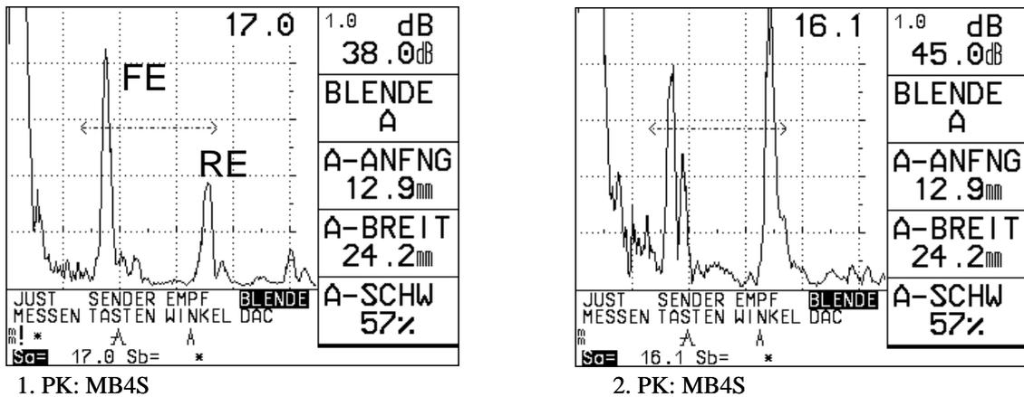
The difference in amplitude of probe no. 1 ( $\varnothing 3\text{mm}$ ) and no.2 ( $\varnothing 1\text{mm}$ ) is 7 dB
