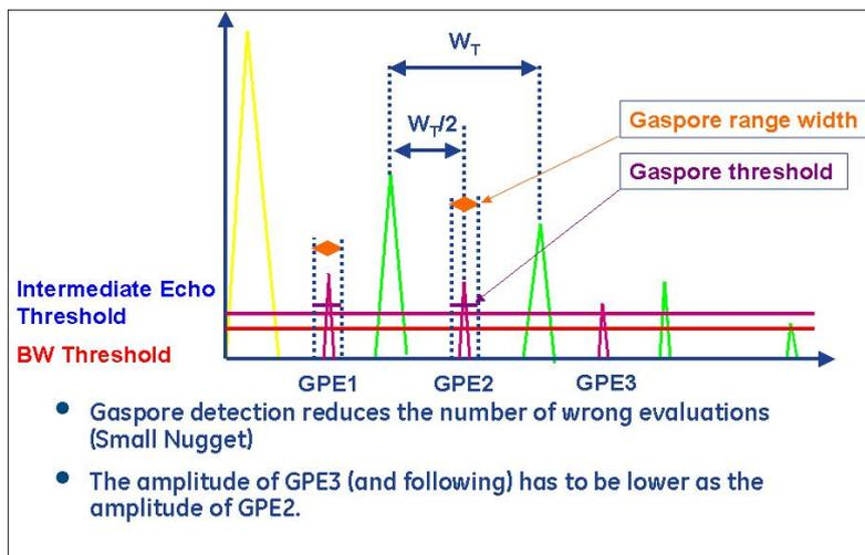
Figure 8. Gas Pore Identification
