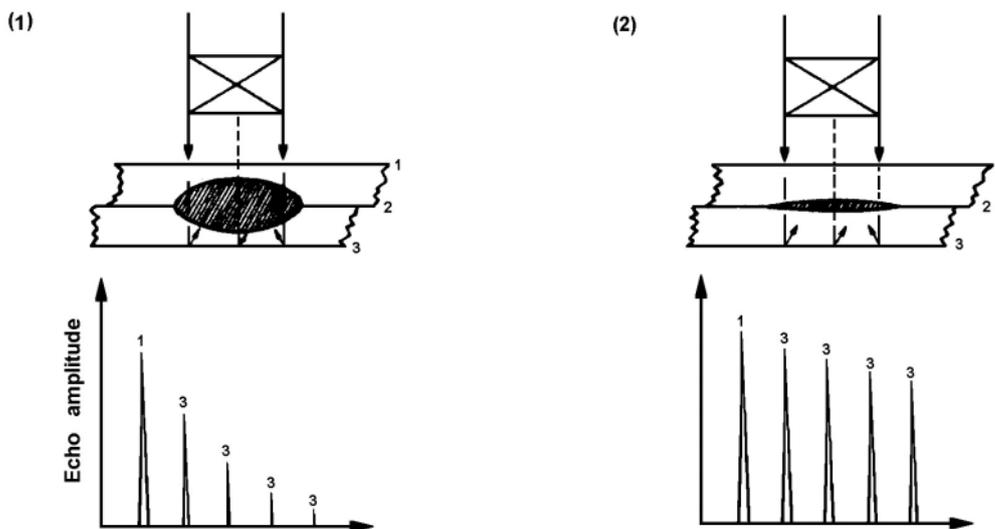
Figure 3. A-Scans showing different attenuation rates
