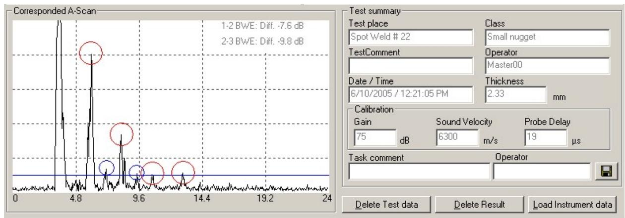
Figure 10. Example of intermediate echoes identified as undersize.
