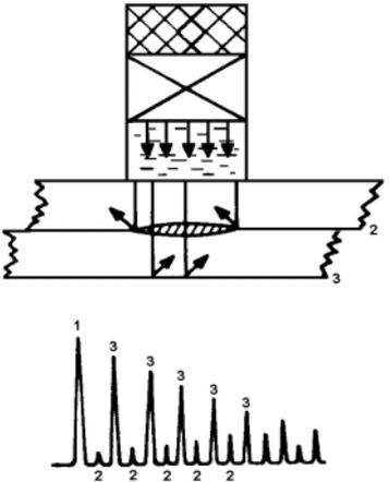
Figure 4. Undersize weld
