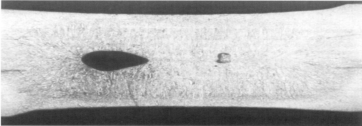
Figure 6. Micrograph of Gas Pore
