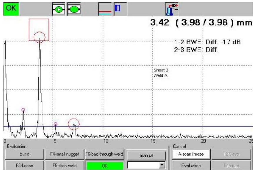
Figure 9. Gas pore detected. Evaluation OK.
