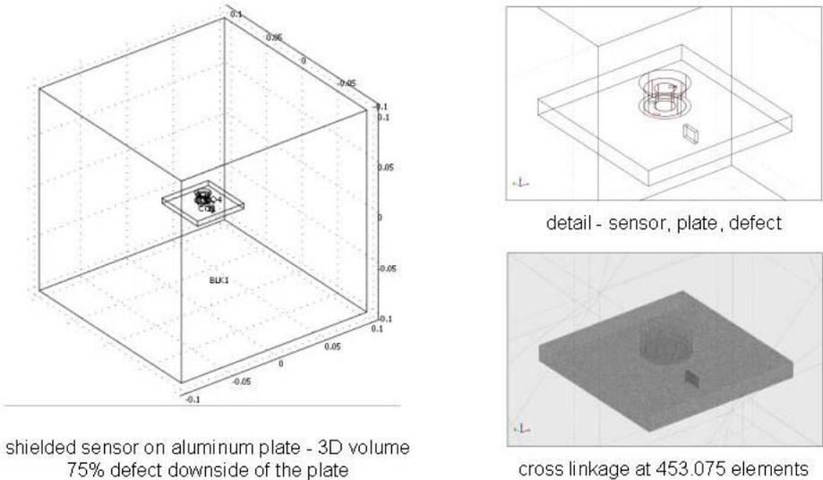
**Figure 7:** 3D model – simulation of eddy currents and magnetic fields
