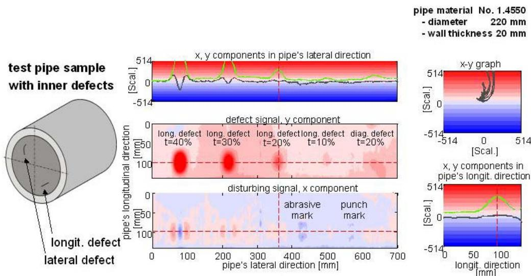
Figure 11: 2D signal analysis of longitudinal inner defects
