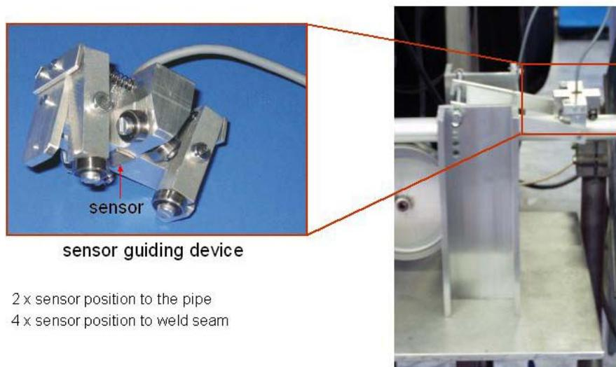
**Figure 13:** Process-integrated remote field eddy current testing
