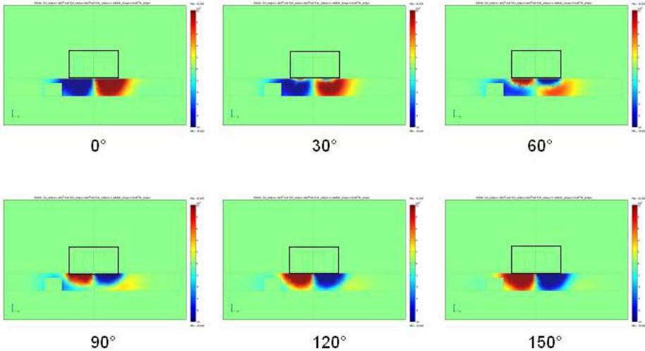
**Figure 8:** Simulation – eddy current distribution (x component)
