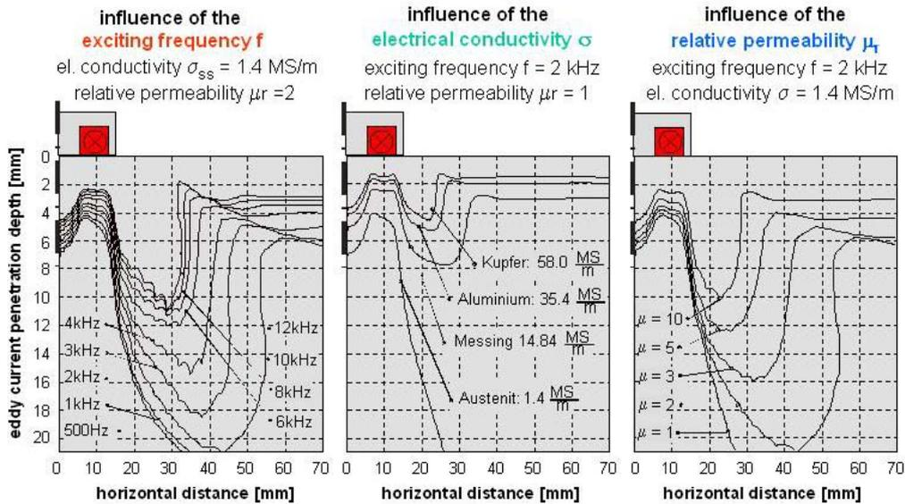
Figure 5: Penetration depth as function of test parameter variation
