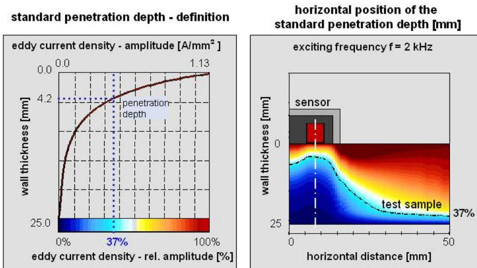
**Figure 4:** Standard penetration depth analyzes simulation results
