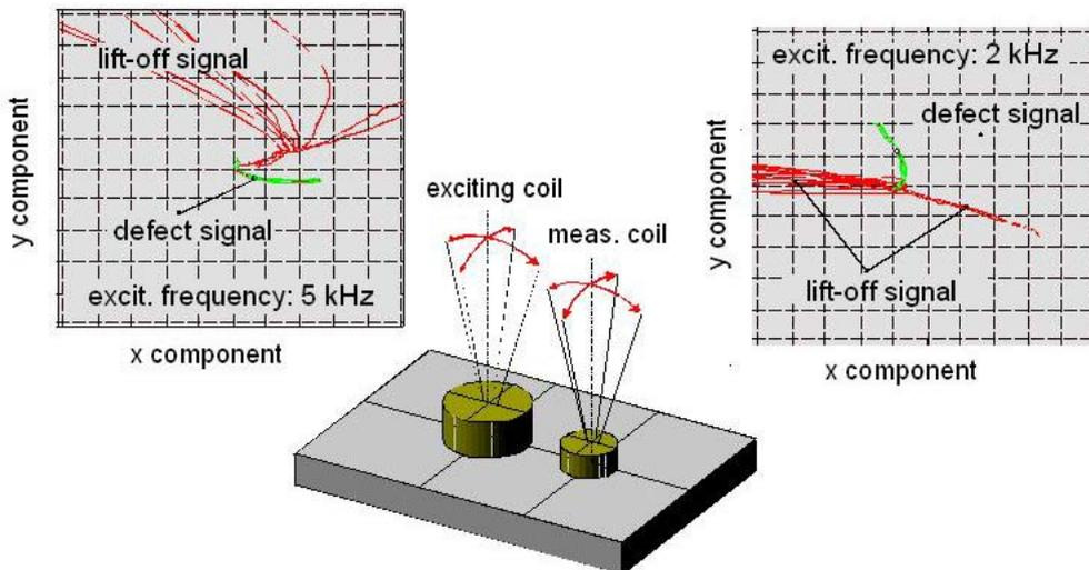
Figure 6: Separation of defect signals and disturbing signals by phase selection
