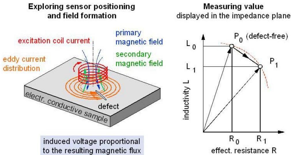
**Figure 2:** Eddy current technique – working principle
