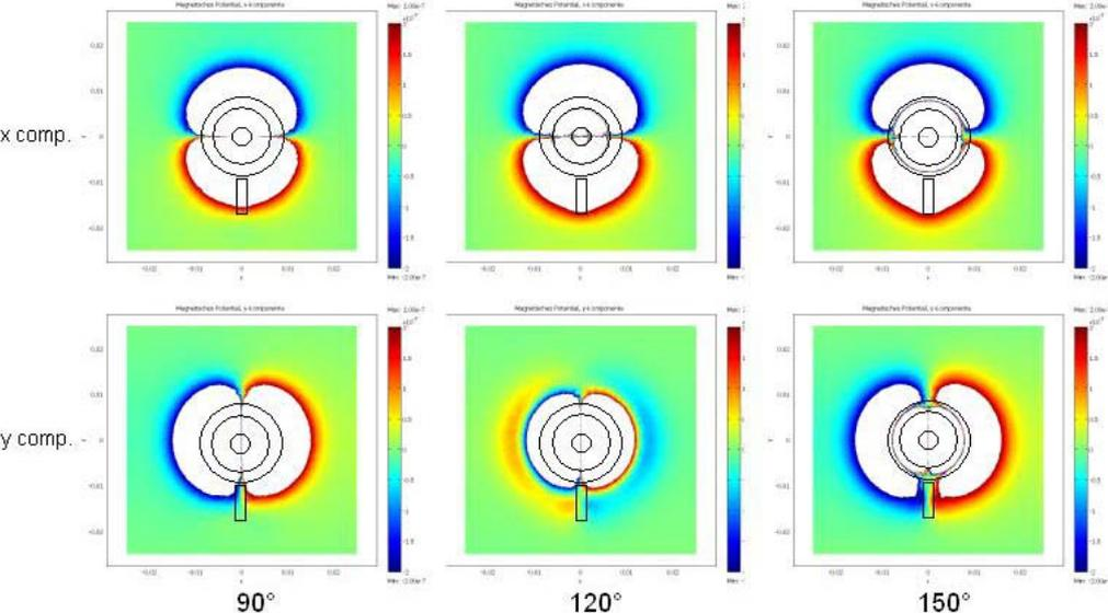
Figure 10: Simulation – magnetic potential II
