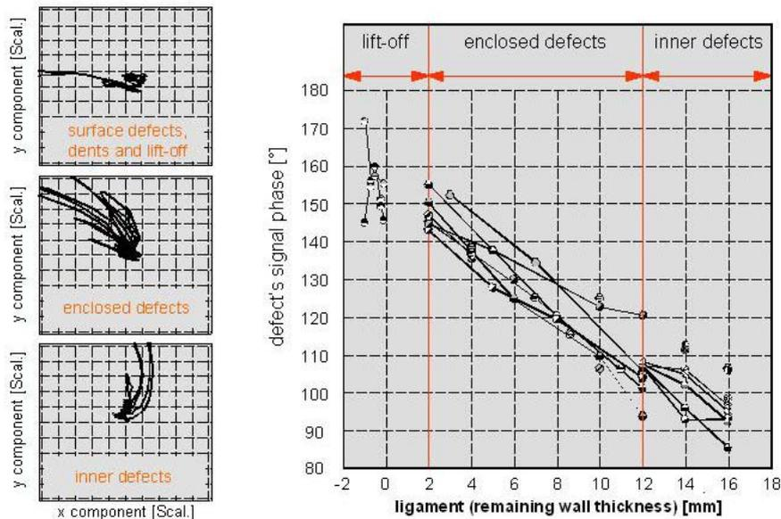
**Figure 12:** Defect depth position – signal phase and ligament
