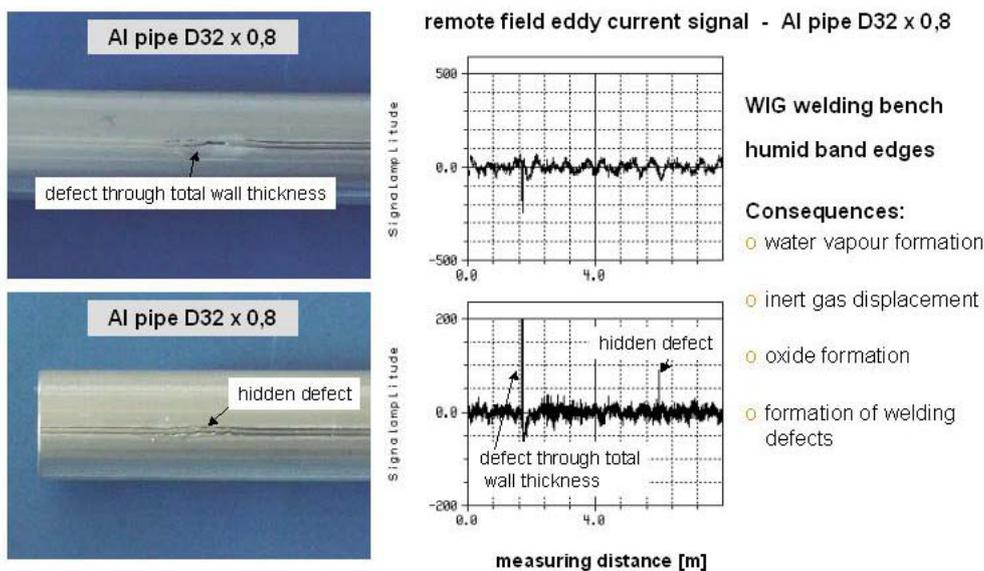
**Figure 15:** Exemplary view and measuring signal of a defect weld seam caused by humid band edges
