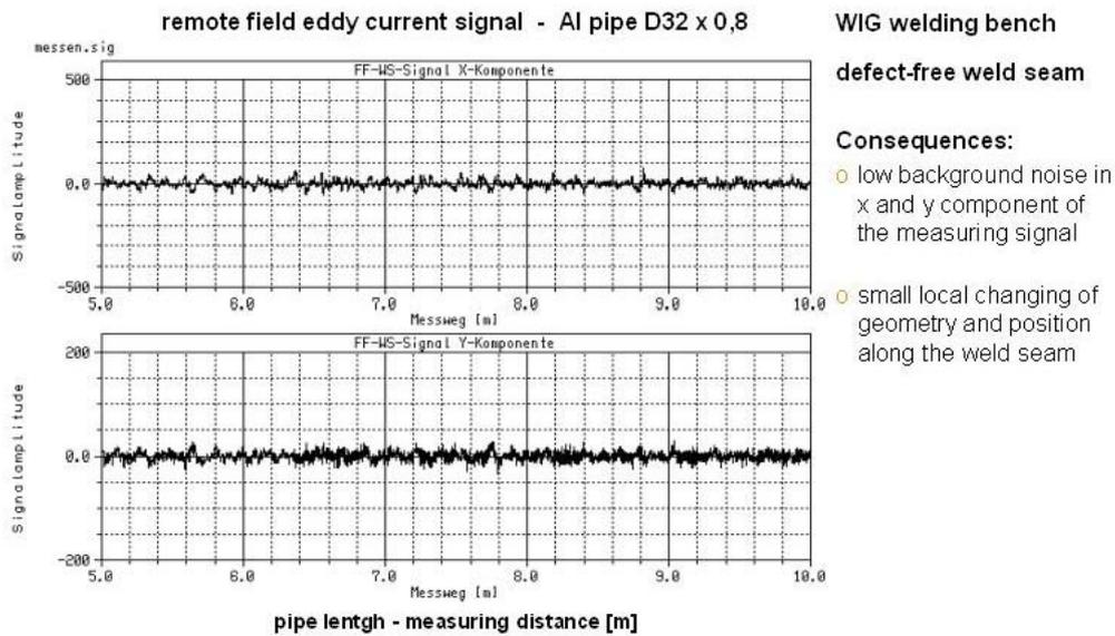
**Figure 14:** Measuring signal of a defect-free weld seam
