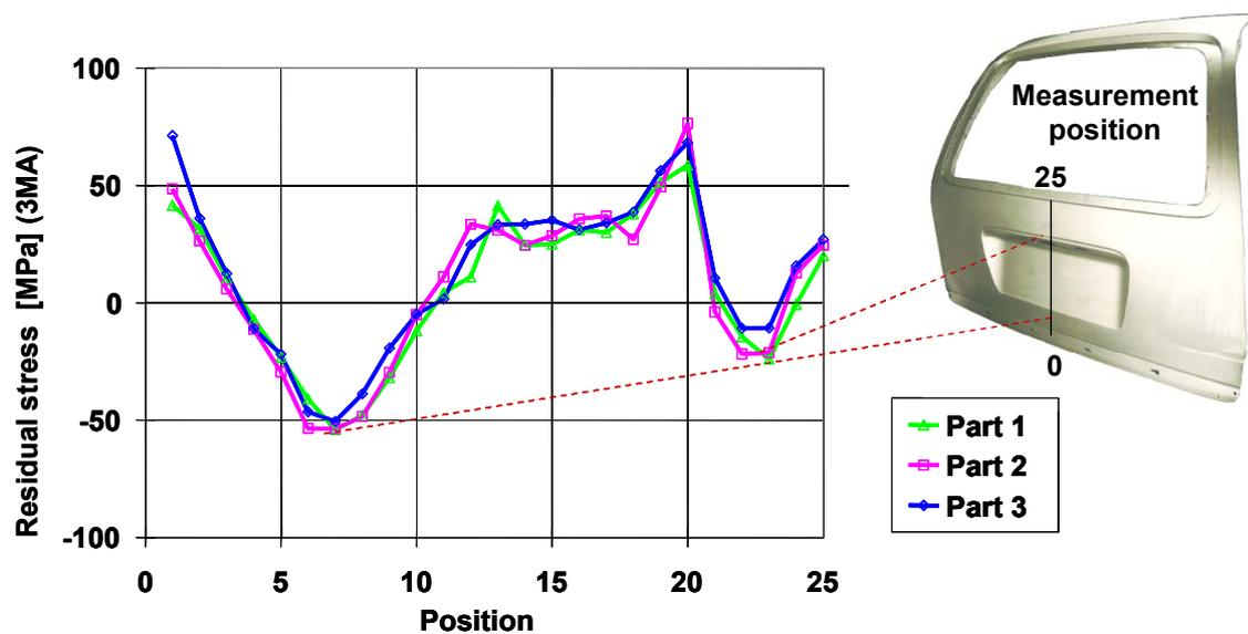
Figure 2. Distribution of residual stress in rear flaps of cars
