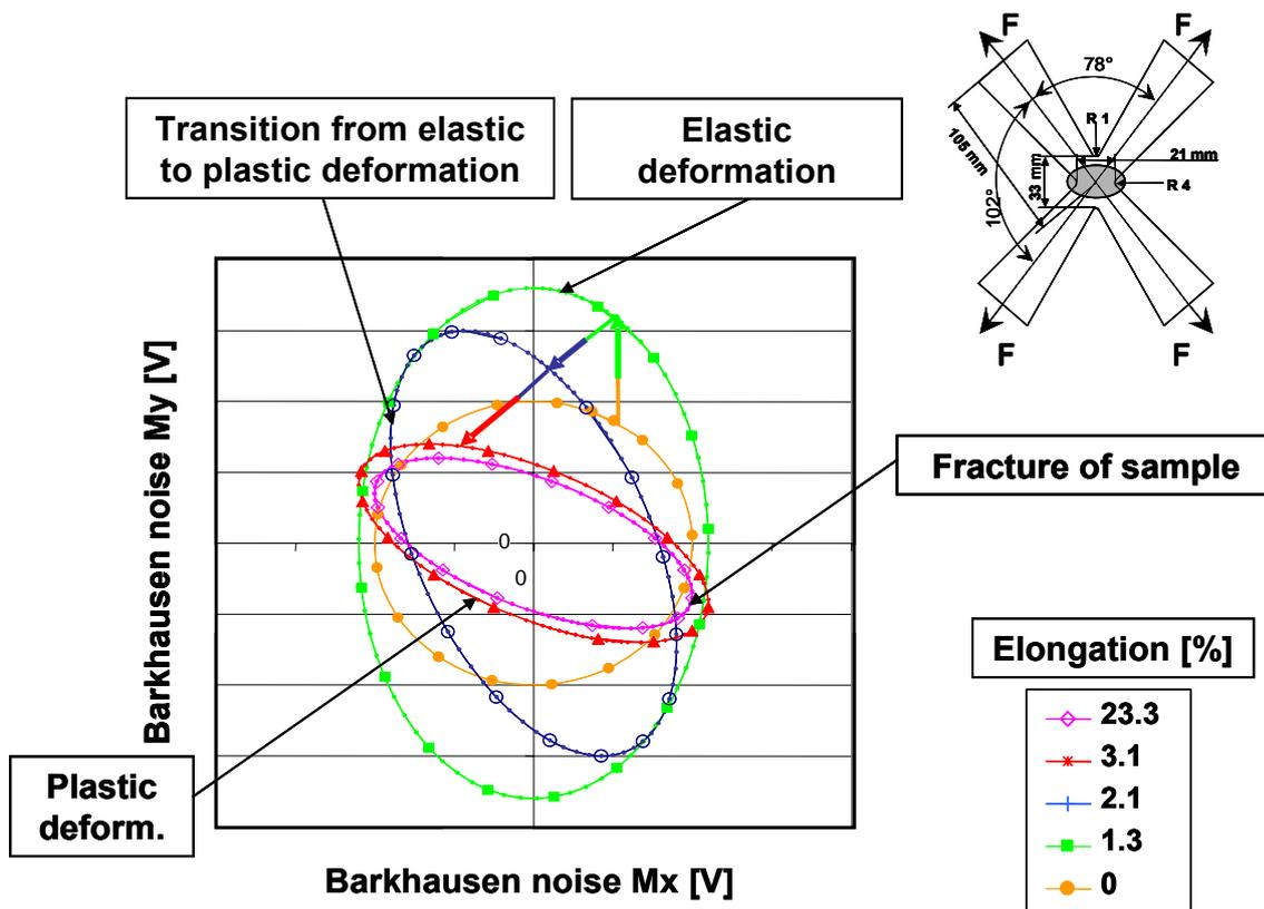
Figure 6. Measurement of pole figures during the cross tensile test on H 320 LA
