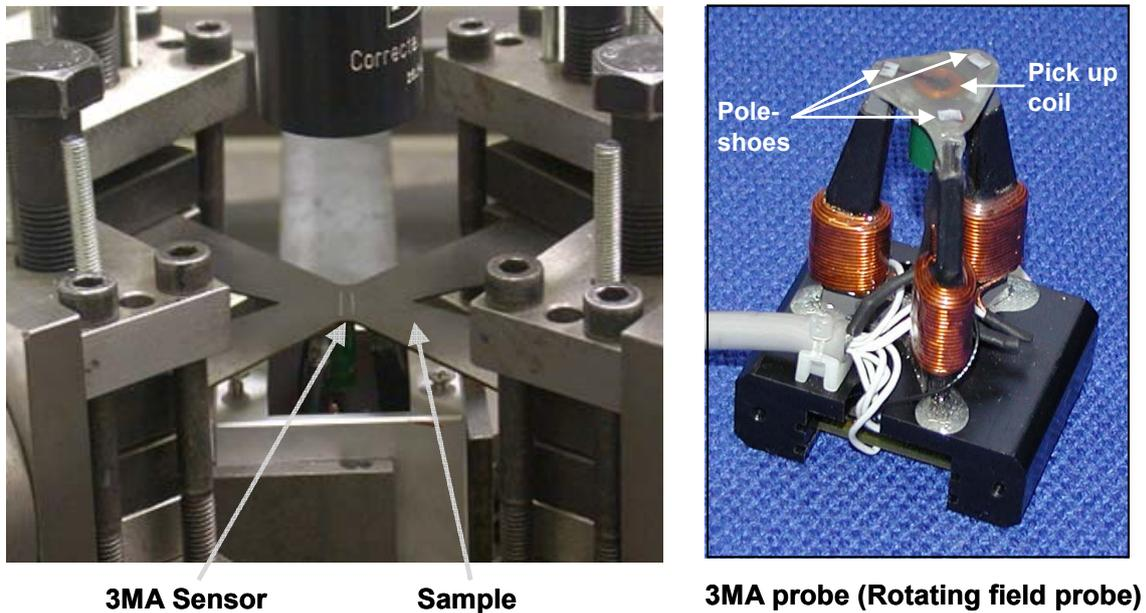
**Figure 5.** Cross tensile test with 3MA rotating field probe and cross tensile sample (left) and special probe using a rotating magnetisation (rotating field probe) (right)
