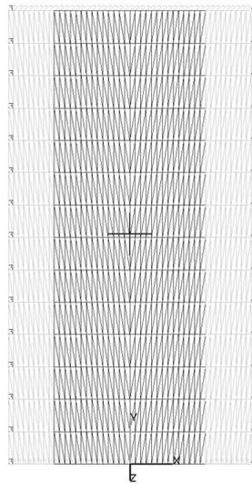
Fig. 3 – Mesh of the 2-2 connectivity piezocomposite (PZT : dark grey, Epoxy : light grey, bounds 3 and 4 coupled via periodicity conditions)
