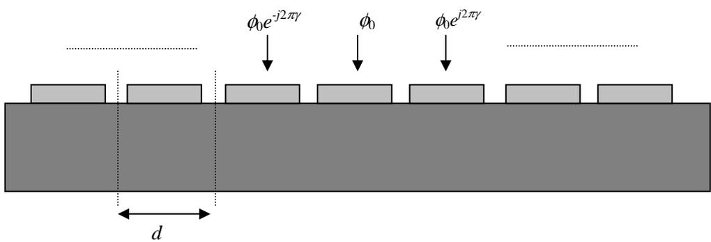
The diagram shows a series of rectangular transducers on a substrate. Three downward arrows represent harmonic excitation at different phases:  $\phi_0 e^{-j2\pi\gamma}$ ,  $\phi_0$ , and  $\phi_0 e^{j2\pi\gamma}$ . A double-headed arrow below the substrate indicates the distance  $d$  between two adjacent transducers.
