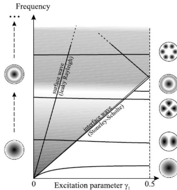
Fig.7 – Definition of the mode of the loaded membrane (the Wilm's diagram [27])
