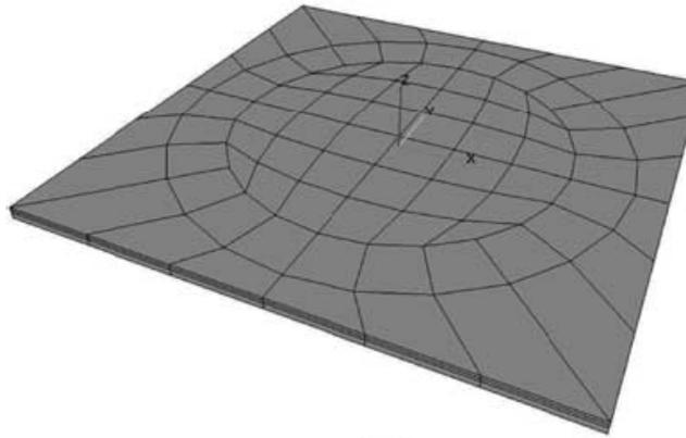
Fig.5 – Mesh implemented for the simulation of bi-periodic cMUT
