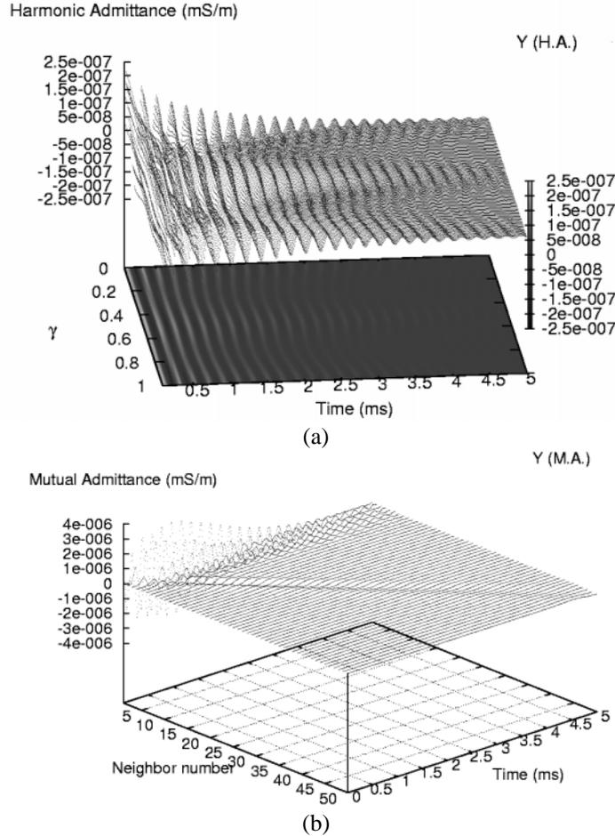
Fig. 4 – Harmonic admittance of the piezocomposite unit cell (a) and related mutual admittances of the 49 first neighbors
