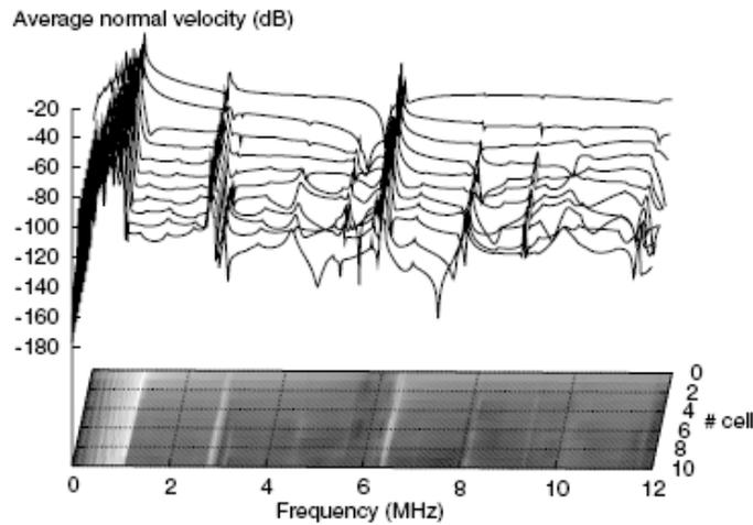
Fig.8 Mutual displacements of cMUTs radiating in water (front side) on semi-infinite silicon (back side)
