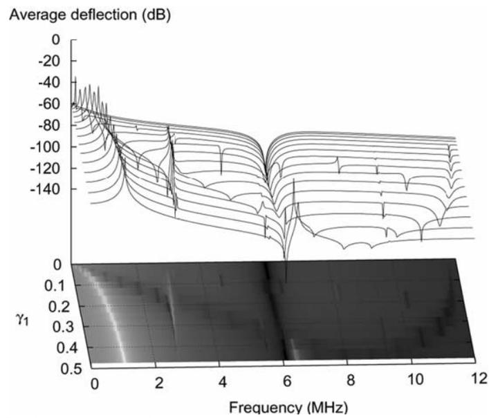
Fig.6 Mean value of the displacement normal to the loaded surface
