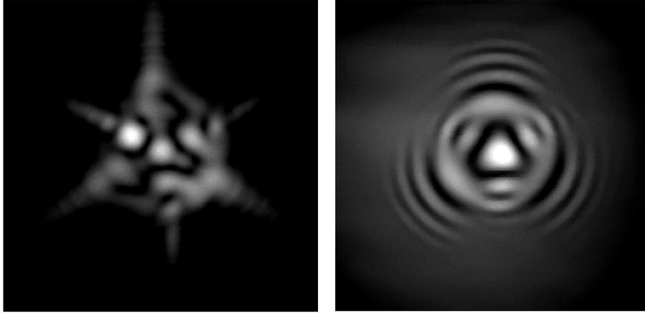
**Fig. 5** Left: magnitude of one of the later transversally polarized echoes (T7 in Fig. 2). Right: magnitude of mode converted waves (L2T1 mode in Fig. 2). The width of the image is 10 mm.
