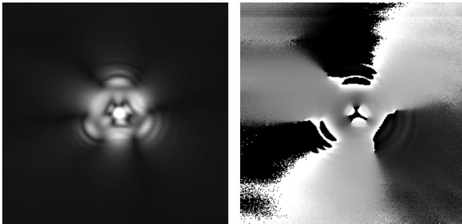
**Fig. 4** Hologram of the first transit signal for transverse polarization (T1 mode in Fig. 2) in  $\text{LiNbO}_3$ . Width of the images: 10 mm; left: representation of the magnitude with brightness proportional to the magnitude; right: representation of the phase with full gray scale proportional to  $2\pi$ .
