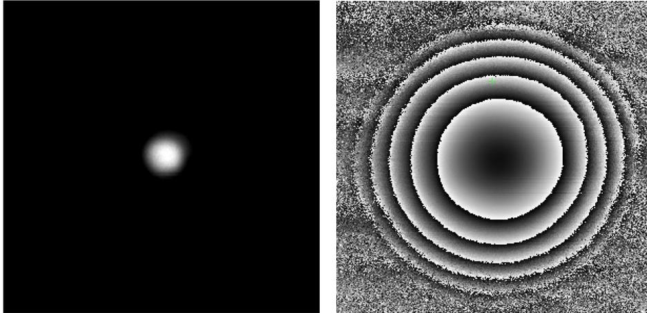
**Fig. 3** Hologram of the first transit signal for longitudinal polarization (L1 mode in Fig. 2) in  $\text{LiNbO}_3$ . Width of the images: 10 mm; left: representation of the magnitude with brightness proportional to the magnitude; right: representation of the phase with full gray scale proportional to  $2\pi$ .
