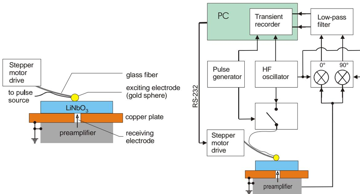
**Fig. 1** Experimental setup: sample mount (left) and electronic scheme (right).
