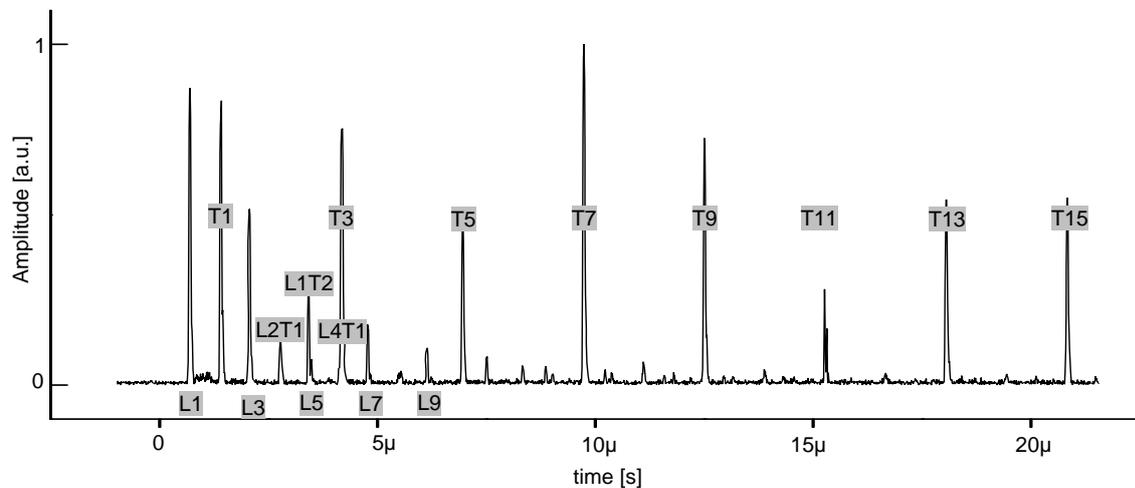
**Fig. 2** Amplitude waveform acquired at the center of the scan area. Duration of the excitation burst was 53 ns. Labels denote transverse (T), longitudinal (L), or mode-converted waves (LT). The number correspond states how often the crystal was traversed by particular mode. Some of the modes interfere due to arrival at nearly the same time (L5 and L1T2, T3 and L4T1).
