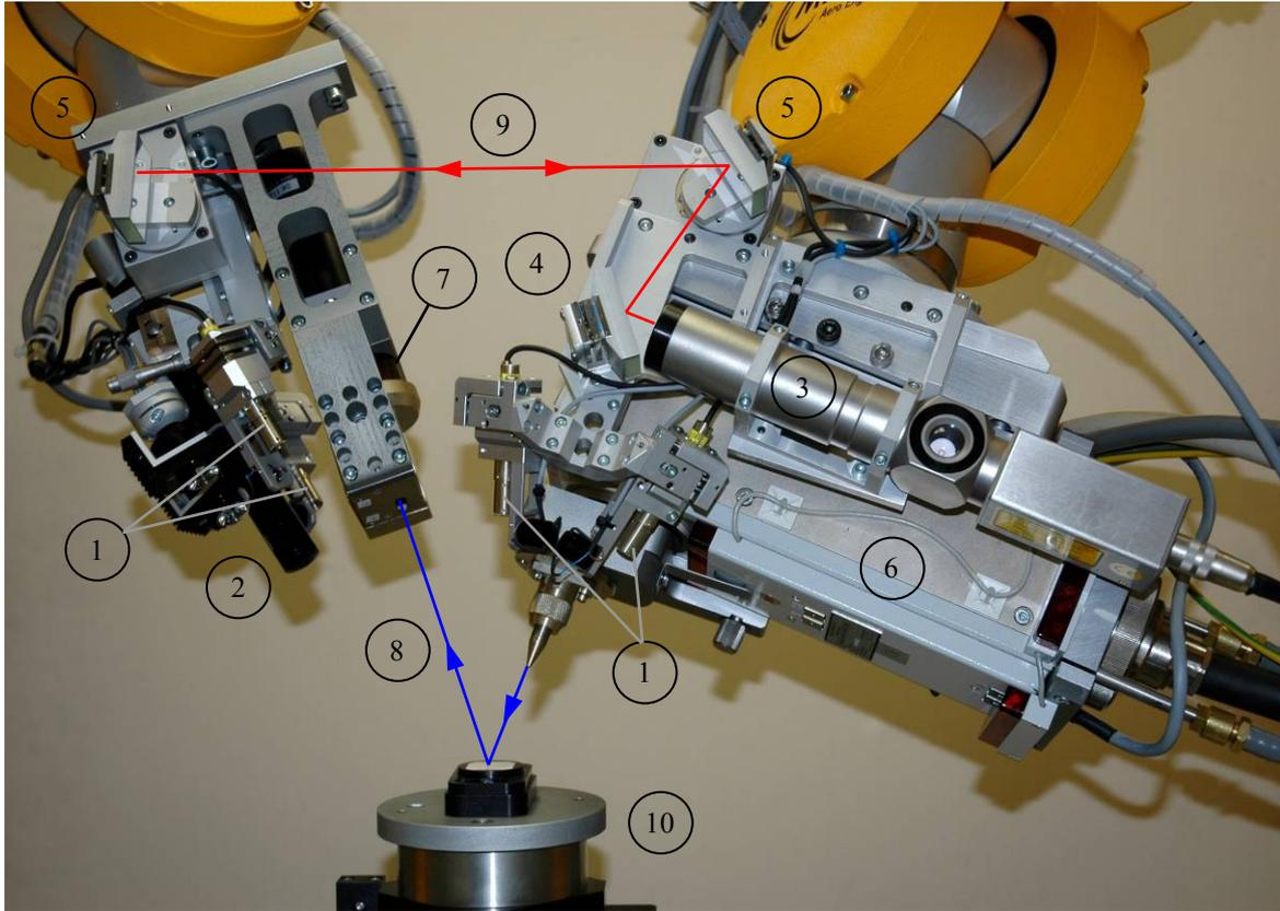
Fig. 3: Detailed view of the optical measuring system to synchronize the two robots. 1= laser line projectors, 2 = camera system, 3 = autocollimation telescope, 4 = fixed deflector mirror, 5 = movable deflector mirror, 6 = X-ray source, 7 = X-ray detector, 8 = X-ray beam, 9 = laser beam, 10 = audit column.
