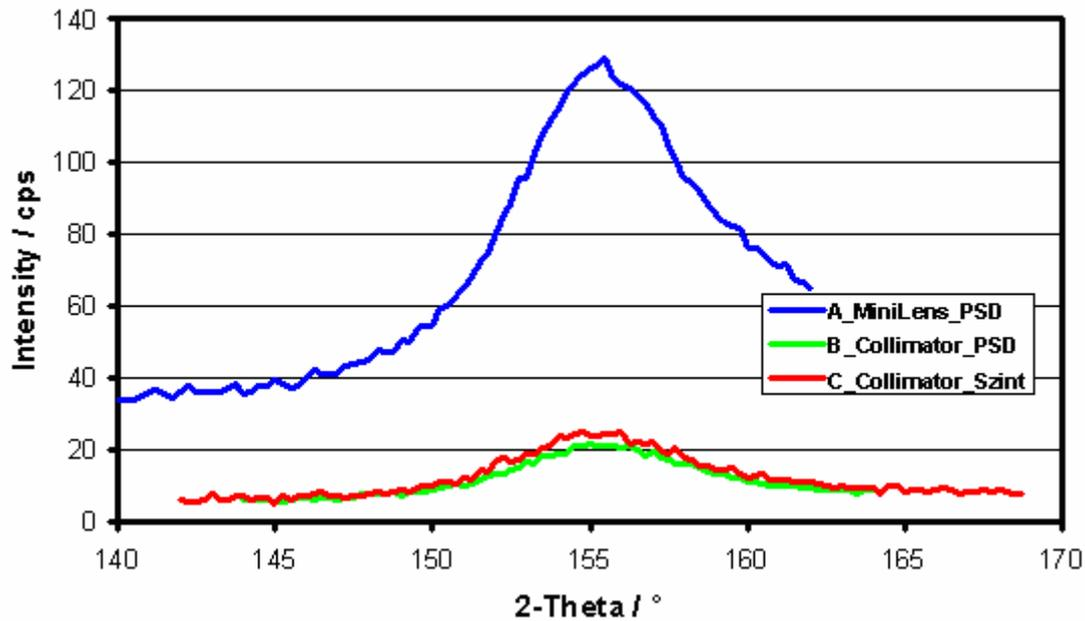
Fig. 8: X-ray diffraction measurements on 100 Cr 6 reference sample (B524) with CrK $\alpha$  radiation. Comparison of scans using 1 mm minilens primary optic (A) against 1 mm collimator (B) and of peak profiles from scintillation (C) and PSD (B) detector with collimator.
