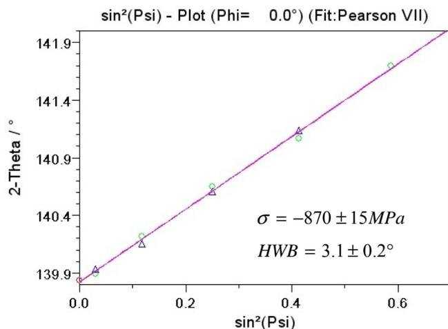
Fig. 6: Residual stress measurements on a compressor blisk in the Charon XRD diffractometer (left) and a typical  $2\theta$ - $\sin^2\psi$  diagram with the determined results (right) at a measuring position near the blade edge in the blade root region.
