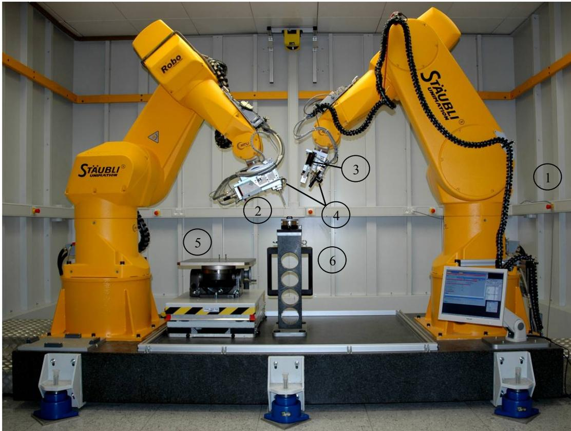
Fig. 2: Interior view of the Charon XRD X-ray robot diffractometer. 1 = radiation protection cabin, 2 = X-ray source, 3 = X-ray detector, 4 = optical measuring system, 5 = component positioning unit, 6 = audit column.
