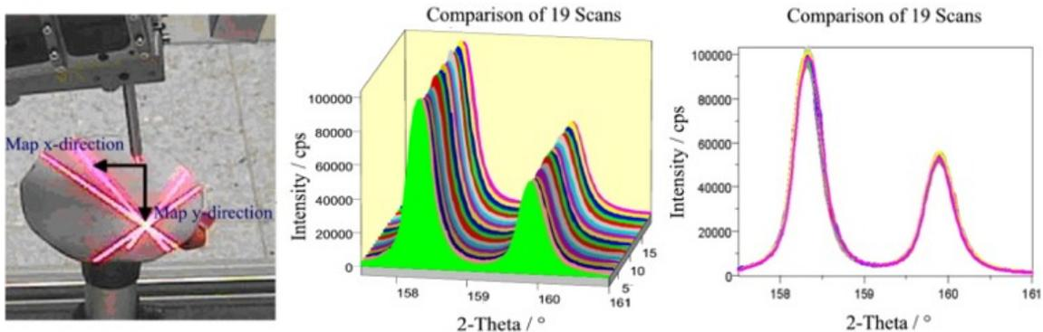
Fig. 5: Setup (left) and intensity profiles in 3D (mid) and 2D (right) of scans in x- and y-directions on tilted single-crystal silicon disk.
