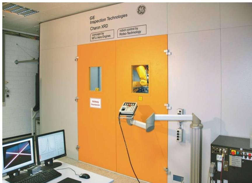
Fig. 1: Outside view of the Charon XRD X-ray robot diffractometer.
