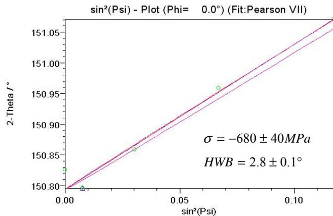
Fig. 7: Residual stress measurements on a stator of a compressor in the Charon XRD diffractometer (left) and a typical  $2\theta$ - $\sin^2\psi$  diagram with the determined results (right) at a measuring position near the airfoil edge.
