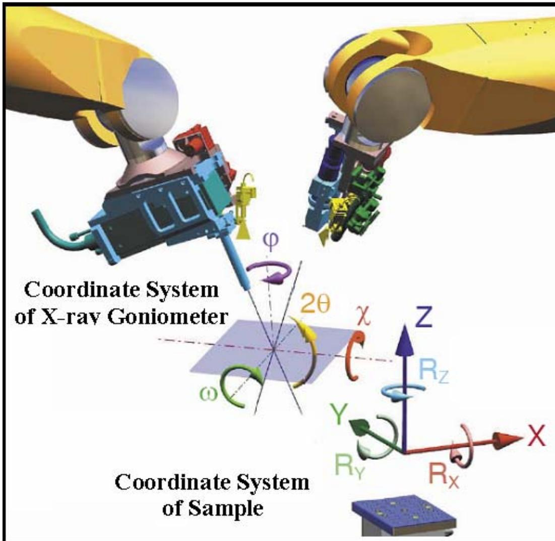
Fig. 4: Schematically view of X-ray goniometer and sample coordinate systems.
